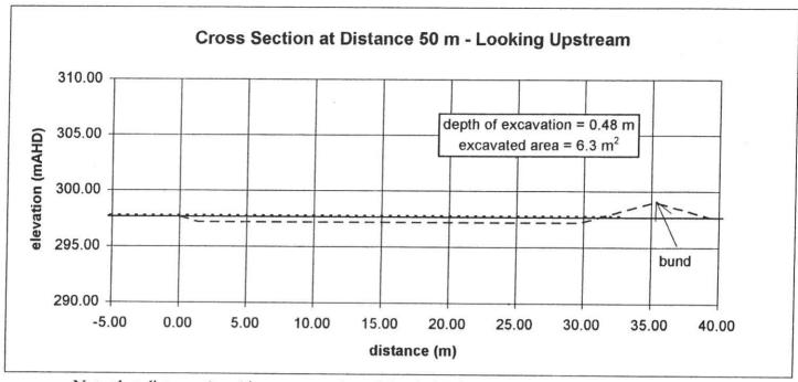
Note that distance 0 m (the western edge of the drain) is to be 40 m NNW of the survey location to provide a more gradual bend radius (see Fig. 13)
