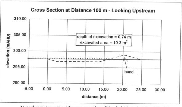
Note that distance 0 m (the western edge of the drain) is to be 20 m SE of the survey location to provide a more gradual bend radius (see Fig. 13)
