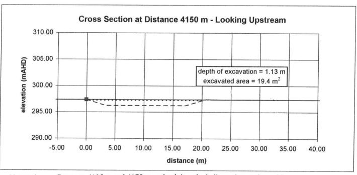
Between 4125 m and 4175 m no bank is to be built on the southern side Notes: 1. to allow natural overflow to flow into the drain.
