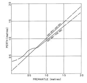
Figure 13. Comparison of the tidal influence between Perth and Fremantle for the years 1961-62 and 1973-74. *Courtesy – P.W.D. (Harbour and Rivers)*
