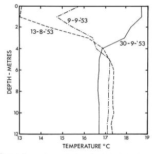
Figure 8. Temperature — depth profiles in the basin of the Swan River Estuary (off Applecross) during the recovery period, 1953. *After Spencer (1956).*
