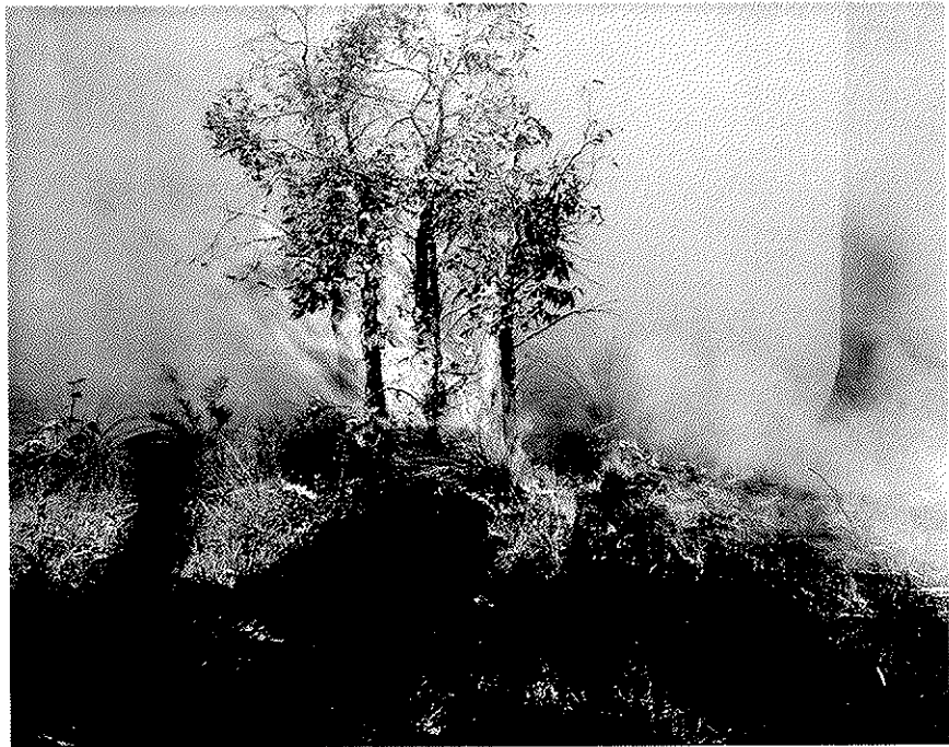
(8). Fire No. 10 at 1516 hrs. ( 46 minutes from the start) Flame height 8-10' in lighter type of fuel. 9-4-59.
