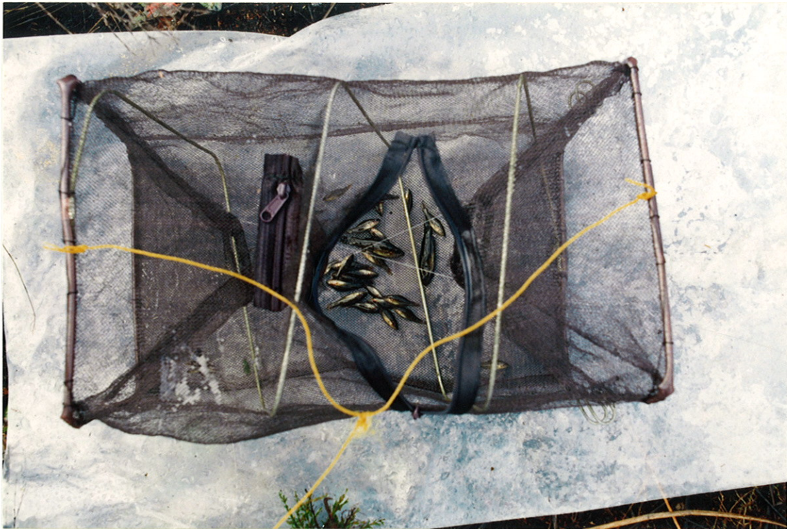
Figure 2. Overhead view of baited fish trap. Note the two funnel entrances, pouch for bait (short zip) and long zip (open) for retrieval of fish. Trap length is 40 cm.
