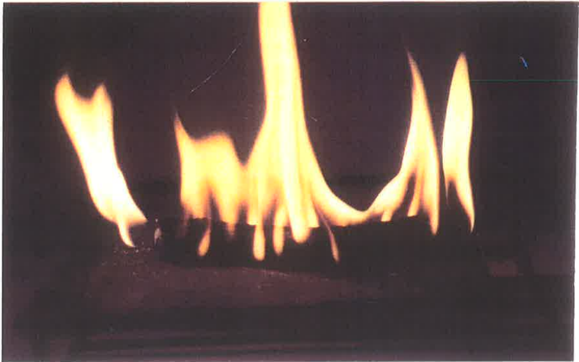
Plate 6-1: A round wood piece burning on a gauze platform. Round twigs <6 mm diameter and leaves are the most flammable component of the jarrah forest fuel complex.
