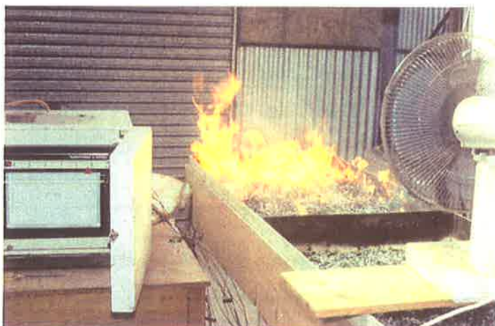
Plate 12-2: Fire-induced soil heating was examined in the laboratory using thermocouples and jarrah forest litter fuel as the heat source.
