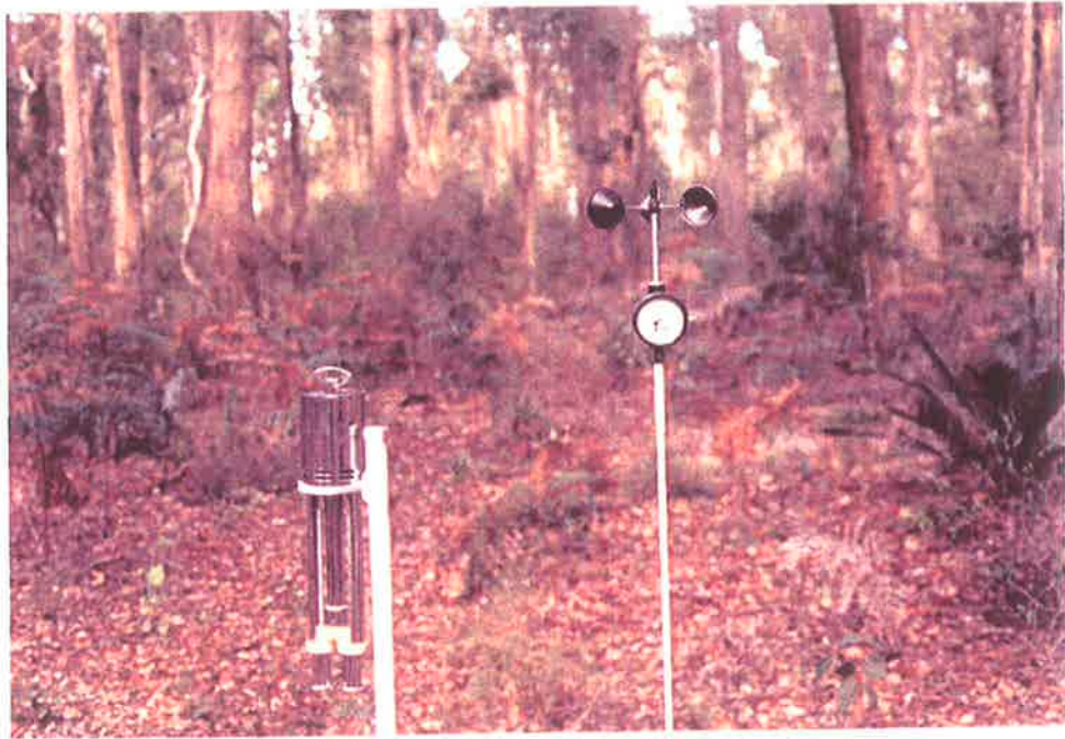
Plate 8-5: A mechanical weather station consisting of a sensitive cup anemometer at 10 m (not shown), an anemometer at 1.5 m and an aspirated psychrometer.
