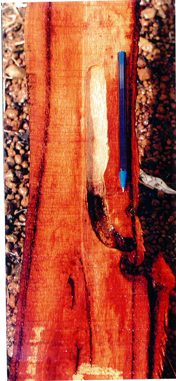
Sawn regrowth slab showing pupation chamber of Tryphocaria and associated gum damage.
