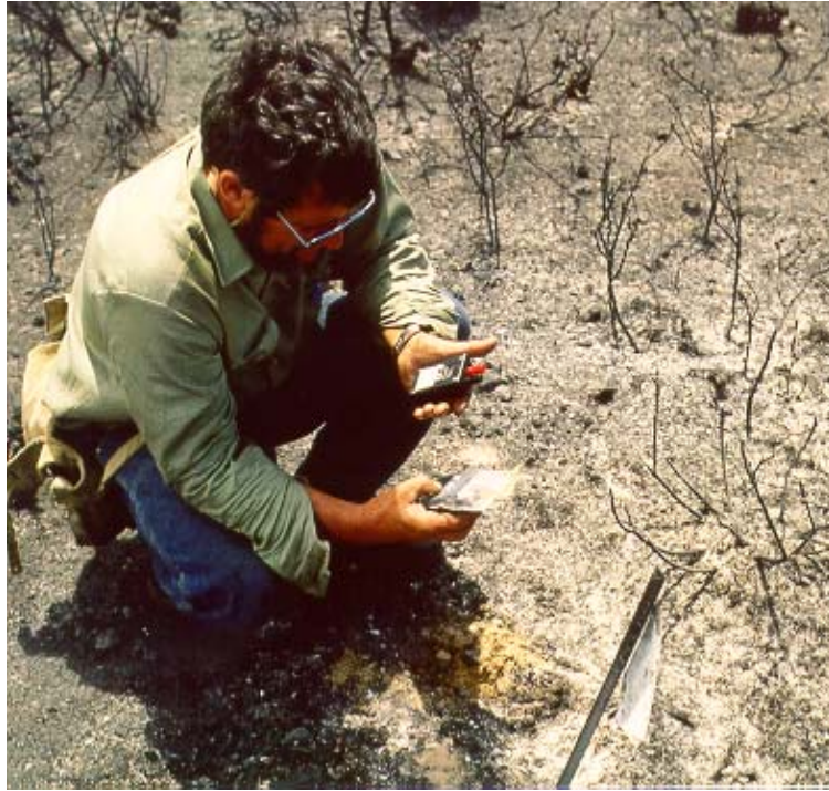
Plate 7 An electronic fire spread timer being collected at the completion of an experimental fire and compared with a master clock to determine the time at which the fire reached an established grid point.
