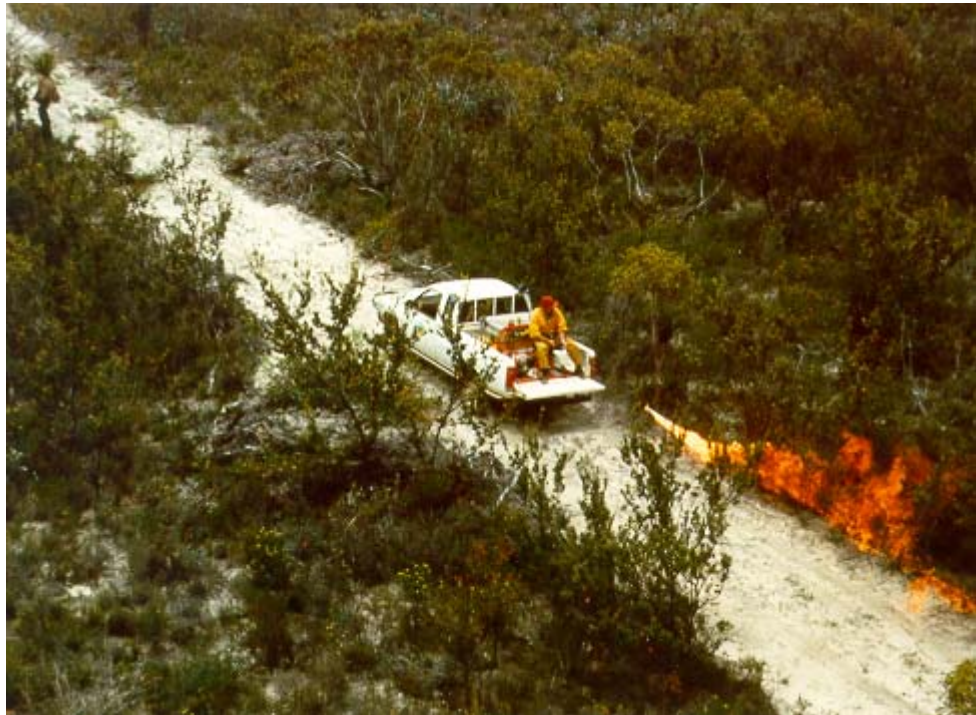
Plate 8 Ignition of experimental fire in Plot E using a vehicle-mounted flamethrower.
