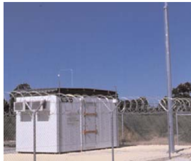
Figure 4. A typical Air Quality Monitoring Station.
