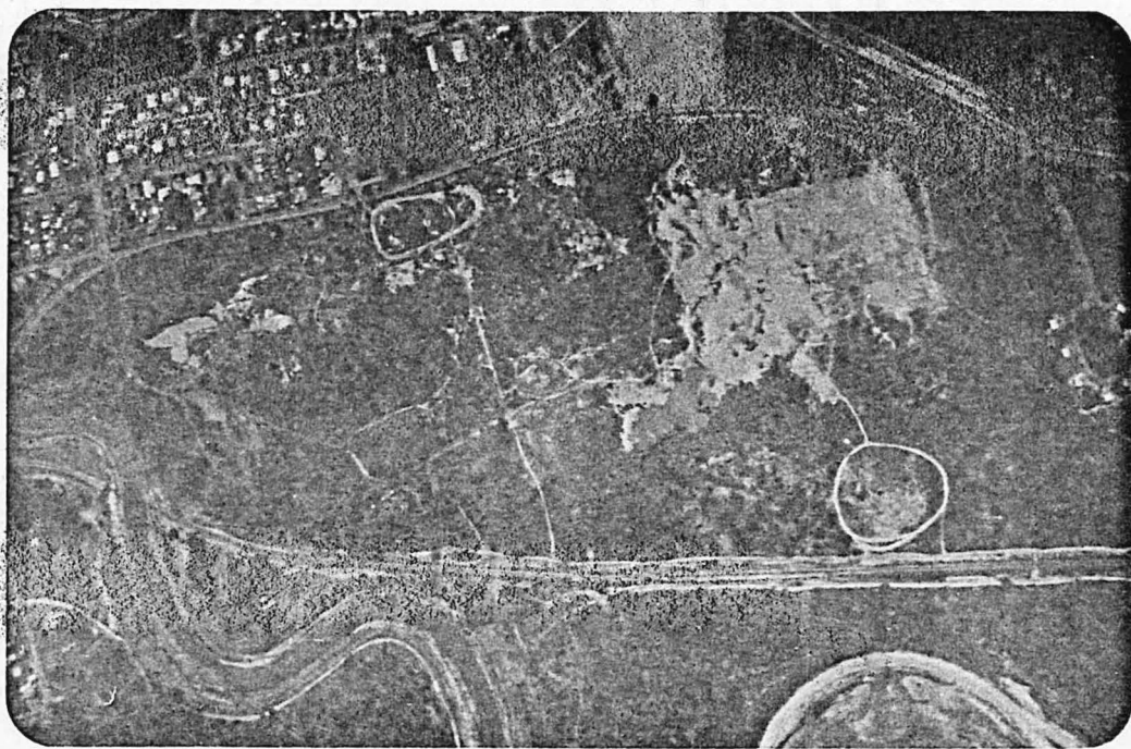
Wallsend open cut between Coalfields Road and Collie River. Just north of Railway line to Darkan. Water area in open cut left centre. Moderate to good regeneration in the open cut and adjoining dumps. Most of the white area right centre in Collie rubbish dump. Photographed by I. Jacobs 3/8/82.
