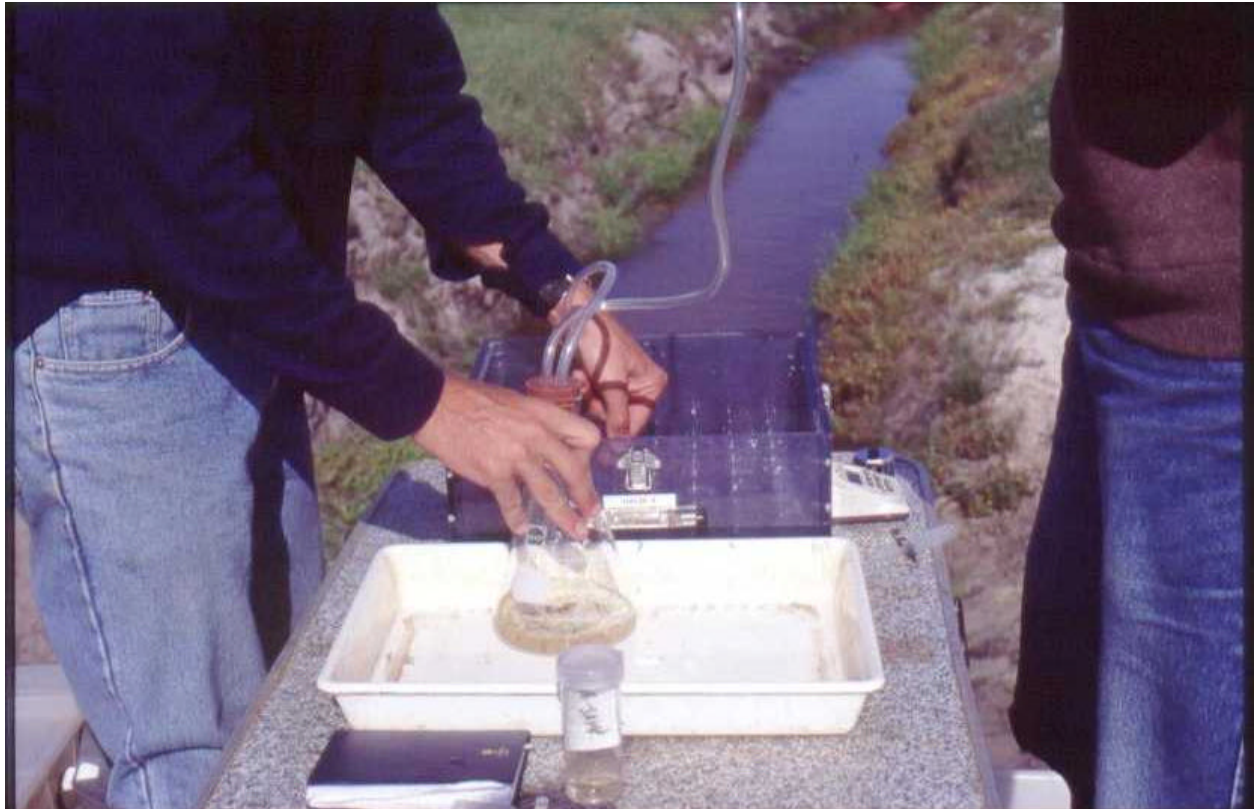
Figure 1. Box subsampler. Sample is being sucked out of a randomly selected cell into conical flask using vacuum created with hand pump (out of sight)
