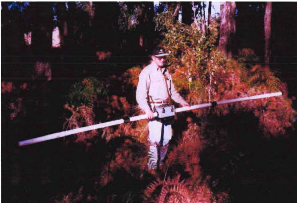
Fig. 1. Geonics EM31 ground conductivity meter shown in vertical dipole mode at 0.8m height.
