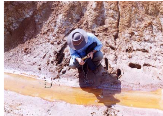
Sampling salt concentration of drain water
