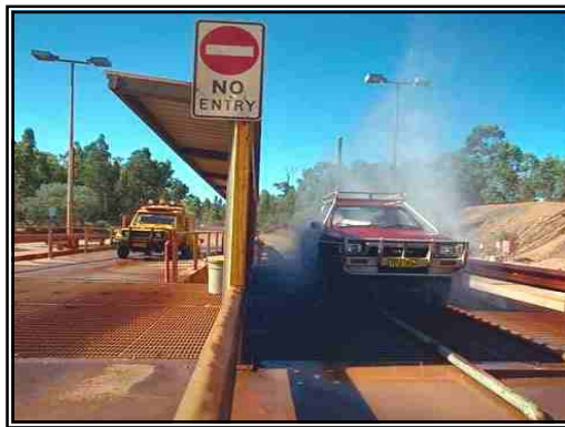
Figure 7.5 Vehicles are cleaned before entering uninfested areas
