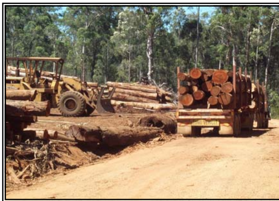
Figure 7.8 A simple front log barrier helps prevent cross contamination from the road to the uninfested forest
