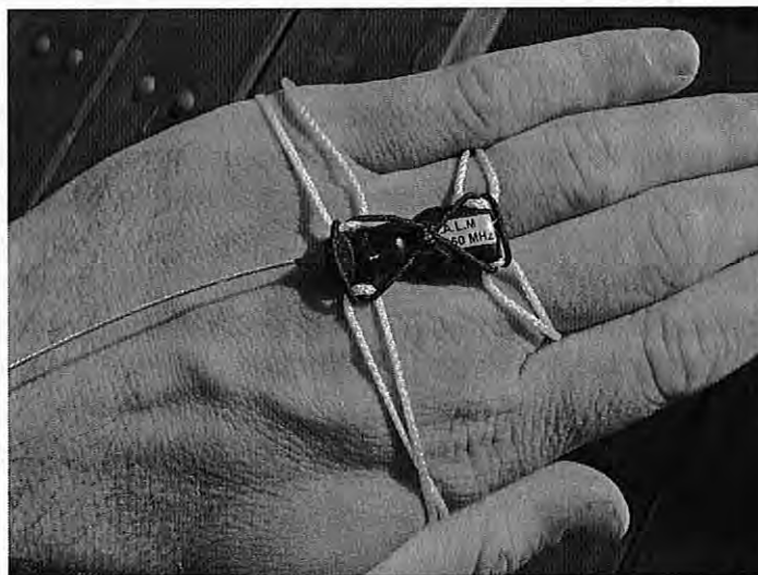
Figure 8 Transmitter with modified harness
