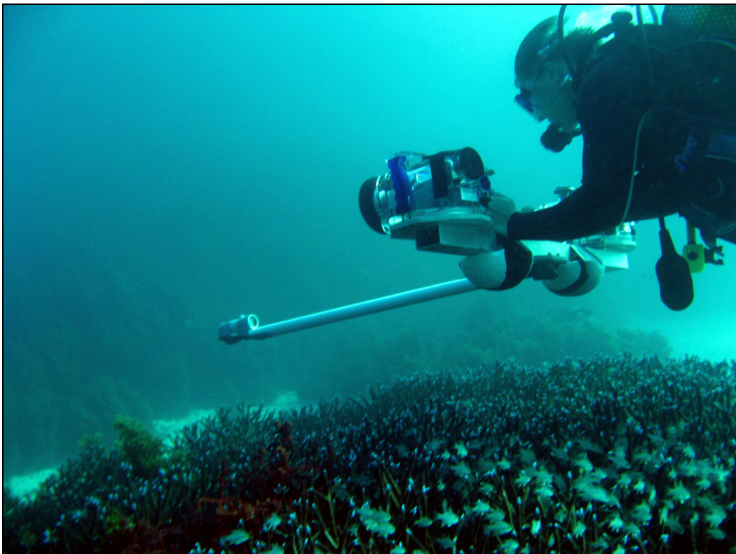
Figure 4. Photo showing the stereo-video UVC equipment being used in a Western Australia tropical reef environment (Abrolhos Islands 2007). Source: Dianne Watson, UWA.
