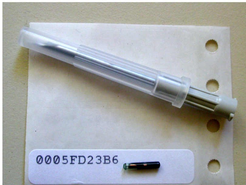
Figure 9: Trovan® passive implant transponder (PIT) and applicator needle used to individually mark mammals and adult varanids trapped at Leschenault Peninsula Conservation Park and Yalgorup National Park. The number is the unique code of the PIT.
