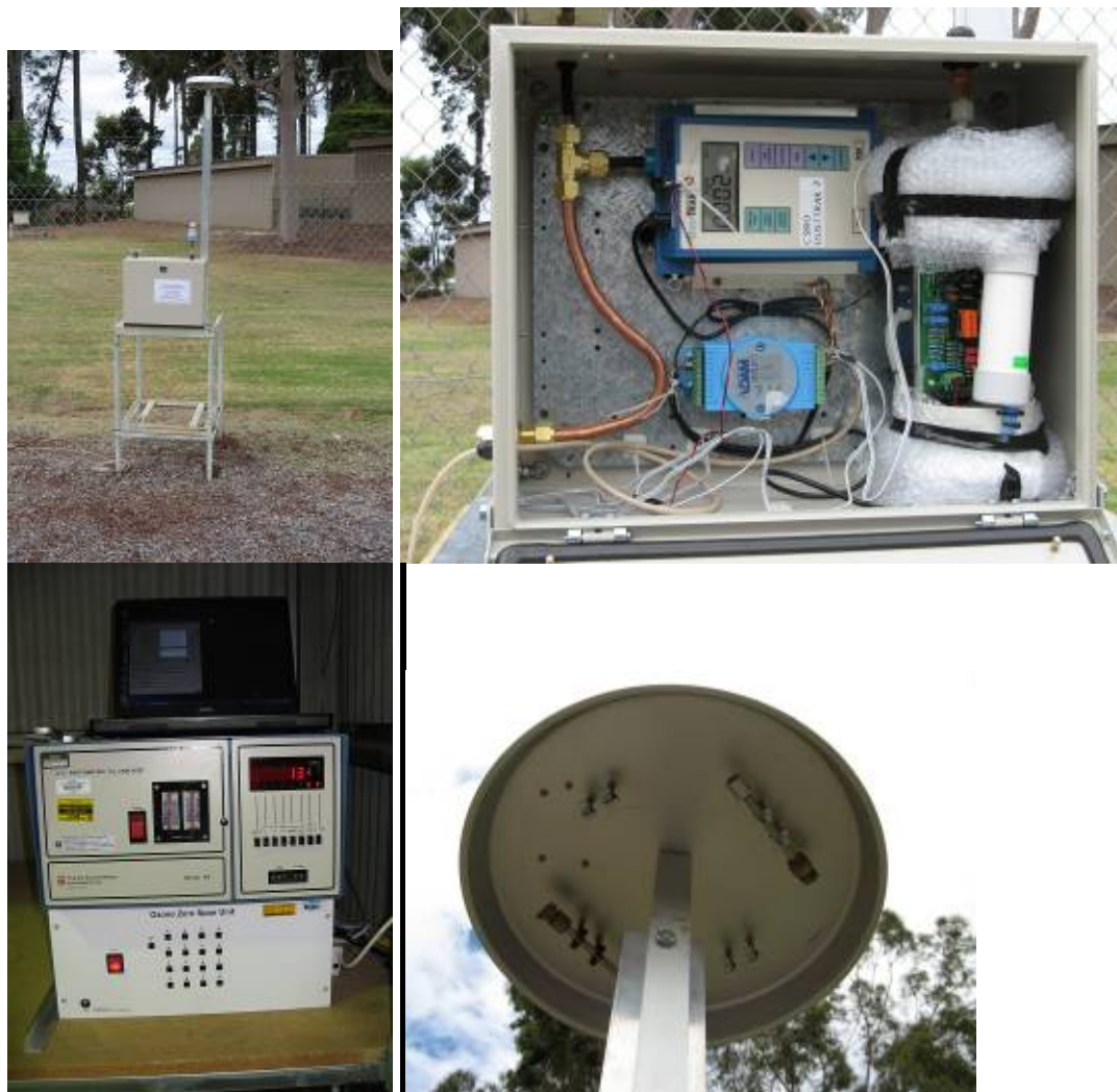
Figure 5-11 Instrument set-up at Manjimup, WA: (a) location of sampling station, (b) sampling box, (c) ozone analyser and (d) BTEX sampling set-up
