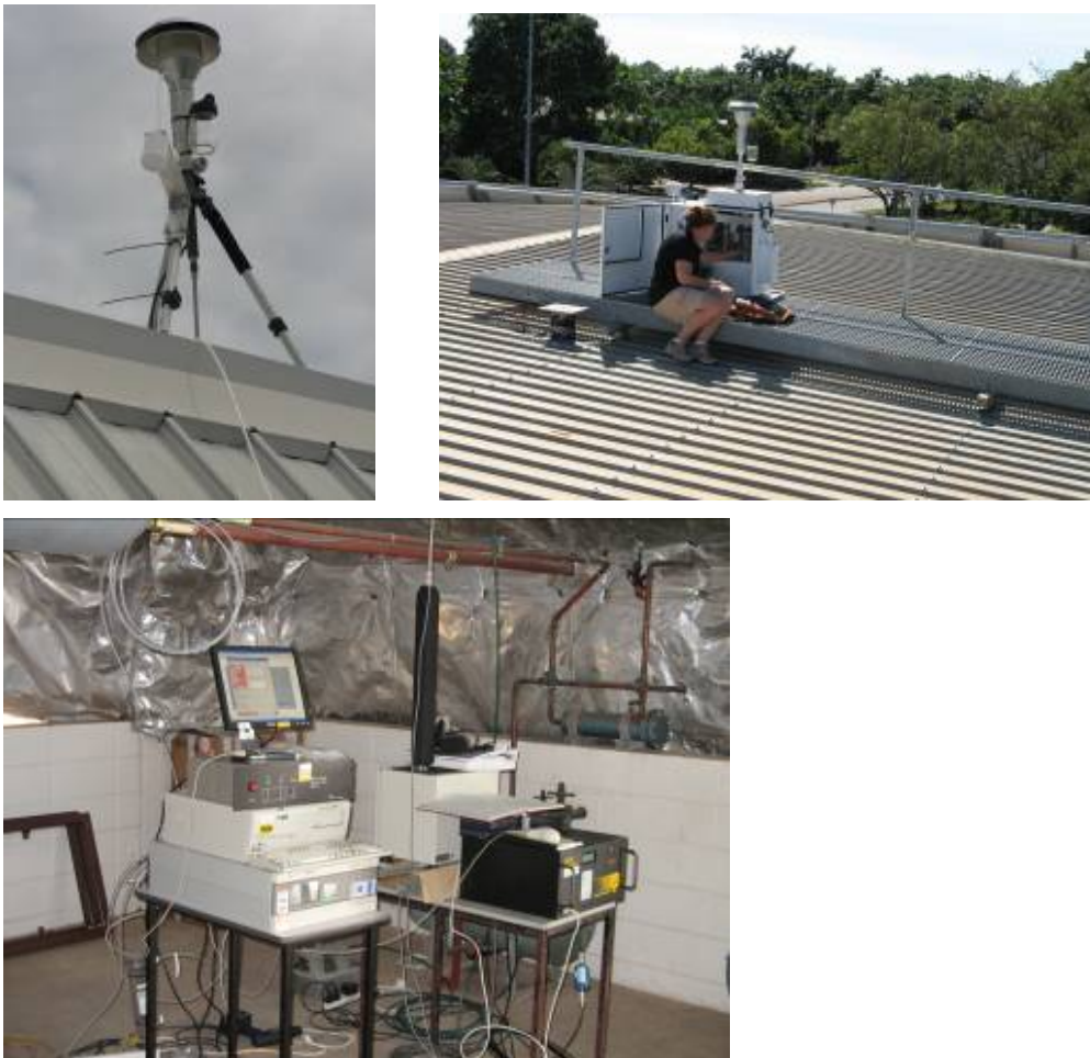
Figure 5-2: Instrumentation set-up at Casuarina, Darwin NT: (a) inlet, (b) partisol sampler and (c) ozone analyser and TEOM
