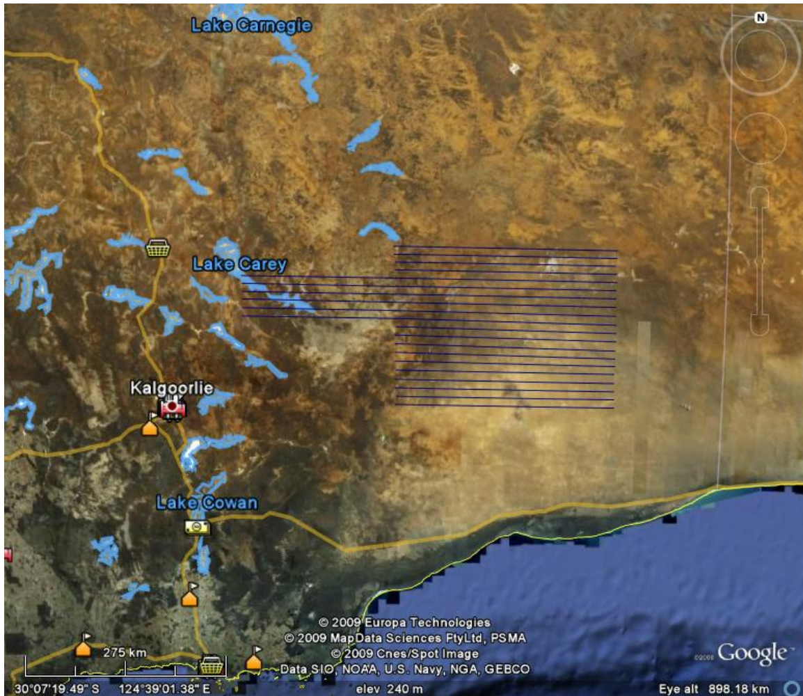
Figure 1: Survey flight lines showing main survey area with additional 6 lines extended to the west across Lake Carey.
