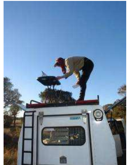
Photo 27: Telemetric download of water level logger data to laptop. Alan Clarke, Lake Pleasant View, 10Aug2010.
