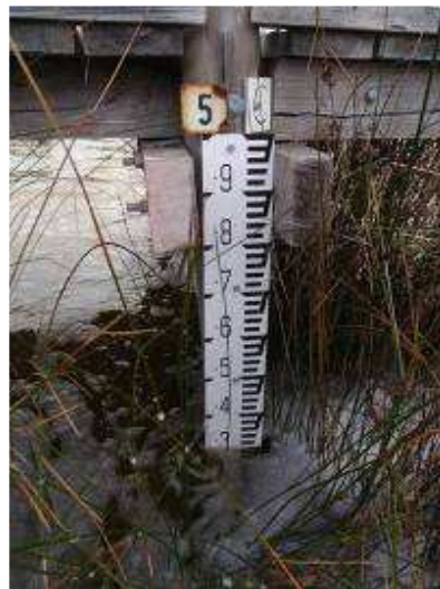
Photo 5: DEC depth gauge 'C' at Lake Clifton on 13Sep2008 read 4.30m.
