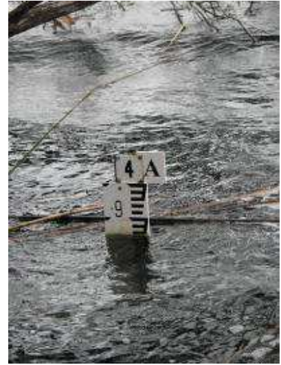
Photo 3: DEC depth gauge 'A' at Lake Wilson on 03Nov2008 read 3.85m.
