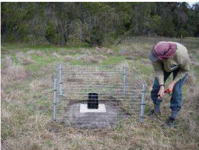
Photo 28: Tipping bucket rainfall recorders have been installed on twelve wetlands. Alan Clarke, 17Jun2009.
