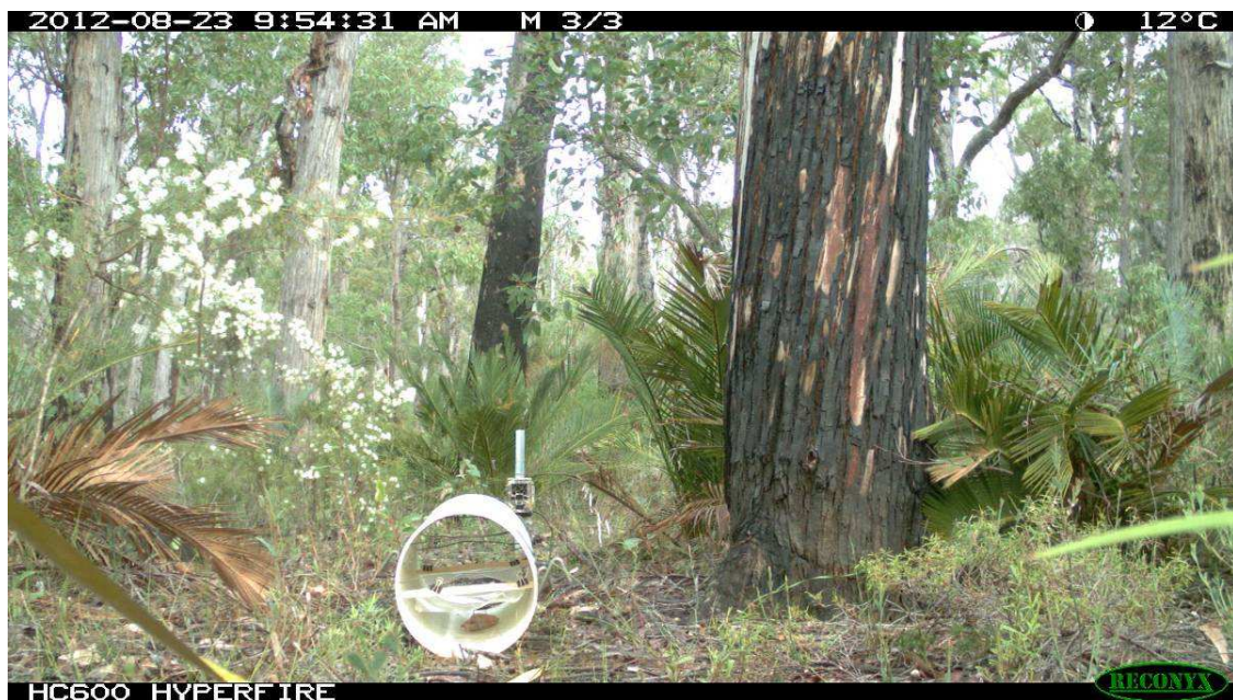
Figure 17. Example of the 'Garretson pipe' setup during the preliminary pilot trial showing the hair trap baited with a chicken wing and a remote sensor camera in the background to monitor approaches by fauna.
