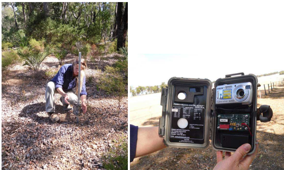
Figure 77. a) Setting up a remote sensor camera in the field to monitor introduced predators and native fauna, b) Pixcontroller Digital Eye remote sensor camera.
