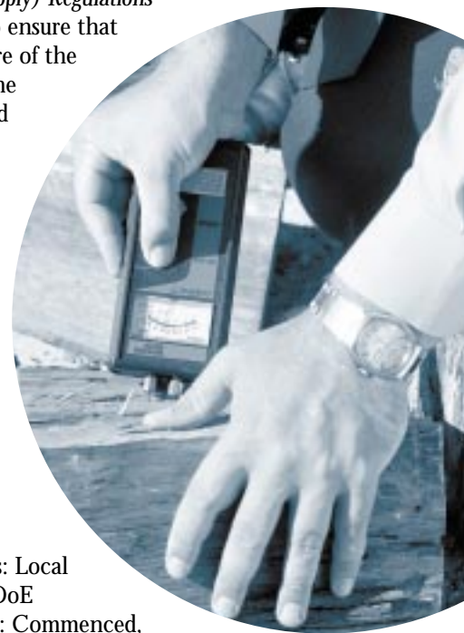
Testing of domestic fire wood for moisture content.
