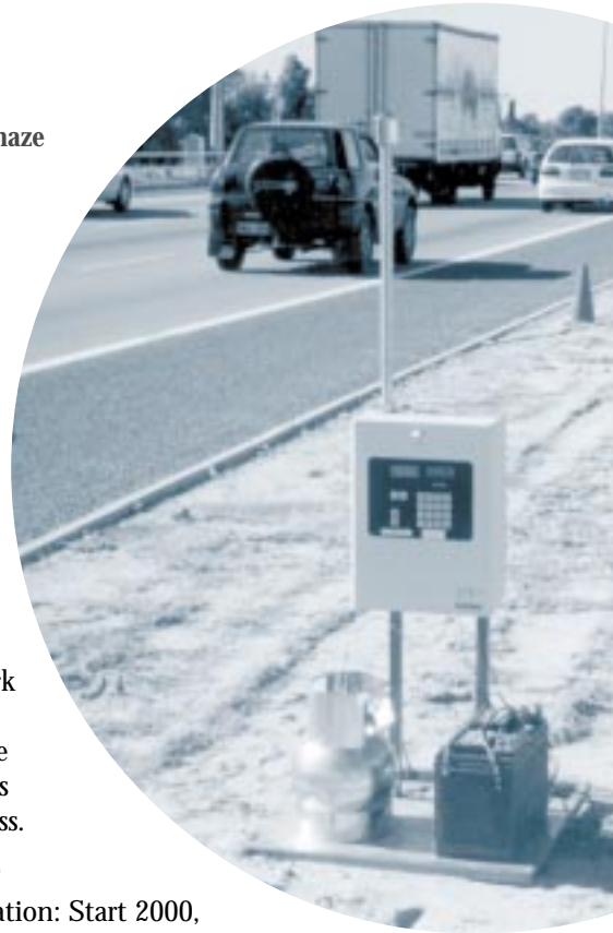
Roadside monitoring of volatile organic compounds (VOCs) discharged in the exhaust emissions of motor vehicles travelling along the Mitchell Freeway.
