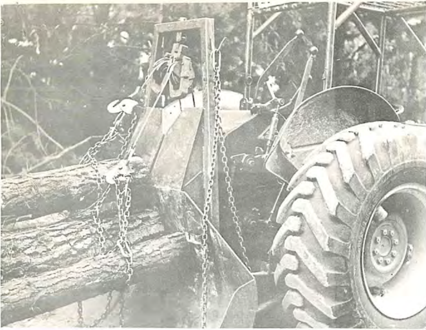
FIGURE 3. A Nell double drum winch fitted to a standard M.F. 35.
