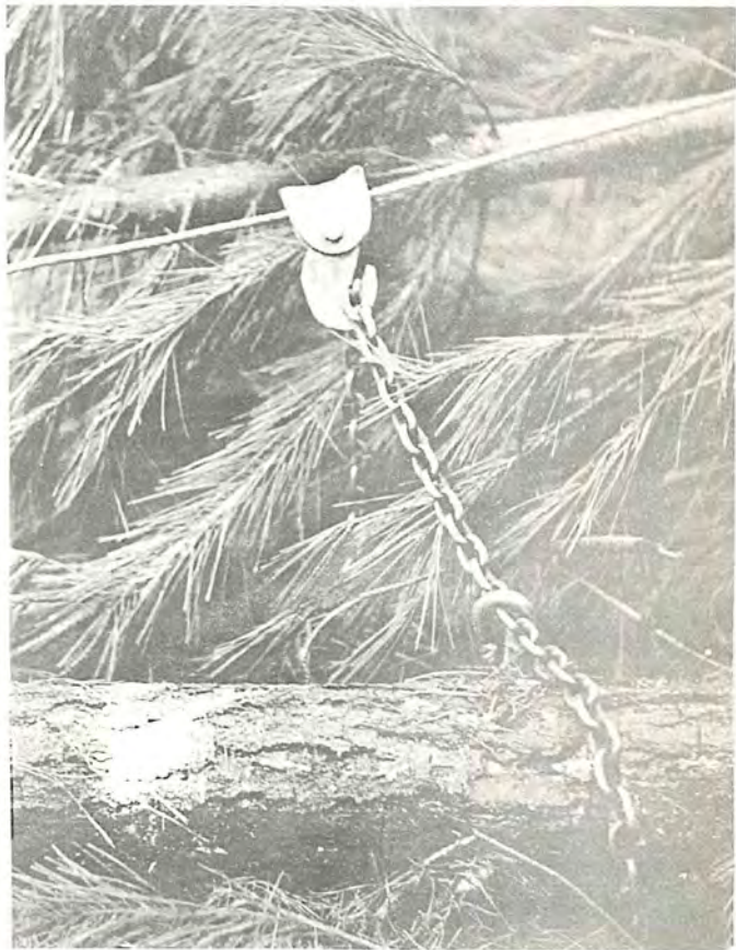
FIGURE 4. Sliding hook and chain choker as used for tree length extraction.
