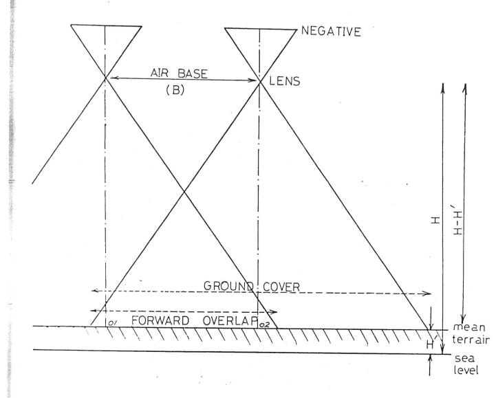
In Figure 4.3 the horizontal or flat terrain lies in a plane above the datum which is mean sea level. The distance between the two planes is denoted by H' and may be referred to as the mean terrain height. The aircraft is flown at an altitude above mean sea level so its exposure altitude is H. We are particularly interested in the distance from the lens to the mean terrain height, this is denoted by H - H' and is called flying height.
