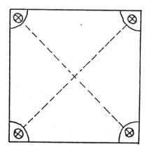
Figure 4.2 shows the usual square format of the air photograph and the <u>fiducial marks</u>. These marks are located within the camera and are exposed onto the negative as each photo is taken. During camera calibration the fiducial marks are adjusted so that when opposite marks are joined they:
