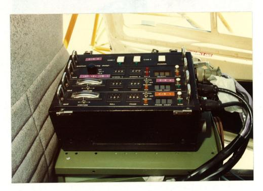
Hasselblad 500 EL/M cameras were introduced for the 1980/89 photography to overcome the measurement problems caused by the Vintens' focal plane shutters. Three Hasselblad 500 magazines were obtained, giving the cameras a reasonable film capacity and a new camera control system was built. A reseau plate was installed in each camera to facilitate measurements by analytical plotter.
