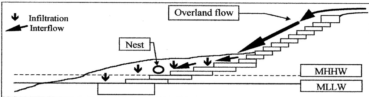
Figure 5. Diagram of a beach armored with a soil cement step-faced revetment. The nest is close to the swash zone, the depth is limited by the steps of the revetment. There is a significant discharge from overland flow and interflow.
