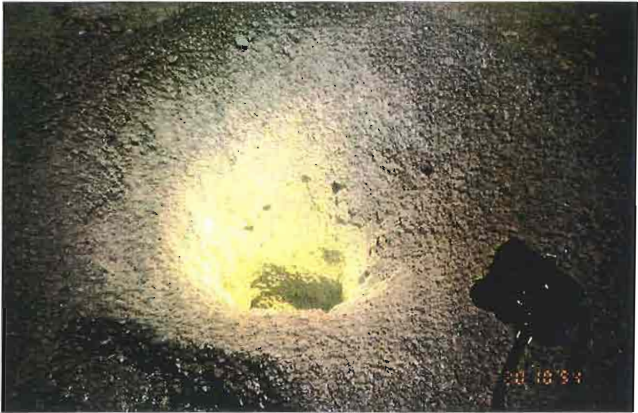
Plate 1a Mt Whaleback Precipitation of Sulphur from venting SO 2 gas at a recently completed blast drillhole in the reactive McRae Shale unit.
