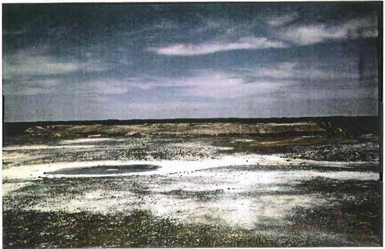
Plate 6a Puddle on coarse ore stockpile with pH measured at 3.2.
