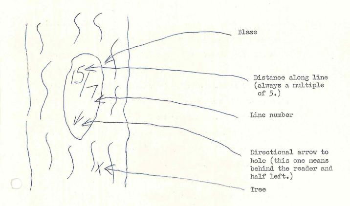
In very thick scrub, the hole itself should be pegged and the peg should show distance and line number. A good clear line should be slashed under these conditions as for other survey lines.
