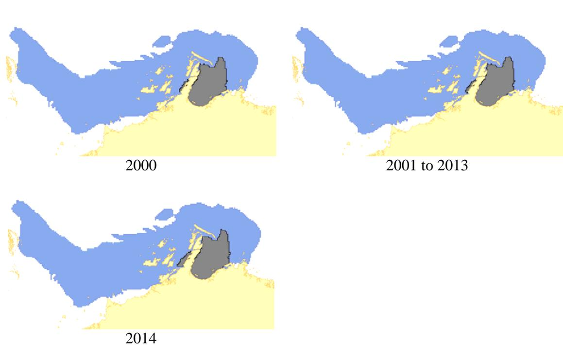
**Figure 5.1.8:** Critical areas for sulphates through time (blue is the total potential footprint and the grey indicates the area where the concentrations may exceed hypothetical ANZECC guidelines).
