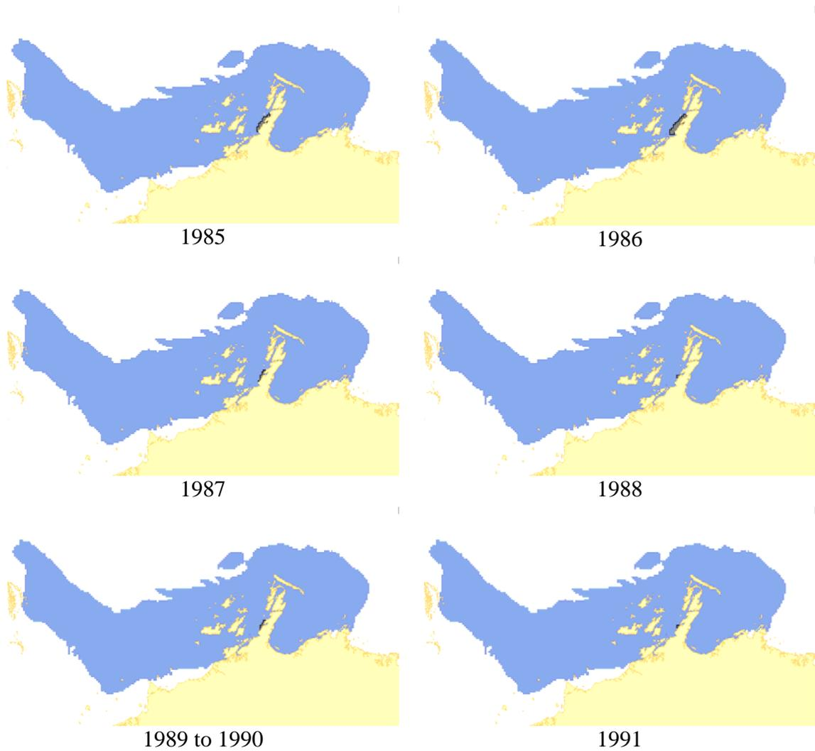
**Figure 5.1.6:** Critical areas for sulphates through time (blue is the total potential footprint and the grey indicates the area where the concentrations may exceed hypothetical ANZECC guidelines).
