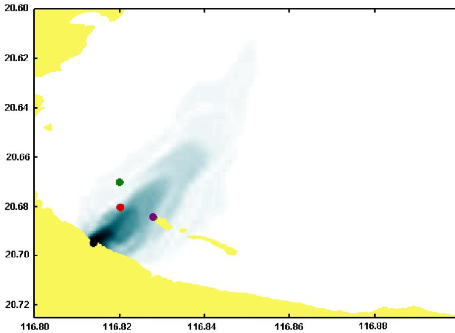
**Figure 5.2.1:** Location of three logger stations and a representative plume in Nickol Bay (green is station A, red is station B and purple is station C).
