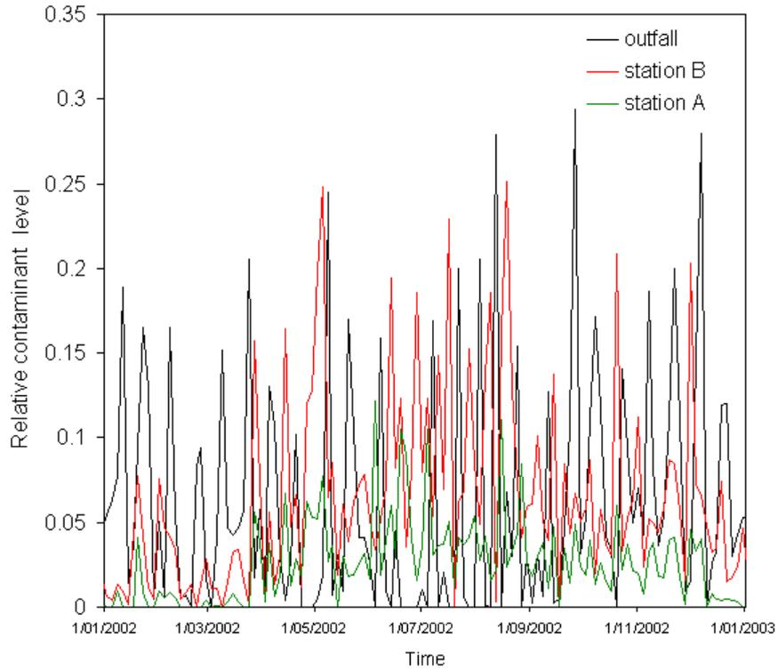
**Figure 5.2.3:** Relative contaminant signal strength at Nickol Bay outfall (black) and logger stations A (green) and B (red).
