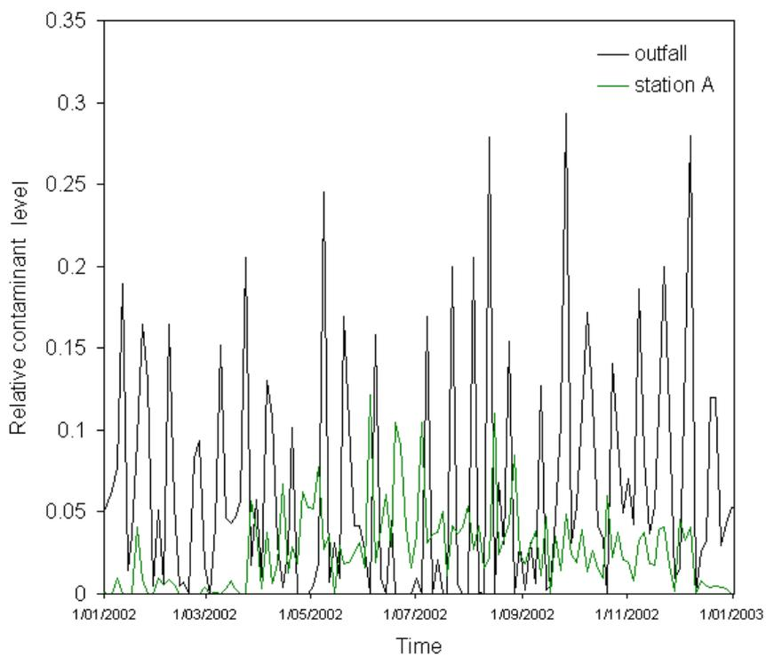
**Figure 5.2.2:** Relative contaminant signal strength at Nickol Bay outfall (black) and logger station A (green).
