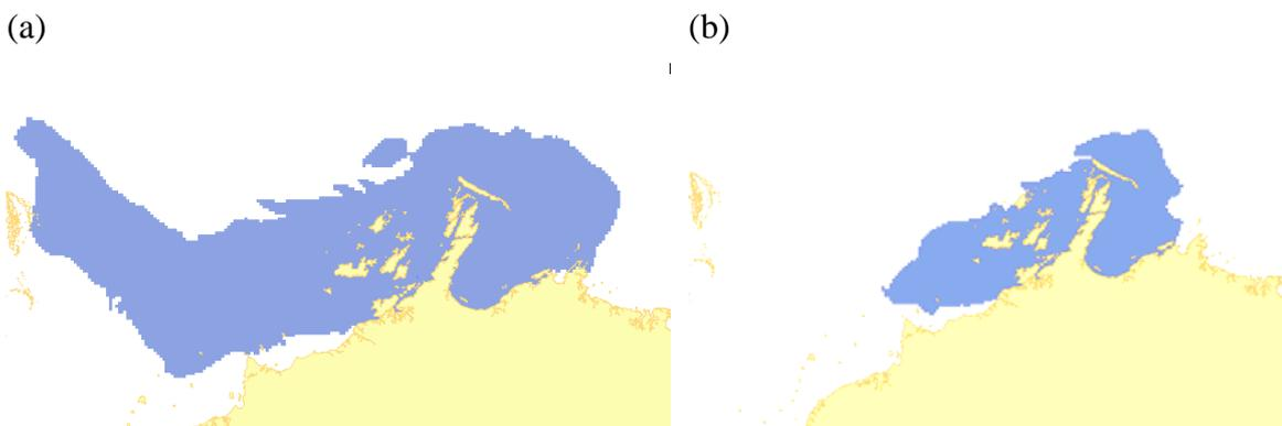
**Figure 5.1.1:** Total footprint of the combined plumes from the Nickol Bay, Mermaid Sound and Hammersley outfalls (a) at the surface, (b) depth averaged.
