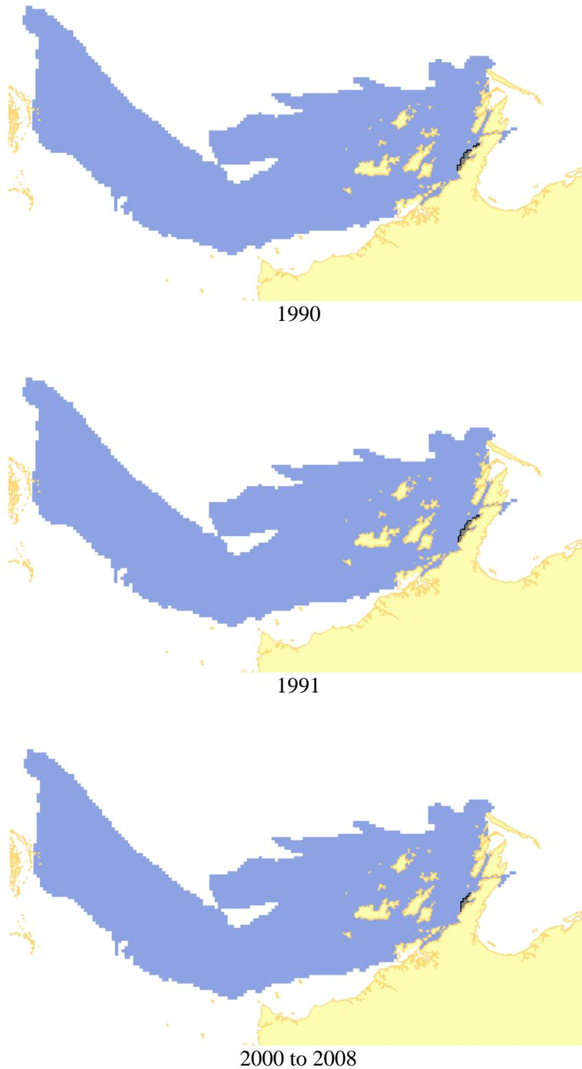
**Figure 5.1.3:** Continued. Cadmium footprint through time (blue is the total potential footprint in the water column and the grey indicates the area where the concentrations may exceed ANZECC guidelines).
