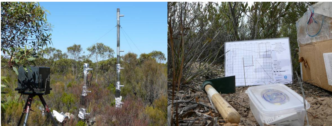
Photo 2: Thermal Environment Radiometer and camera in fire proof box - Block AS3
