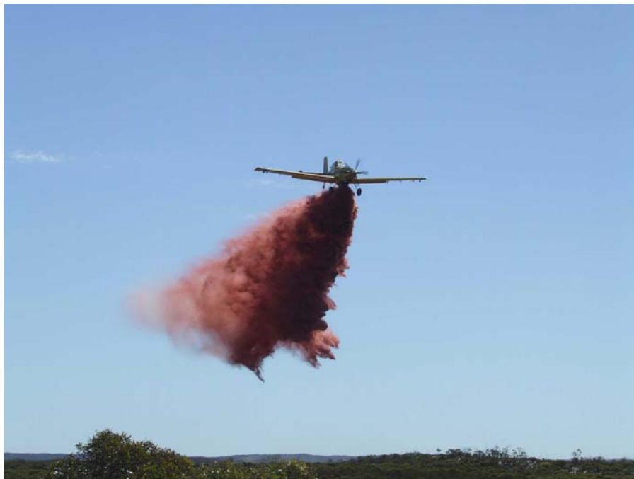
Photo 1: Water Bomber releasing chemical suppressant (Phoscheck) prior to ignition.
