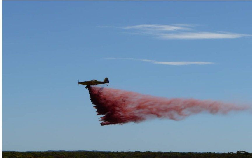
Photo 8: Water Bomber releasing chemical suppressant (Phoscheck) prior to burn trial.
