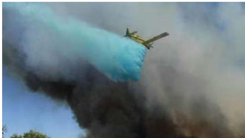
Photo 9: Water Bomber releasing chemical suppressant (foam) during burn trial. Photo Source: Bushfire CRC
