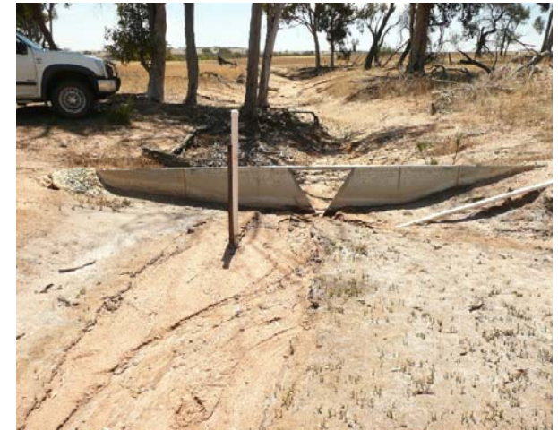
D-notch weir and piezometer at one of the 25 sites on which monitoring is occurring to evaluate the hydrological impacts of the STF plantings.
