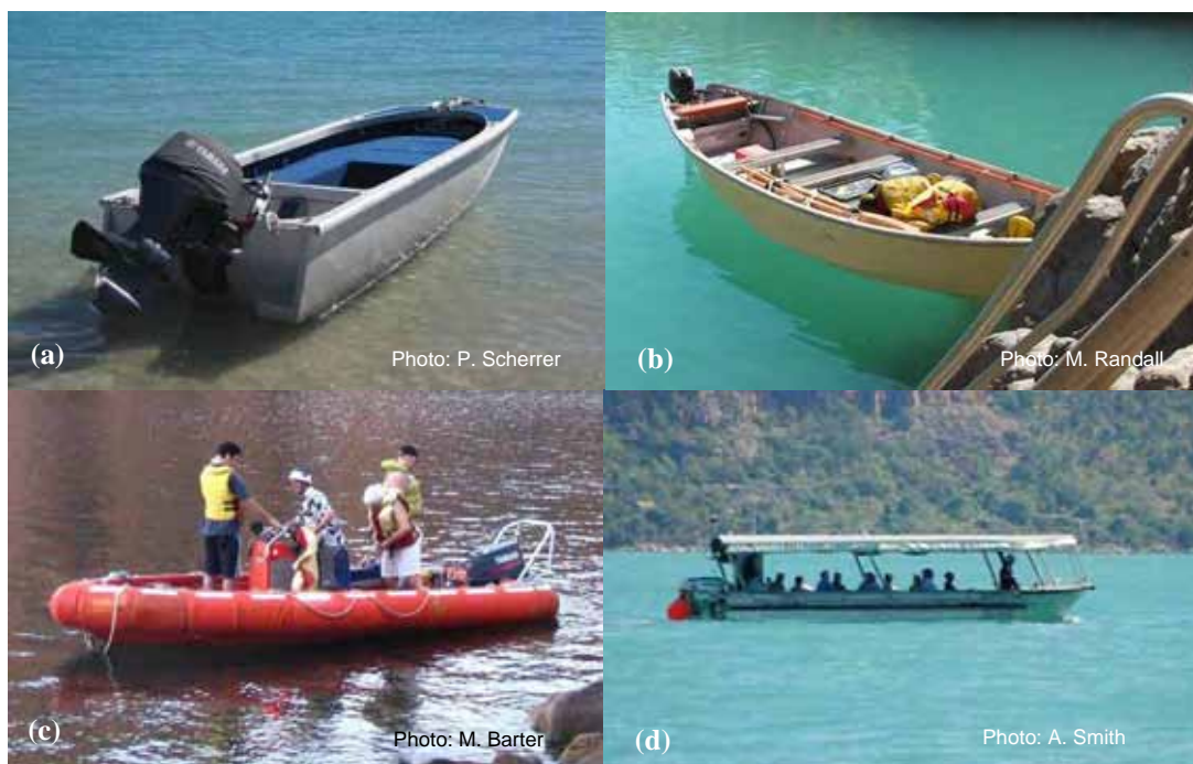
Figure 12: Types of tender vessels used by expedition cruise vessels along the Kimberley coast: (a) dinghy, (b) dory, (c) IRB, (d) purpose built excursion vessel. Note: Vessel identifiers have been removed on images.
