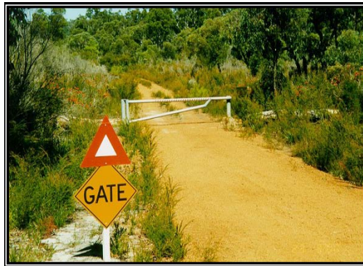
Figure 6. Managing the use of roads retained within uninfested areas with gate & warning signs.
