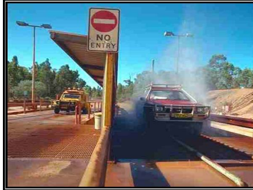
Figure 8. Vehicles are cleaned before entering uninfested areas
