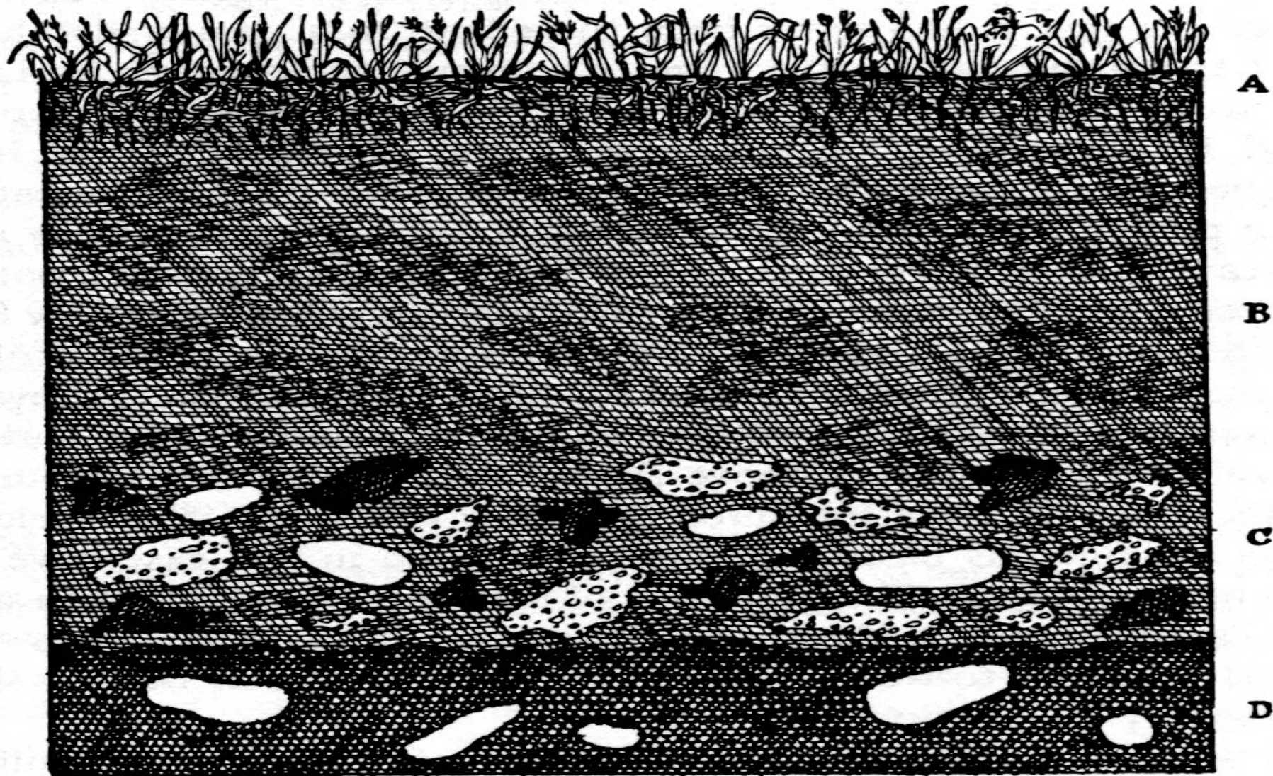
FIG. 5. Section, reduced to half the natural scale, of the vegetable mould in a field, drained and reclaimed fifteen years previously; A, turf; B, vegetable mould without any stones; C, mould with fragments of burnt marl, coal-cinders and quartz pebbles; D, subsoil of black, peaty sand with quartz pebbles.
