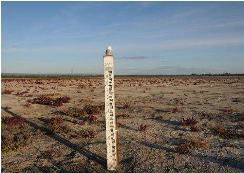
Figure 3.8: Staff gauge at Forrestdale Lake from which water depth measurements are currently recorded (taken by Jenny Davis in May 2008).
