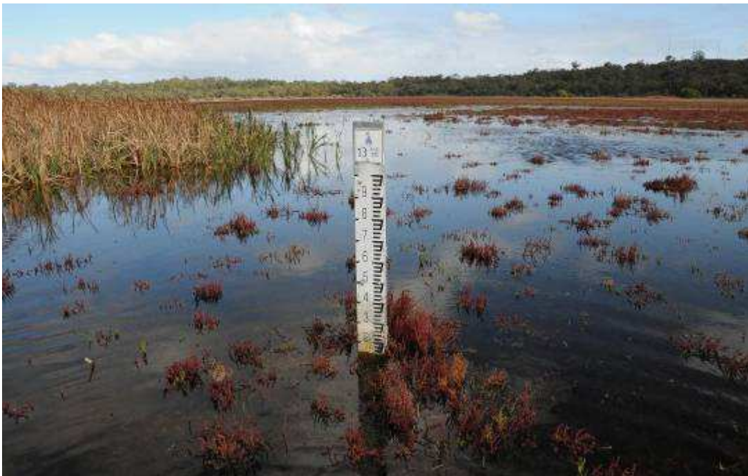
Figure 3.7: Staff gauge at Thomsons Lake from which water depth measurements are currently recorded (taken by Jenny Davis in June 2008).
