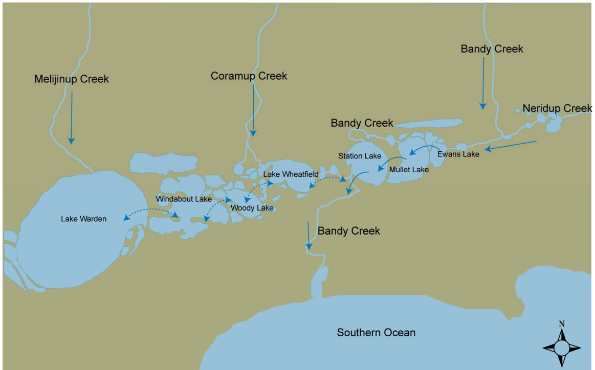
Figure 12. Conceptual surface water flows within the Lake Warden System Ramsar Site, Esperance, Western Australia.
