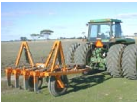
Figure 8.5. The MTR (left) with hydraulic breakout on each tyne and this implement in operation (right). This implement was designed specifically to improve revegetation site preparation in the wheatbelt.
