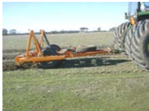
Figure 8.5. The MTR (left) with hydraulic breakout on each tyne and this implement in operation (right). This implement was designed specifically to improve revegetation site preparation in the wheatbelt.
