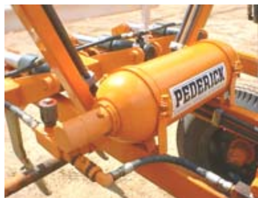
Figure 8.2. The accumulator contains pressurised nitrogen gas. The pressure set in this cylinder governs the hydraulic breakout rating.
