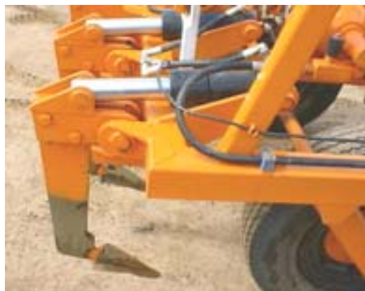
Figure 8.1. Each tyne is fitted with a hydraulic displacement ram. Breakout pressure can be adjusted.
