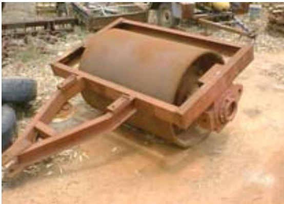
Figure 6.2. A roller suitable for rolling rip lines flat and smooth (note: in this instance, in the absence of mounds).
