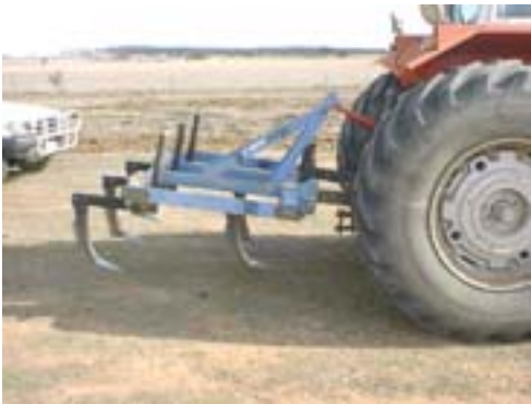
Figure 8.4. A five tyred three point linkage (3PL) Agroplough (left) and this implement in operation (right). The Agroplough has a shear pin breakout on each tyne. The shear pin mechanism limits this implement to a narrower range of soil types in comparison to a hydraulic breakout system (below). The 3PL system also has limits compared to a trailed implement.
