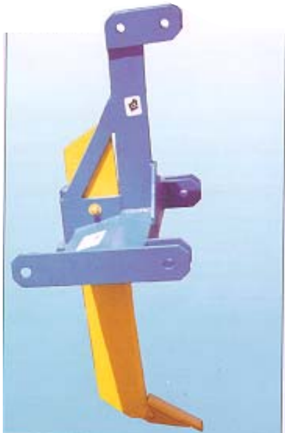
Figure 11. A basic three-point linkage ripper showing rigid tyne construction. This type is limited in its usefulness.
