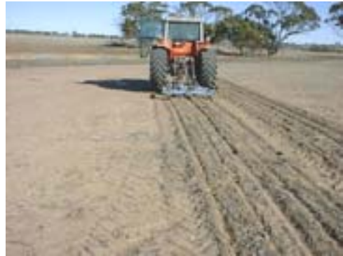
Figure 8.4. A five tyred three point linkage (3PL) Agroplough (left) and this implement in operation (right). The Agroplough has a shear pin breakout on each tyne. The shear pin mechanism limits this implement to a narrower range of soil types in comparison to a hydraulic breakout system (below). The 3PL system also has limits compared to a trailed implement.
