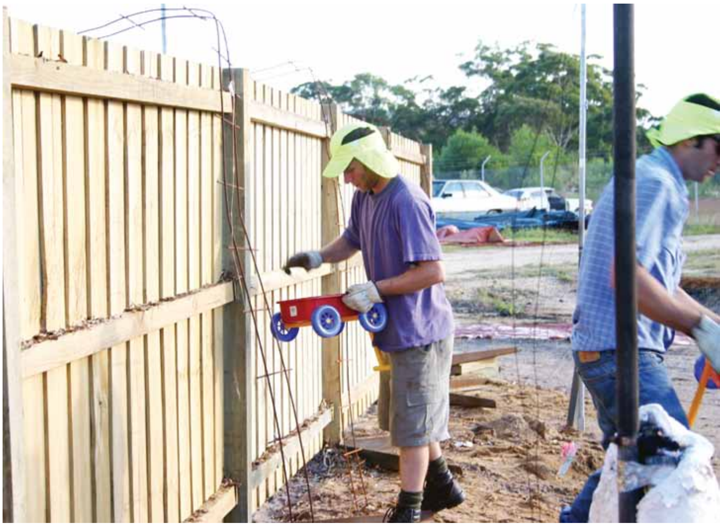
▲ Setting up timber fence for test burning.
