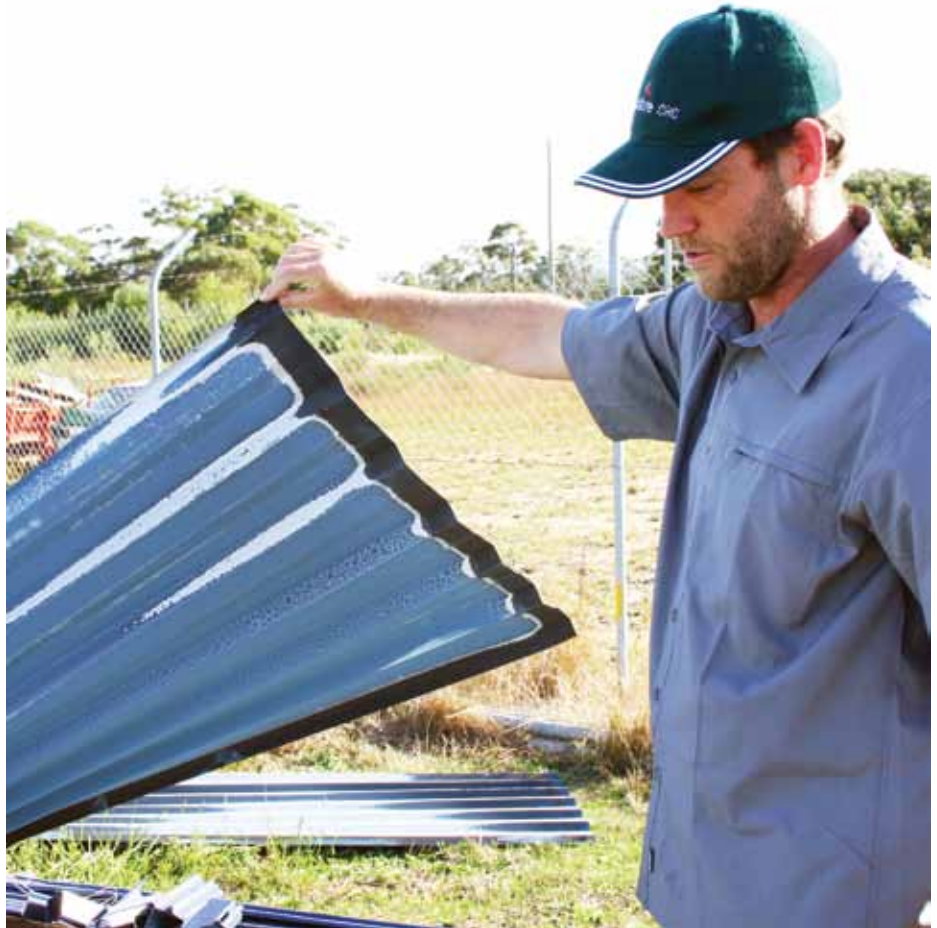
▲ Researcher Justin Leonard examines a fence after burning test at the NSW Rural Fire Service Hot Fire Training Facility.
