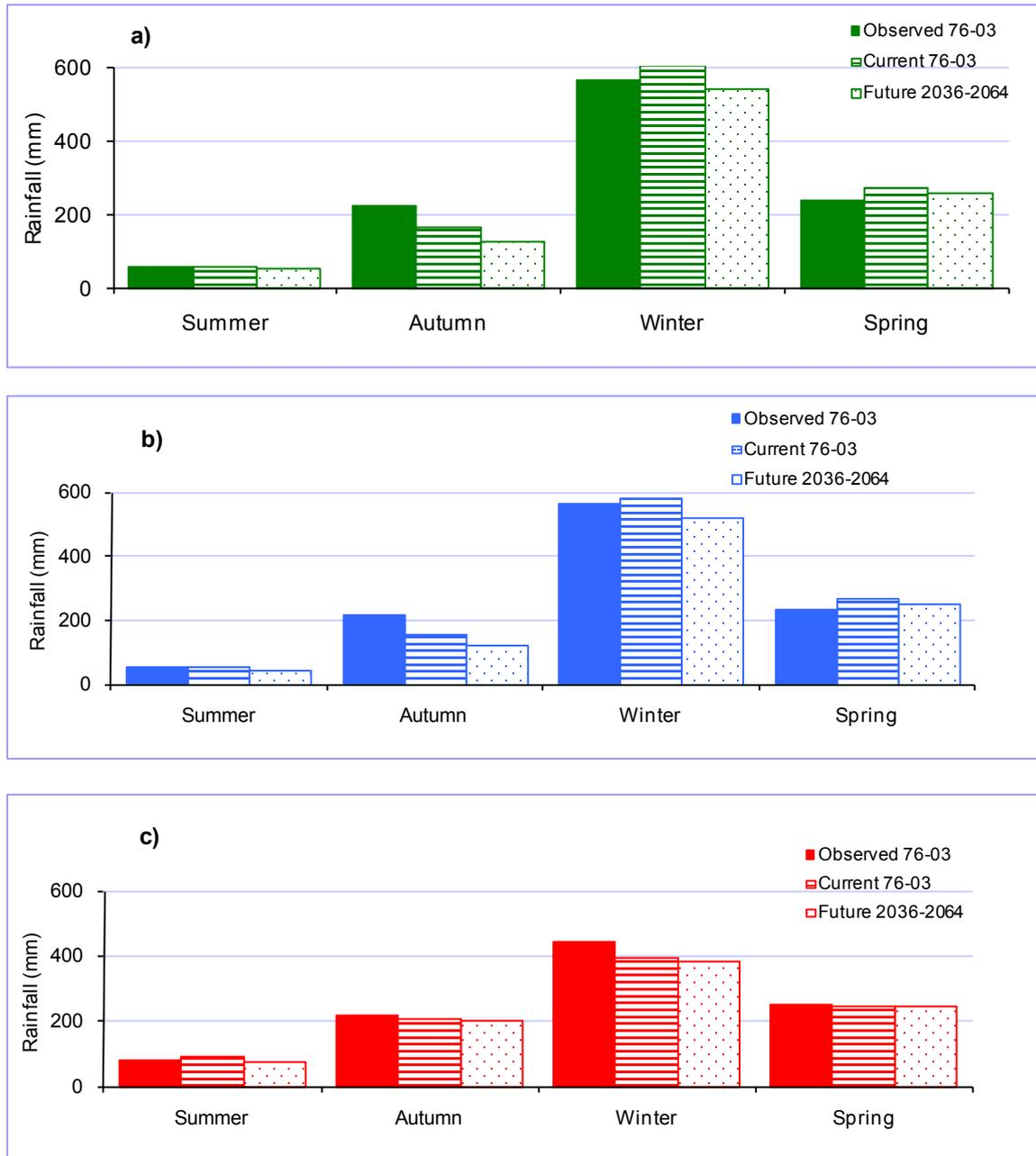
Figure 22 Mean seasonal observed, current and future rainfall for: a) Stirling Dam catchment (509197), b) Serpentine River catchment (9023) and c) Denmark River catchment (9531) for 2050
