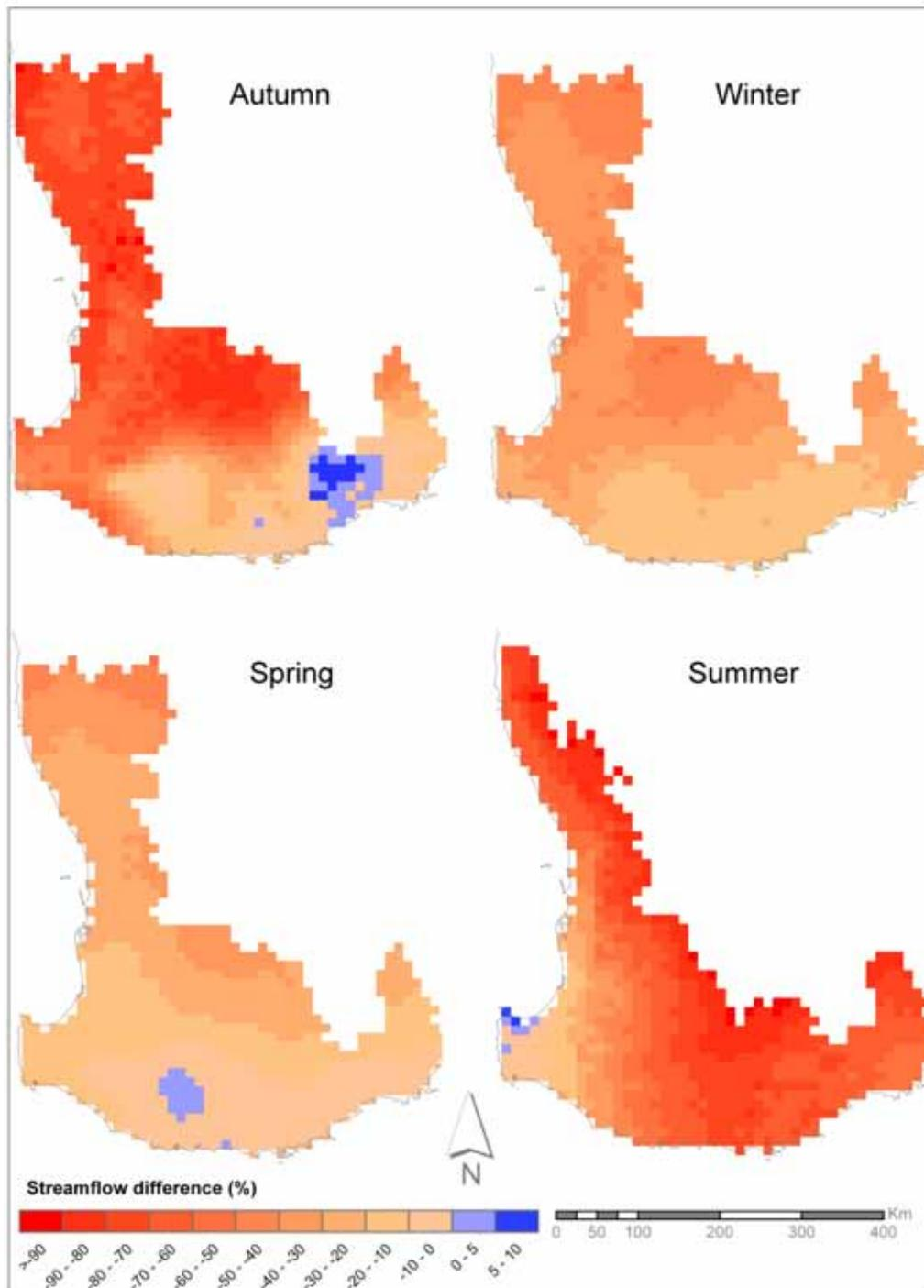
Figure 16 Mean seasonal streamflow difference for 2050 estimated using the linear equation
