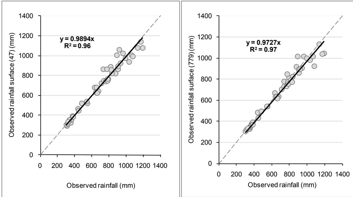
*Figure 7 Comparison of mean annual rainfall: a) observed rainfall surface created with ANUSPLIN 4.2 from data from 47 stations versus observed rainfall (point data) recorded at 47 stations, b) observed rainfall surface created with ANUSPLIN 4.2 from data from 779 stations versus observed rainfall (point data) recorded at 47 stations*
