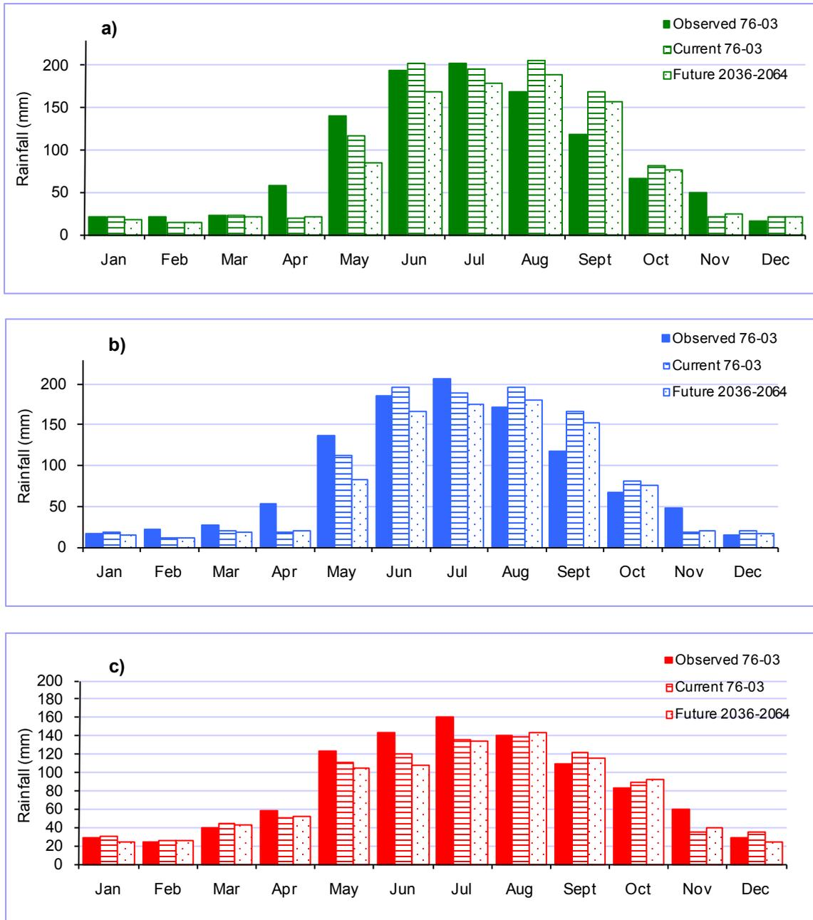
Figure 23 Mean monthly observed, current and future rainfall for three modelled catchments: a) Stirling Dam b) Serpentine River c) Denmark River
