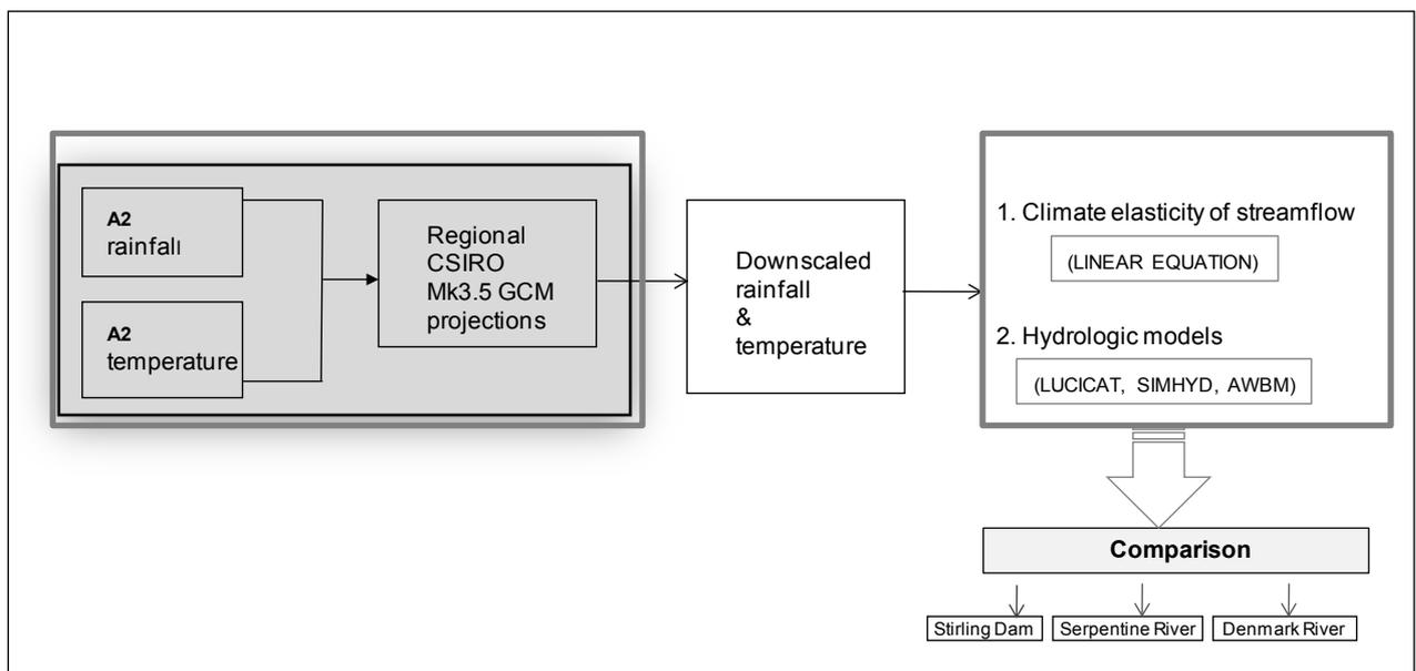
Figure 1 Project methodology schematic
