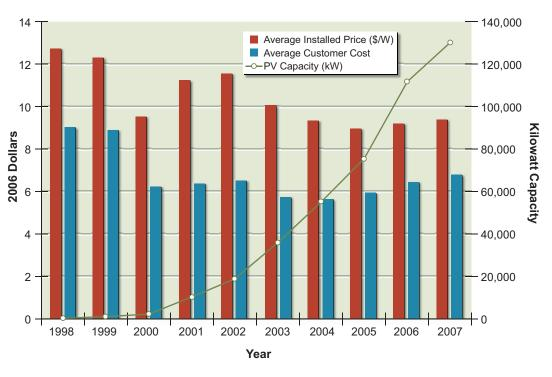
**FIGURE 4.11** Price, customer cost after subsidy, and number of PV installations per year in California under California Energy Commission incentive programs. Source: CEC, 2008.
