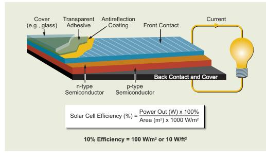
**FIGURE 3.4** Schematic of a typical solar cell. Source: DOE, 2005.
