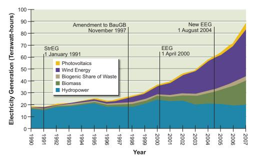
**FIGURE 4.6** Growth in electricity generation from renewable energy sources in Germany. Source: German Federal Ministry for the Environment, Nature Conservation, and Nuclear Safety, 2007.
