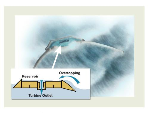
**FIGURE 3.9** Design of the Wave Dragon device. Source: Wave Dragon. Reprinted by permission.
