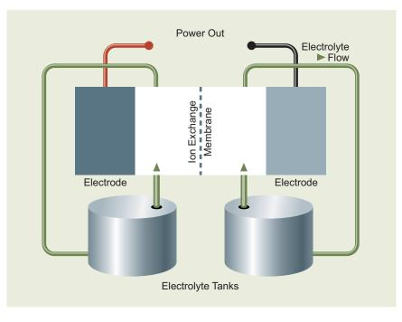
FIGURE 3.14 Schematic of a flow battery.
