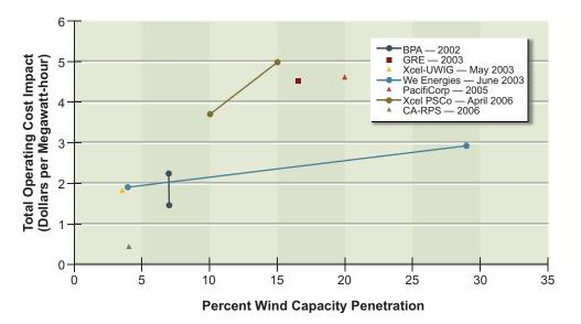
**FIGURE 4.1** Summary of wind plant ancillary services costs from various studies looking at the cost of regulation service, load following, unit commitment, and natural gas. Source: Developed from data in Smith (2007) and in Wiser and Bolinger (2008).
