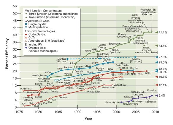
**FIGURE 3.5** *Historical progress of solar cell efficiencies. Source: NREL, 2009.*
