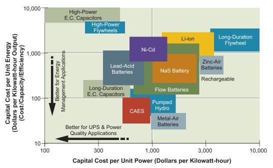
**FIGURE 4.2** Storage technolgies and costs of energy and power. Source: Electric Power Research Institute; presented in Rastler, 2008.
