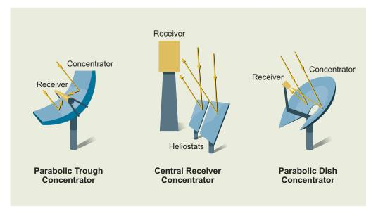
FIGURE 3.6 Optical configurations for concentrating solar power.
