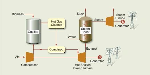
**FIGURE 3.10** *Diagram of a biopower IGCC plant. Source: Bain, 1993.*
