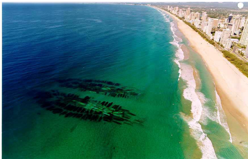
Narrowneck Queensland – Artificial Surf Reef designed to mitigate coastal erosion (Burgess et al , 2003).
