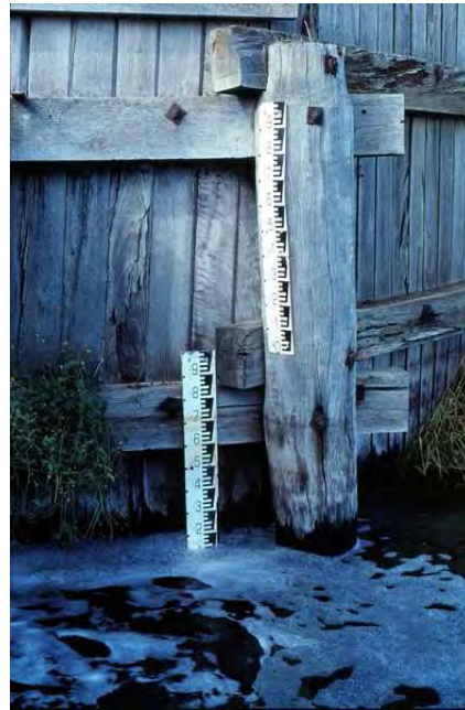
Photo 38: Subsequent Water & Rivers Commission Vasse estuary gauge boards at floodgates (16May1999).
