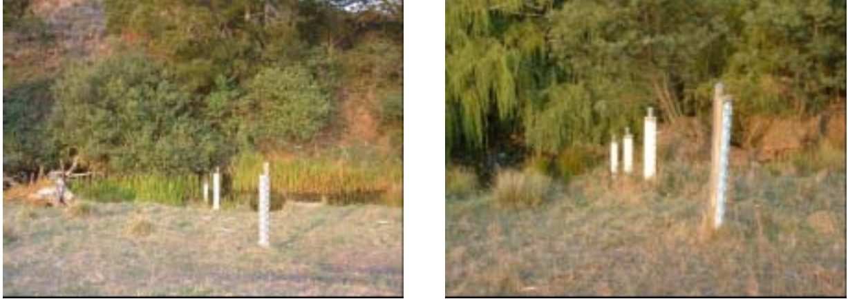
Figure 2. The gauge boards at surveyed cross-sections 2 and 3 on the Merrimans Creek at Stradbroke West.
