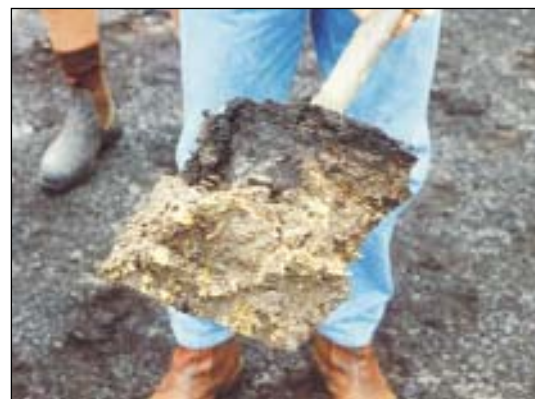
Figure 19. An example of acid sulfate soil containing yellow jarosite mottles. This was taken from a backswamp where the surface topsoil and peat had been lost through fire, creating a large acid scald. Sites like this can be a major source of acidity. (Photo: Rebecca Lines-Kelly)
