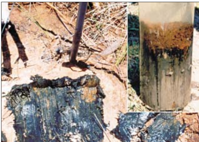
Figure 33. This photo shows MBO (the black material) in the base of a drain after scraping away the surface sediment. The inset is a vertical core in perspex taken from the bottom of a drain. It shows base sediments (grey layer) covered by MBO (black layer) and topped with iron flocs (orange layer). High drain flow velocities can scour the MBO layer and mobilise it into the water column, consuming oxygen and producing acidity. (Photo: Mitch Tulau. Inset: Scott Johnston)
