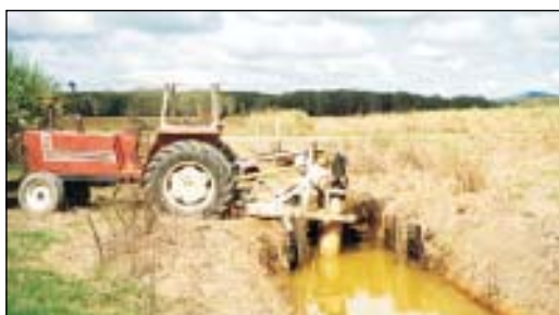
Figure 12. In low-lying areas drains are sometimes pumped to assist water removal. Lowering drain water levels by pumping in ASS areas which have high soil permeability can increase drain water acidity and enhance acid export (see Figure 31).
