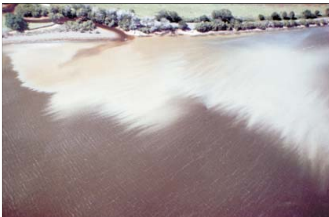
Figure 11. A large acid plume caused by flocculation of iron and aluminium which often occurs when acidic drainage water mixes with estuary water.
