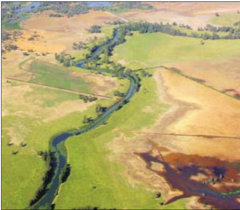
Figure 9. A drained wetland with scalding from acid sulfate soils (far right). The loss of surface vegetation greatly reduces agricultural productivity. Over-drainage of acid sulfate soils is a primary cause of such scalds. Fires, overgrazing, salinity and death of vegetation from deep flooding can be contributing factors. (Photo: Clarence River County Council)
