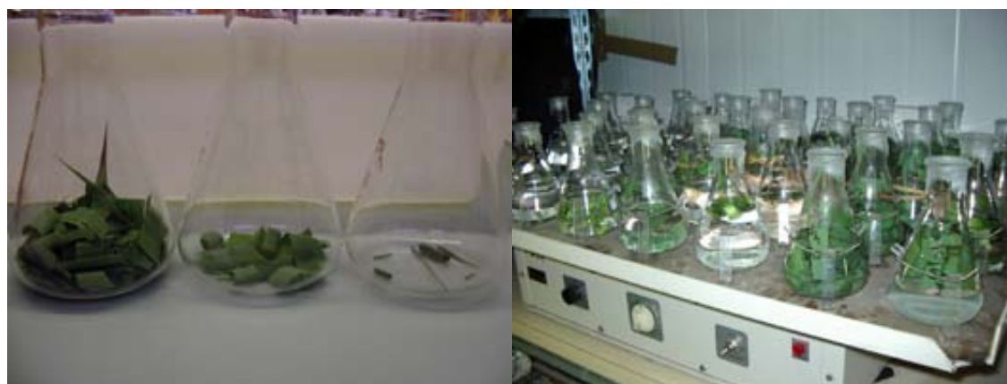
Figure 5.1. Photograph showing experimental setup: flasks containing plant tissues and RO water rest on an orbital shaker table within a darkened enclosure in a constant temperature room set to 20°C.
