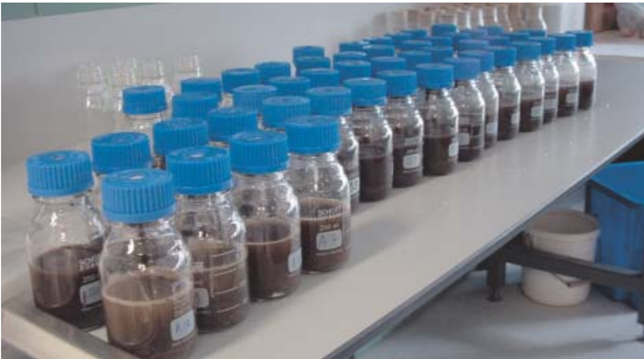
Soil samples prepared for laboratory measurement of denitrification potential. Photo Rob DeHayr.
