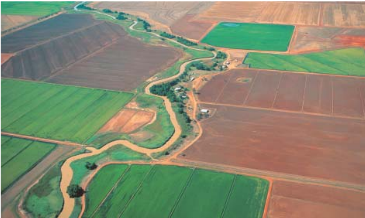
A range of erosion processes can cause water quality impacts at landscape scales, with the degree of connectivity between the sources and the river system also important. This photograph of Mirrool Creek in NSW shows cultivated paddocks in close proximity to a river. Bank erosion along the meandering river channel can deliver large amounts of sediment directly into the river during flood events. Buffer strips can provide opportunity to trap sediment and nutrients from paddocks if well managed. Photos throughout this chapter courtesy CSIRO Land and Water.
