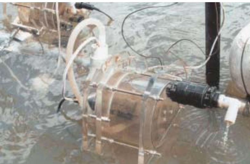
Sealed chambers used for measurement of habitat specific metabolism.
