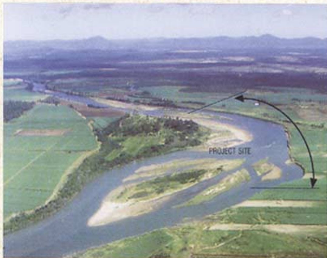
Aerial view of site. Bank erosion extending into cane land on right
