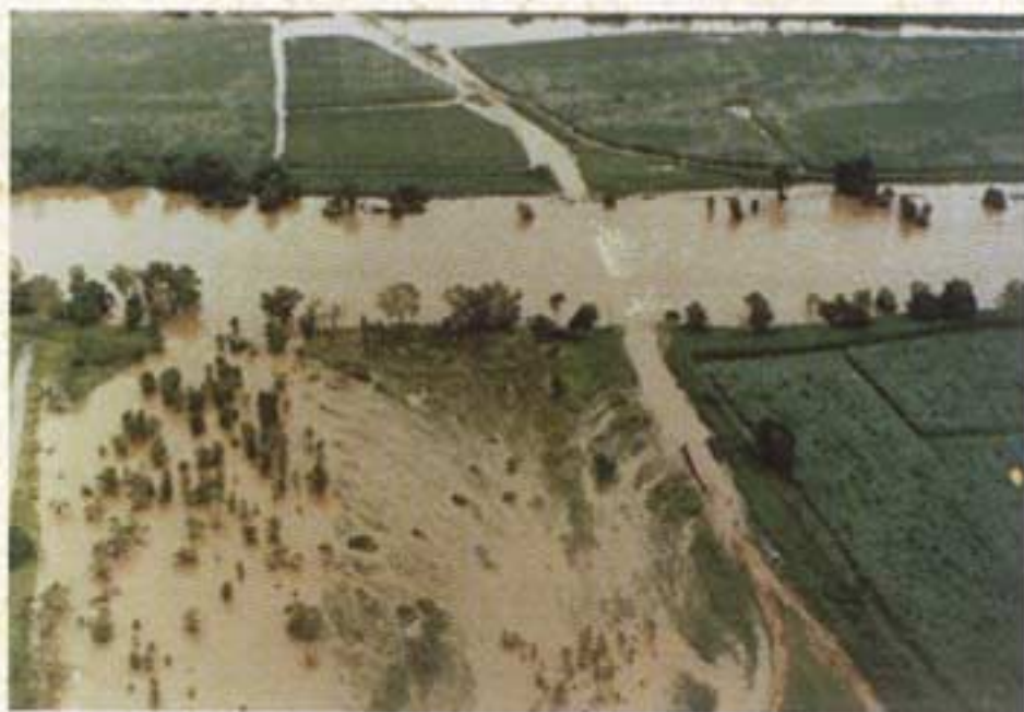
Overbank erosion from flood outflow on Haughton River near Gien
