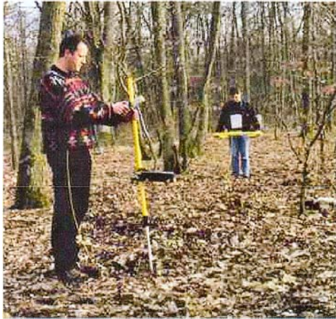
Figure 17 Iris Instruments Promis-10 wide coil spacing triple orientation receiver coil FDEM instrument
