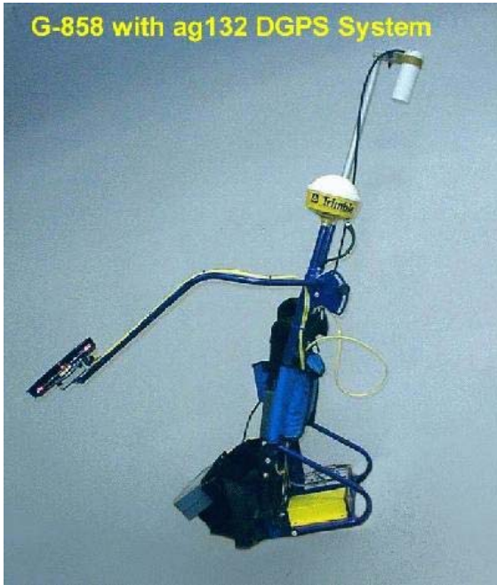
Figure 67 A backpack mounted Geometric magnetometer with a Trimble parallel swathing light bar.
