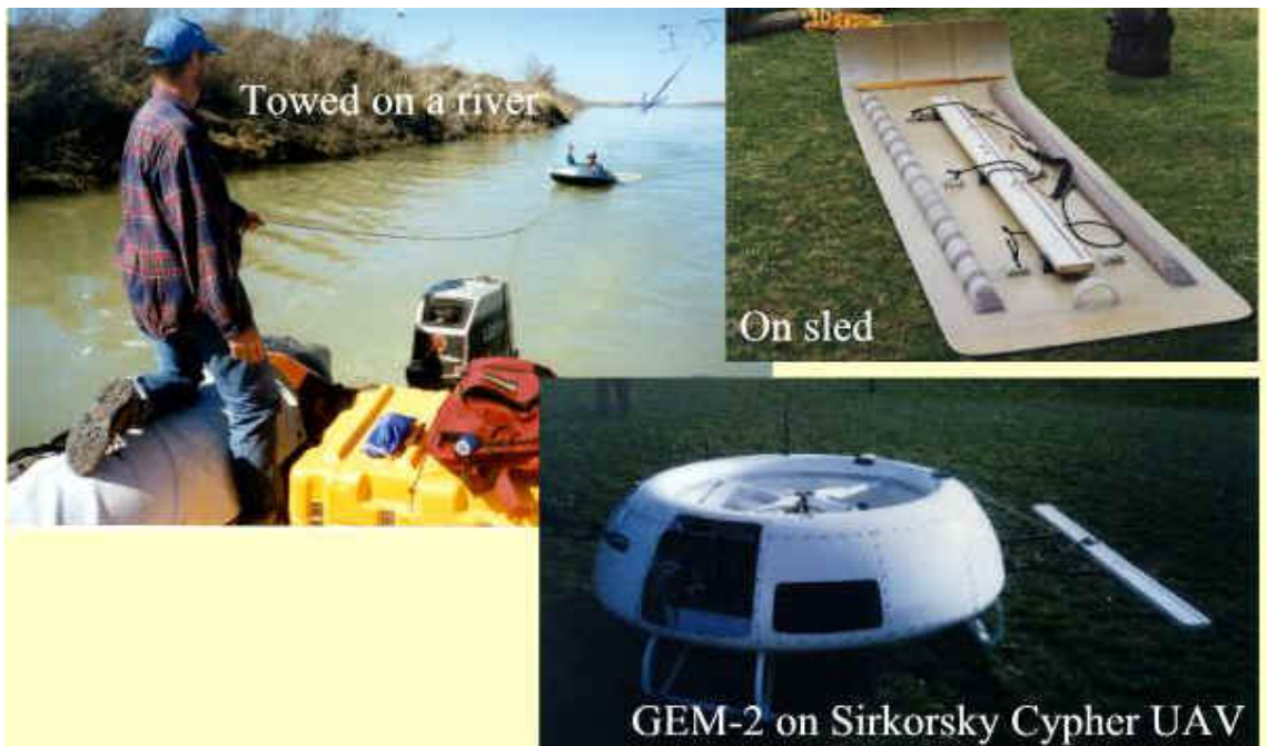
Figure 20 Various field implementations of the Geophex GEM2.
