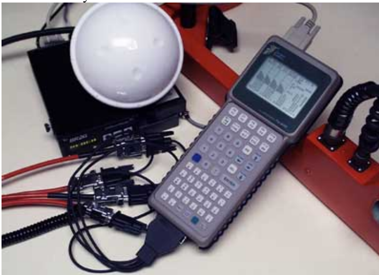
Figure 15 Allegro Pro4000 operating Geomar Multi31 (receiving GPS data and EM31 data from 3 different receiver coils).
