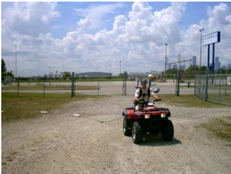
Figure 25 A capacitively coupled resistivity meter towed behind an all-terrain vehicle in Nebraska. The capacitively coupled resistivity meter (the cable and white tubes) consists of a
