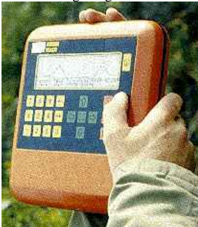
Figure 73 ABEM Wadi VLF receiver
