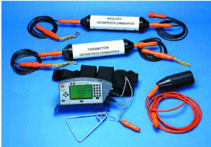
Figure 24 The Ohm-mapper with 2 transmitter and 2 receiver electrodes. A full system has 6 receiver electrodes.
