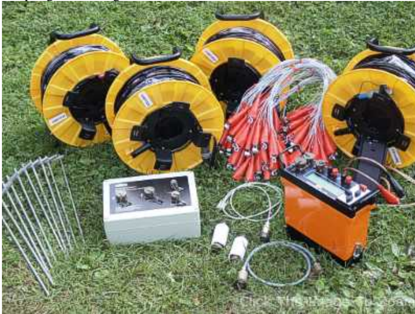
Figure 34 The ABEM Lund Resistivity Imaging System
