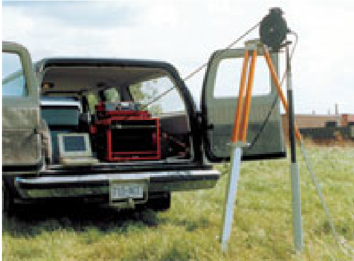
Figure 61 Geonics EM39 downhole electromagnetic induction logger. Gamma is also provided by Geonics
