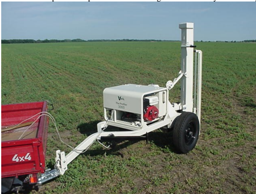
Figure 64 Veris Penetrometer with EC and pressure sensors.
