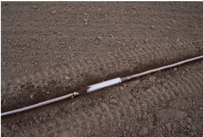
Figure 28 A PACES system electrode making contact with moist soil in a groove ploughed by the towing tractor.
