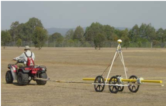
Figure 8 DualEM 2/4 being operated on a non-conductive trailer. (Photo: Alpha Geoscience Pty. Limited)
