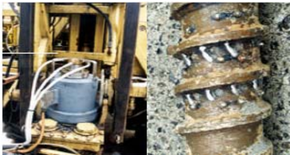
Figure 62 An auger tool set up to determine hydraulic permeability in undisturbed aquifers by injecting and withdrawing water through small holes while drilling.
