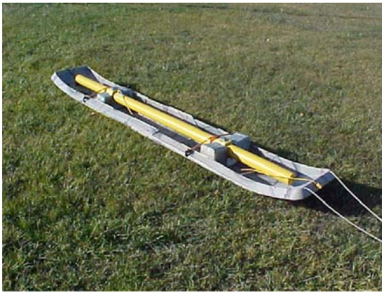
Figure 6 DualEM 2s on a rudimentary sled (Photo: John Holman, USDA-ARS)
