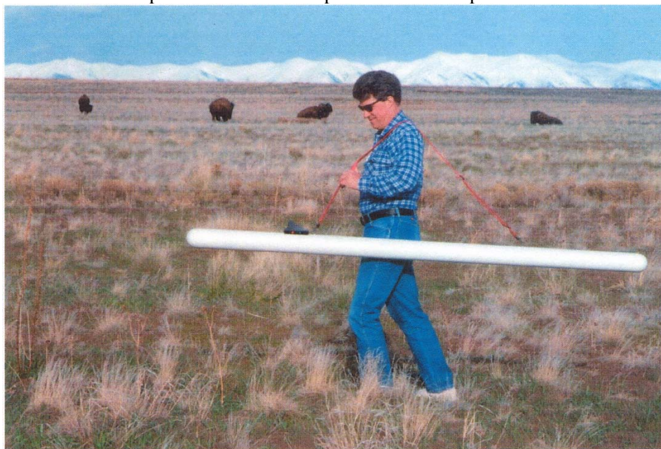
Figure 18 L&R Instruments MiniEM
