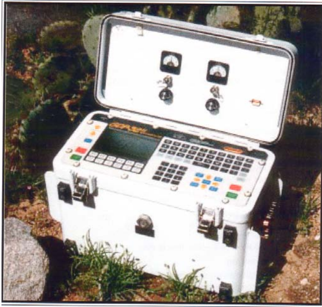
Figure 44 The Zonge GDP32-2 with an embedded NanoTEM Transmitter.
