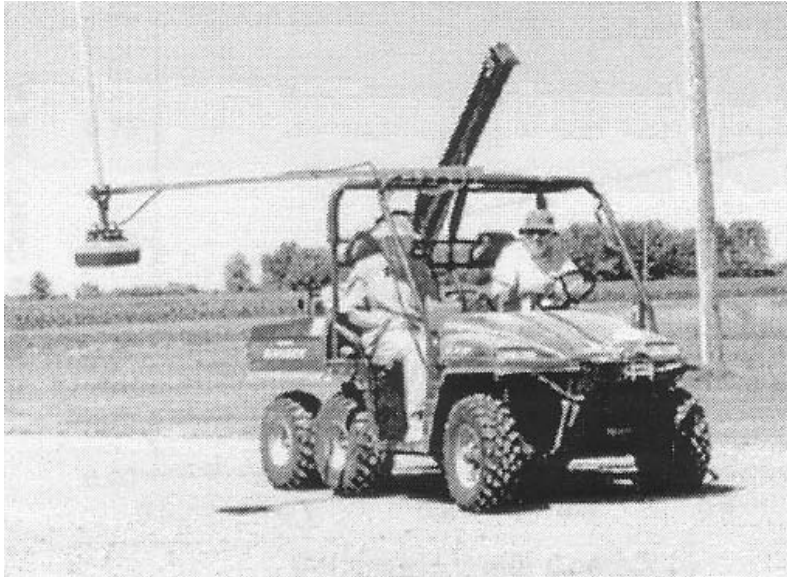
Figure 65 An elevated 500-MHz ground penetrating radar (GPR) system being used to measure soil moisture content using surface reflection amplitude (from Huissman, 2003).
