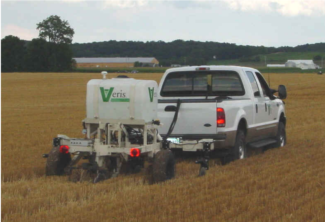
Figure 29 The Veris mobile sensor platform with electrodes sensing EC at 0.0-0.3m and 0.0 to 1.0m and pH at 0.1m depth every 12 seconds.
