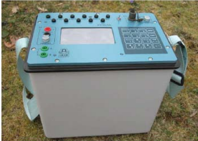
Figure 39 The Iris Instruments Syscal Pro geoelectric imaging device.
