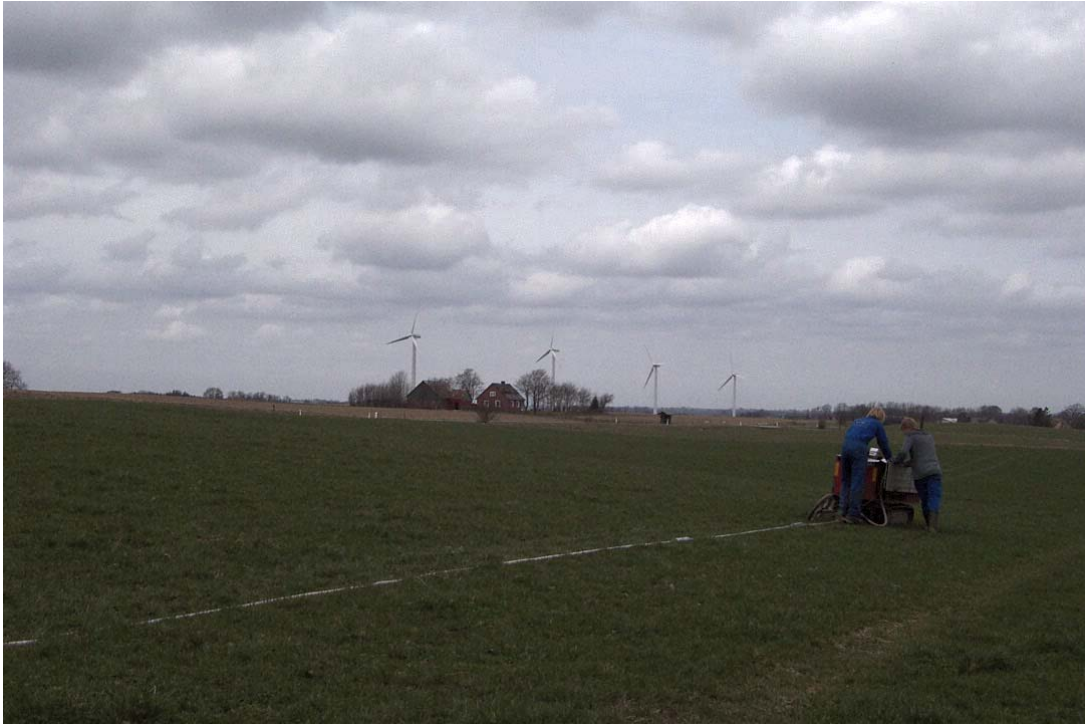
Figure 27 The PACES device being towed along near Aarhus, Denmark. The 300kg 90m long geo-electric cable is being towed behind a tracked vehicle similar to the Australian ‘Dingo’ mini-earthmover. The system images to a depth of about 30m provided that the ground is moist.
