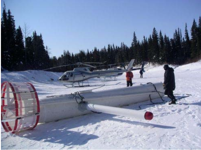
Figure 56 Impuse helicopter-borne frequency domain electromagnetic system.
