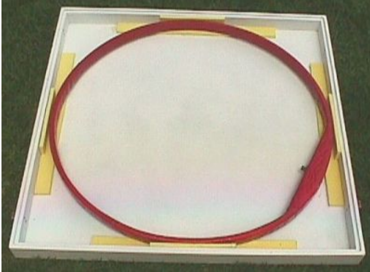
Figure 16 A Red Dog's DT Barlow FDEM-8 system coil. The system uses two coils, a transmitter and a receiver, like the Geonics EM34 but has some advantages over the EM34 including affordability.
