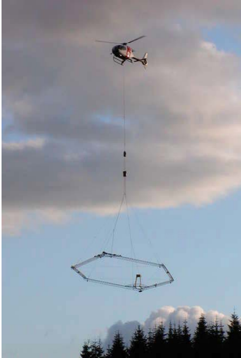
Figure 47 SkyTEM rigid helicopter-borne transient electromagnetic system with null coupled receiver coil.
