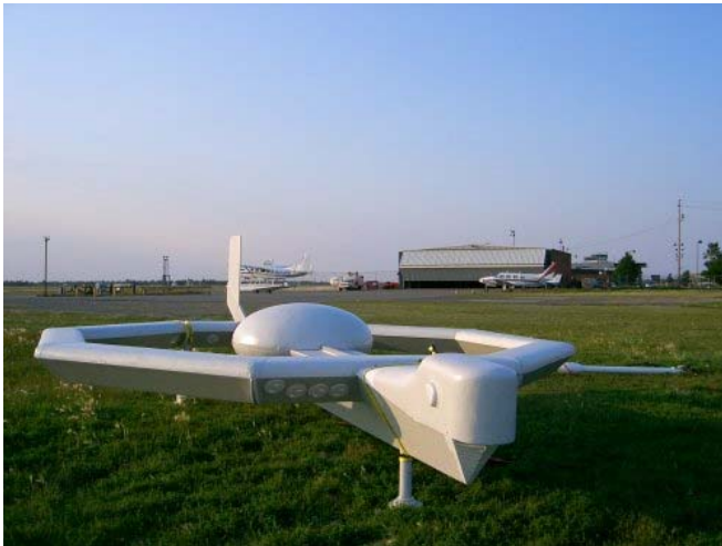
Figure 57 UFO discovered in Toronto – no. AeroTEM helicopter-borne rigid transient electromagnetic system.
