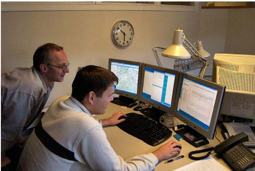
Figure 49 SkyTEM interactive processing. Fences and powerlines are identified on a map showing flightlines and data at the intersections is manually observed and removed if it appears as if it could be affected.
