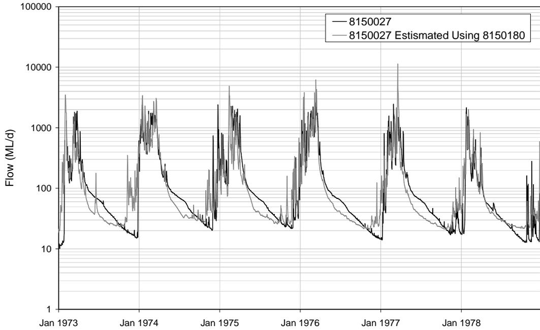
■ **Figure C-3: Comparison of Gauged and Estimated Flow at 8150027**
