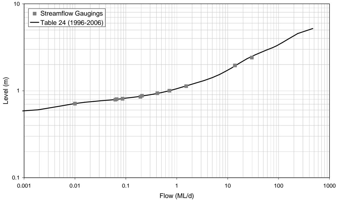
■ **Figure A-85: Rating Table 24 and Streamflow Gaugings for 8170066 (1996-2006)**
