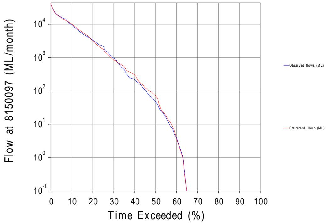
■ **Figure D-9 Monthly SIMHYD Flow-Duration Curve - East Finniss River at Rum Jungle (G8150097)**
