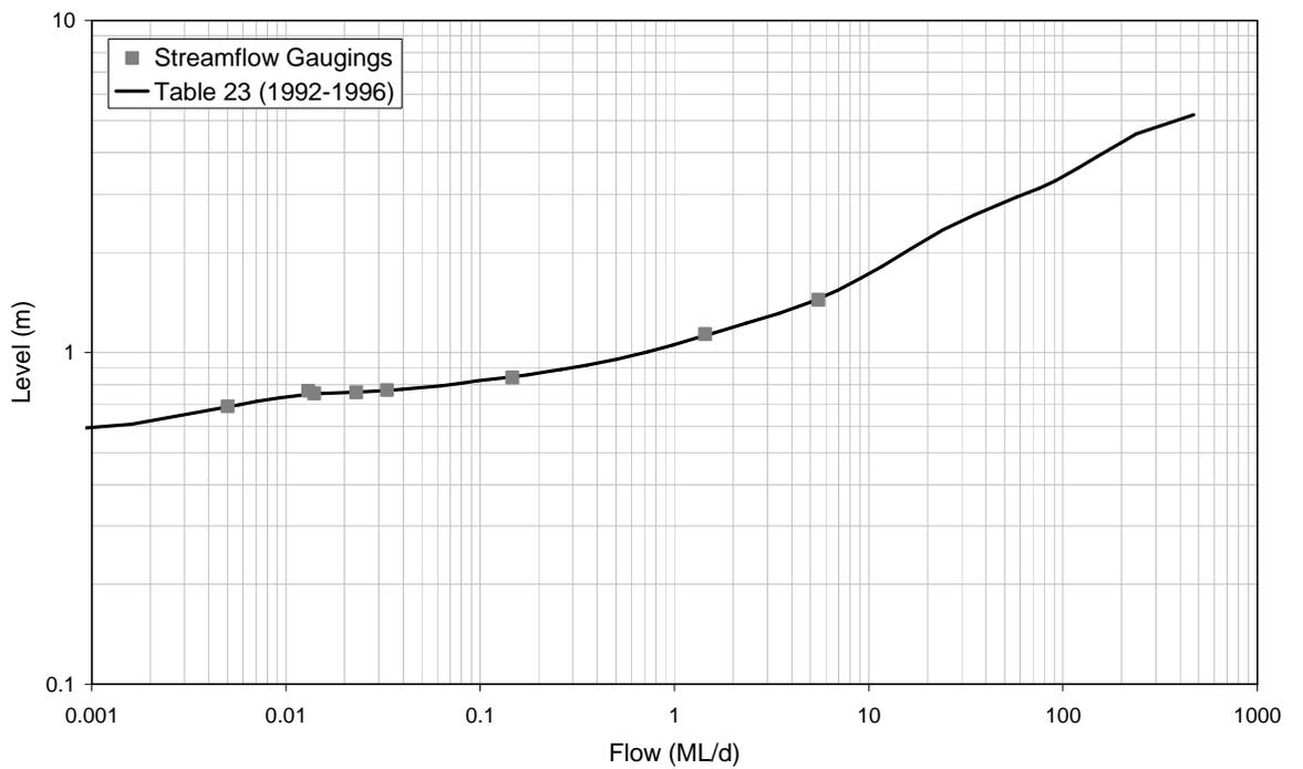
■ **Figure A-84: Rating Table 23 and Streamflow Gaugings for 8170066 (1992-1996)**
