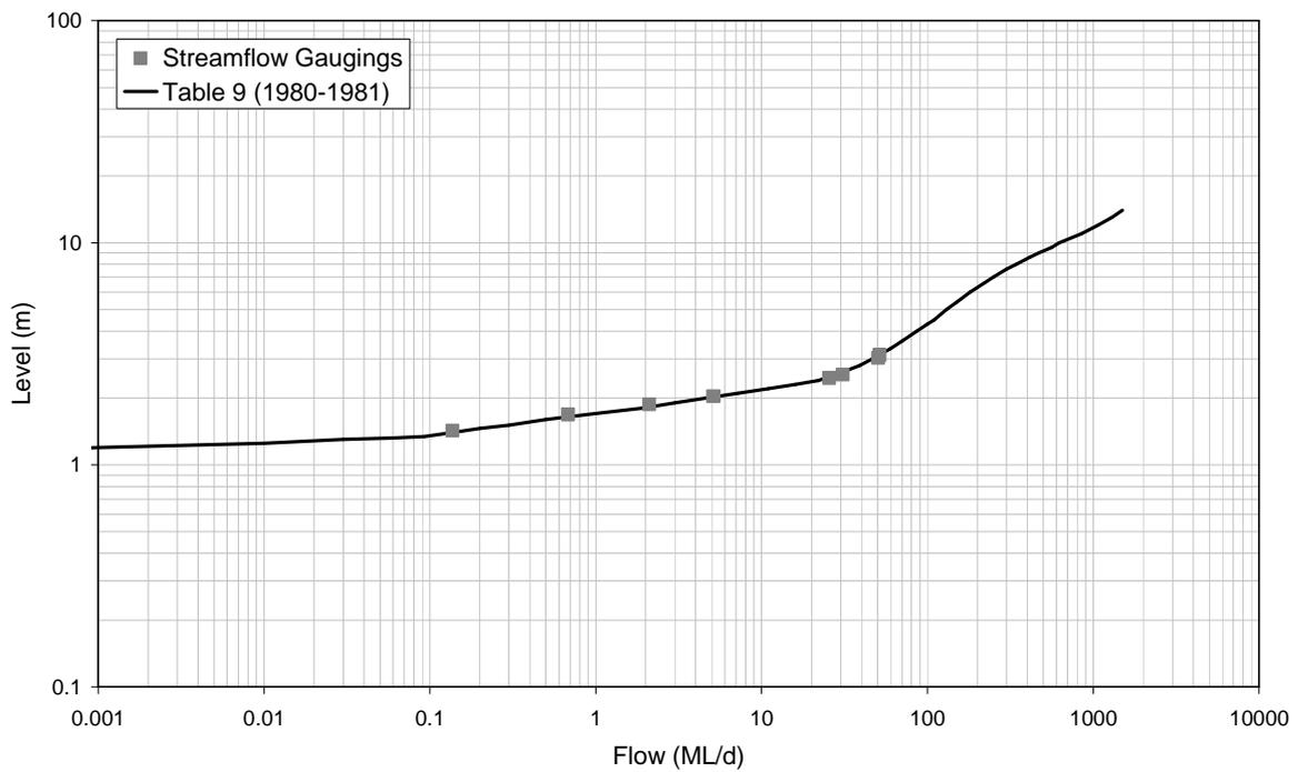
■ **Figure A-47: Rating Table 9 and Streamflow Gaugings for 8170002 (1980-1981)**
