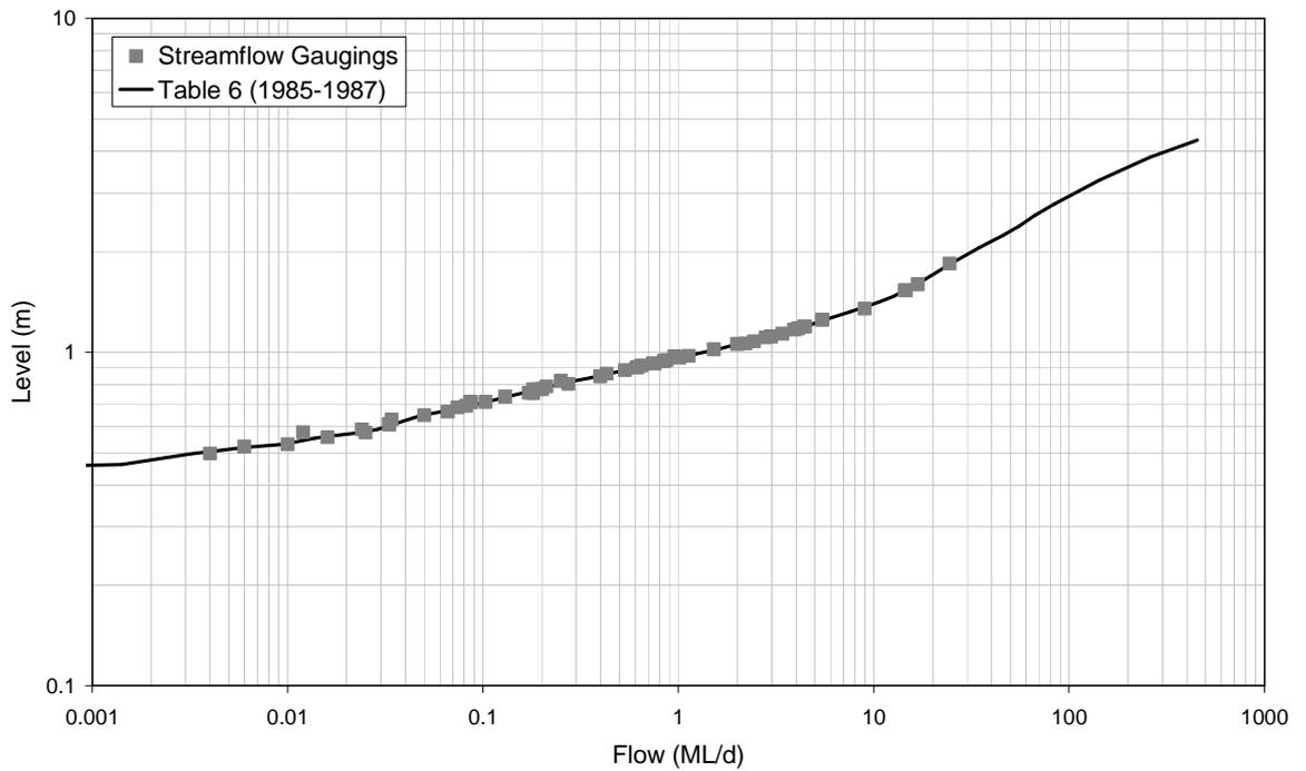
■ **Figure A-18: Rating Table 6 and Streamflow Gaugings for 8150097 (1985-1987)**
