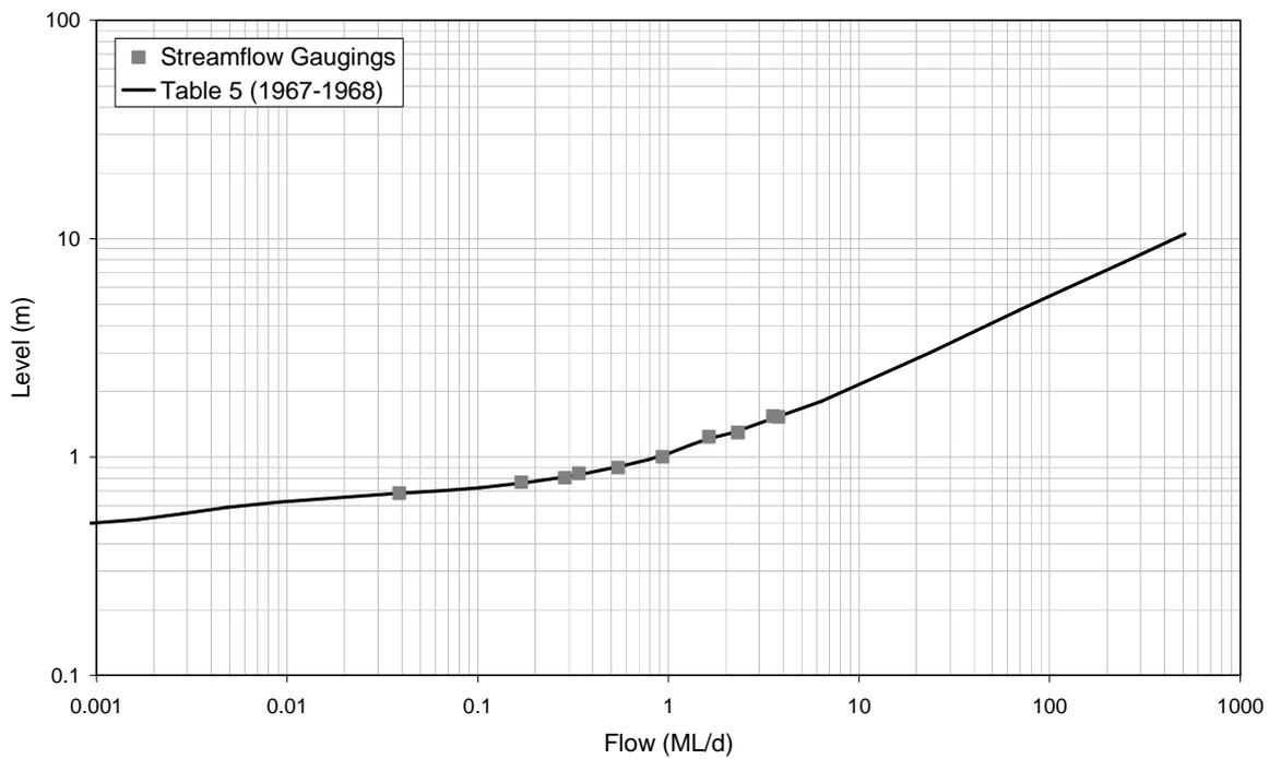
■ **Figure A-52: Rating Table 5 and Streamflow Gaugings for 8170005 (1967-1968)**
