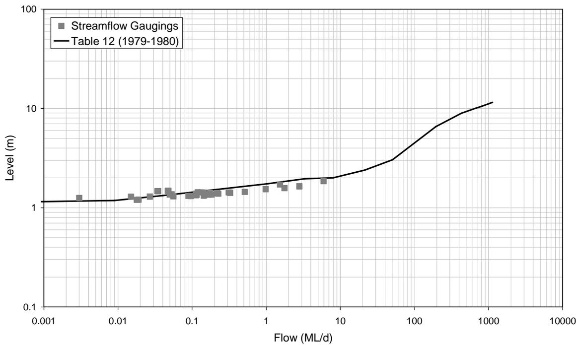
■ **Figure A-45: Rating Table 12 and Streamflow Gaugings for 8170002 (1979-1980)**
