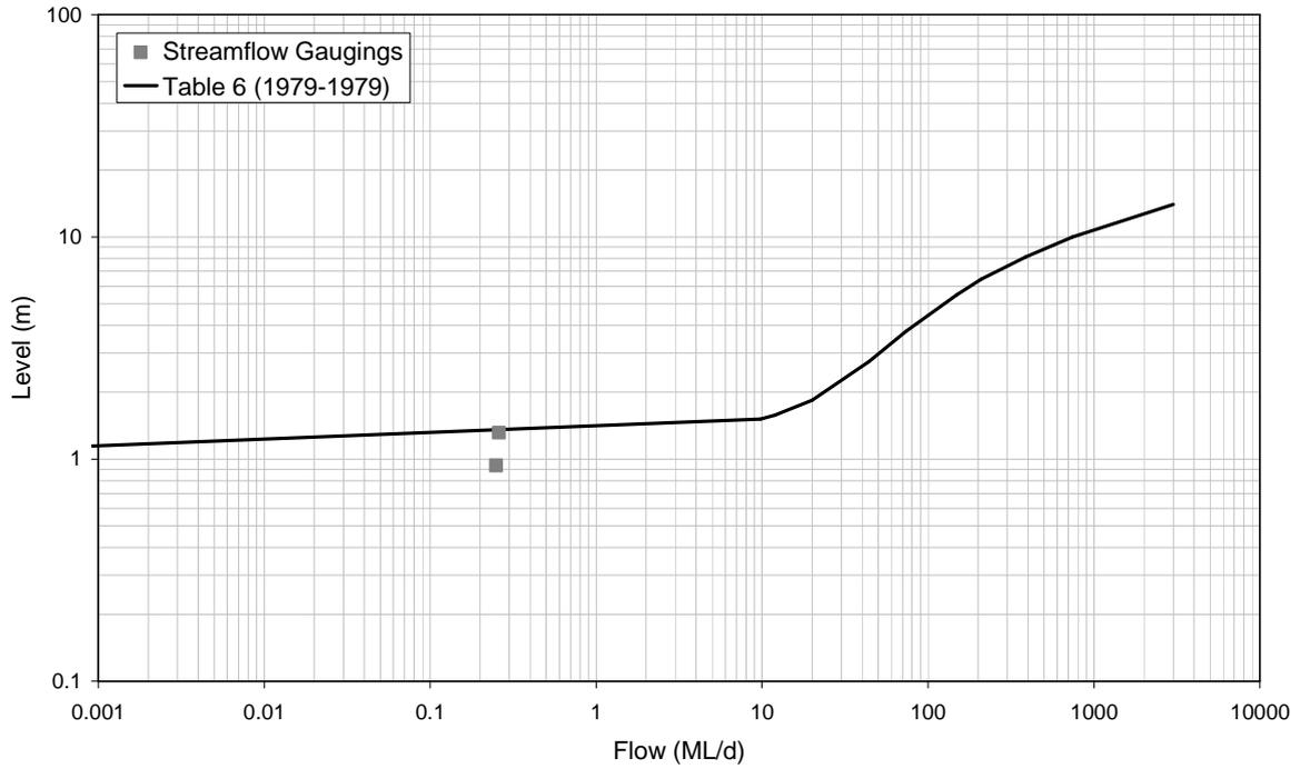
■ **Figure A-44: Rating Table 6 and Streamflow Gaugings for 8170002 (1979)**
