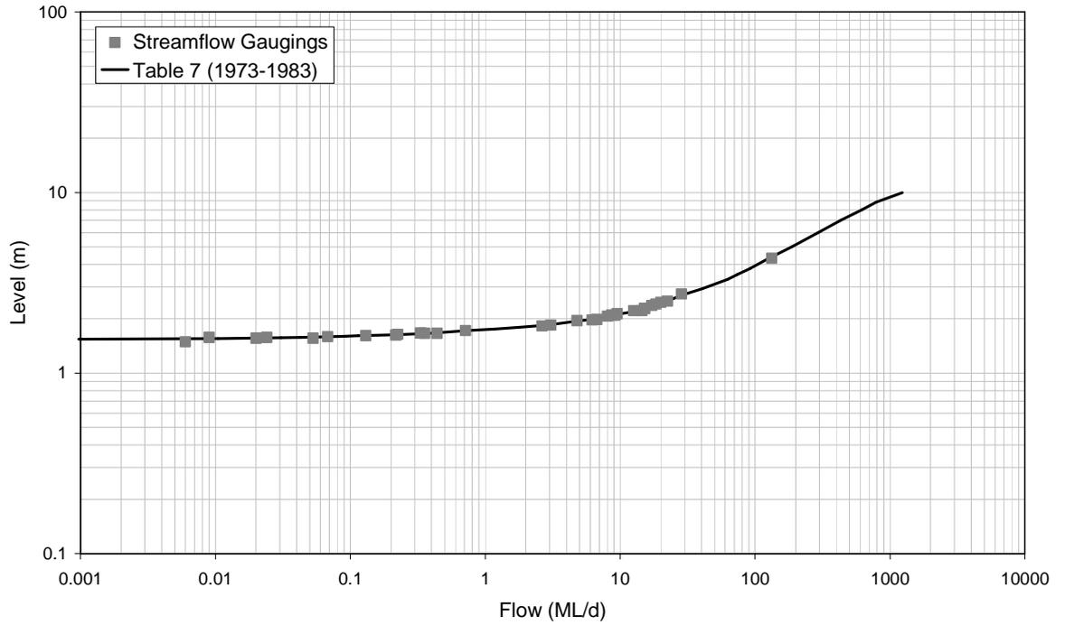
■ **Figure A-24: Rating Table 7 and Streamflow Gaugings for 8150098 (1973-1981)**
