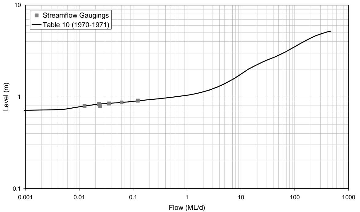
■ **Figure A-72: Rating Table 10 and Streamflow Gaugings for 8170066 (1970-1971)**
