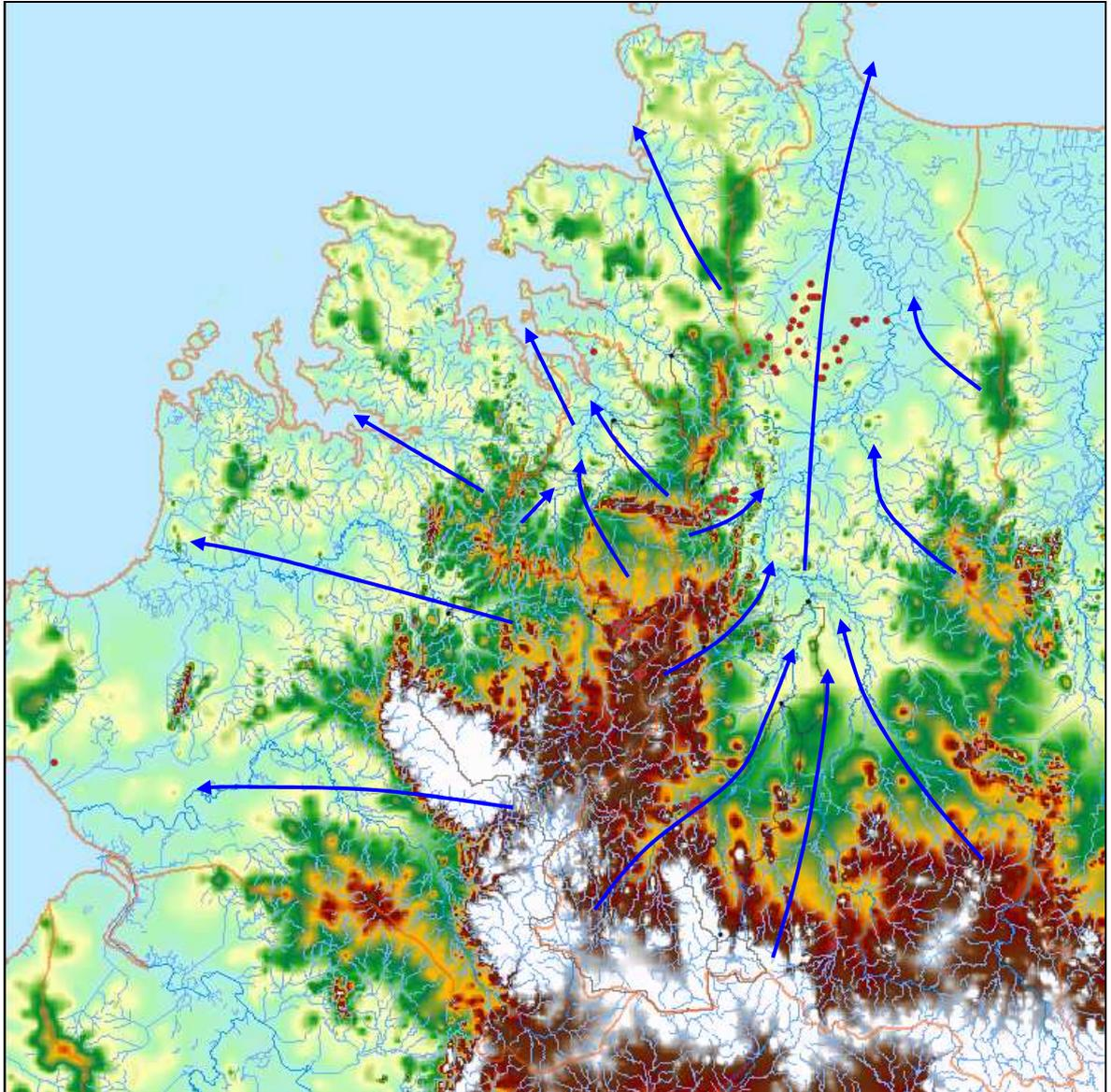
■ **Figure F-2: Initial Conceptualised Groundwater Flow Directions Based on DEM**
