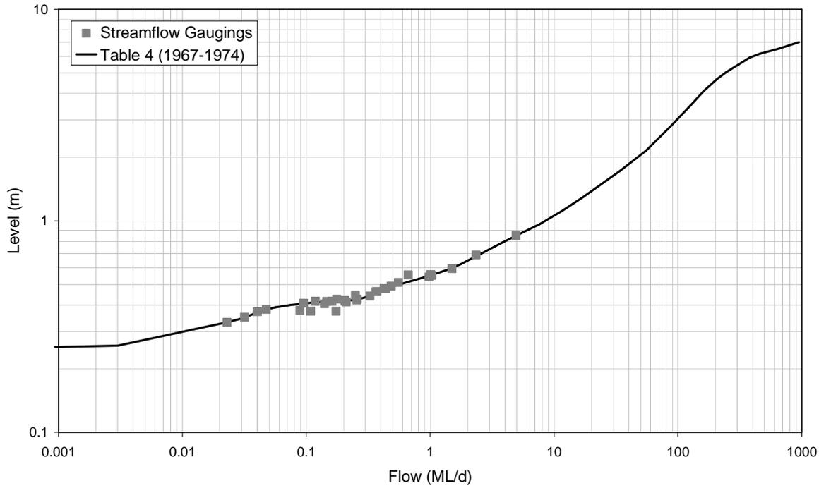
■ **Figure A-88: Rating Table 4 and Streamflow Gaugings for 8170084 (1967-1974)**
