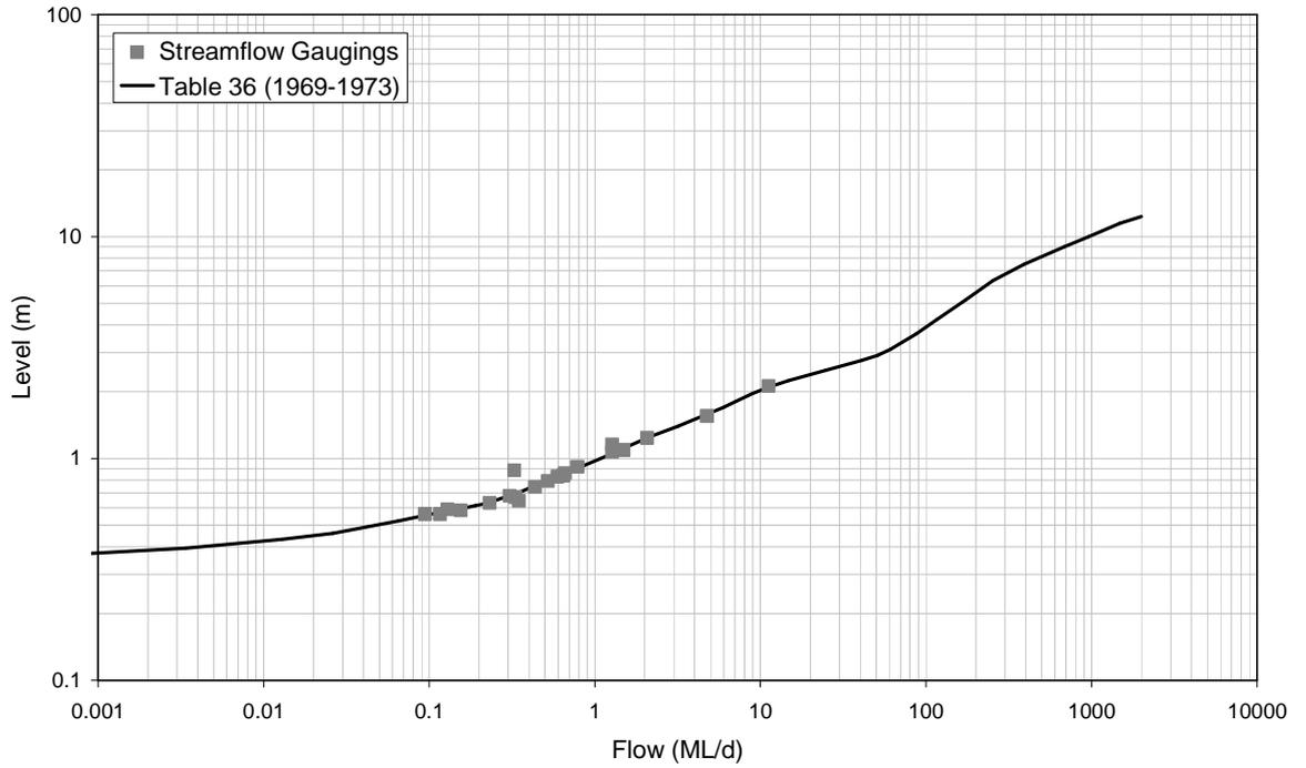
■ **Figure A-31: Rating Table 36 and Streamflow Gaugings for 8150180 (1969-1973)**
