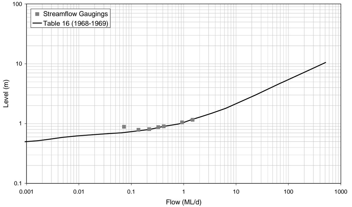
■ **Figure A-53: Rating Table 16 and Streamflow Gaugings for 8170005 (1968-1969)**
