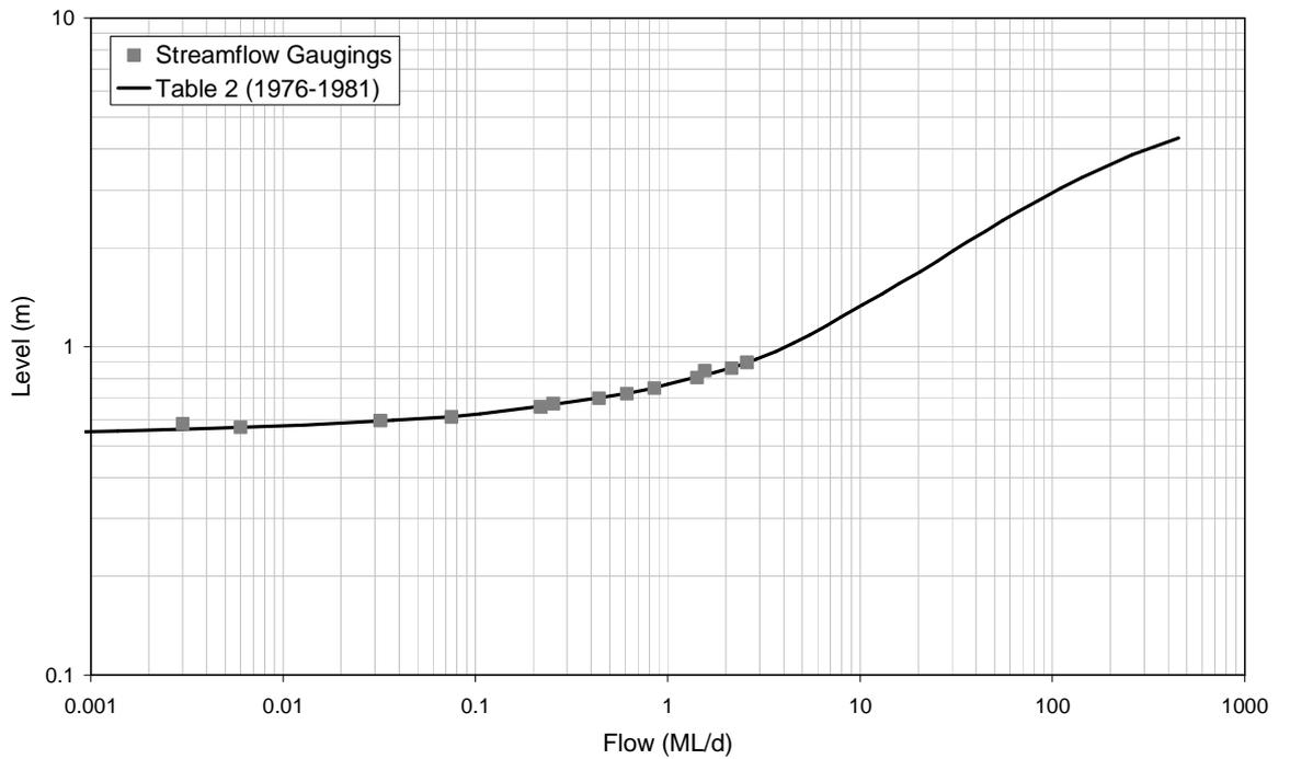
■ **Figure A-14: Rating Table 2 and Streamflow Gaugings for 8150097 (1976-1981)**
