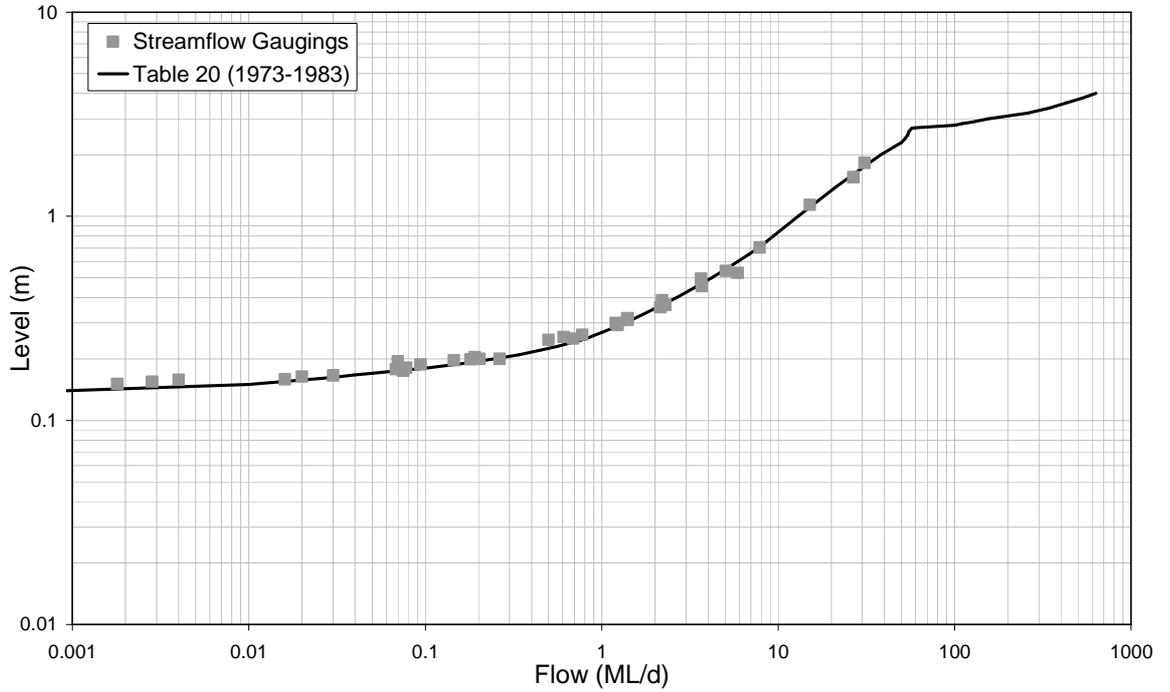
■ **Figure A-4: Rating Table 20 and Streamflow Gaugings for 8150018 (1973-1983)**
