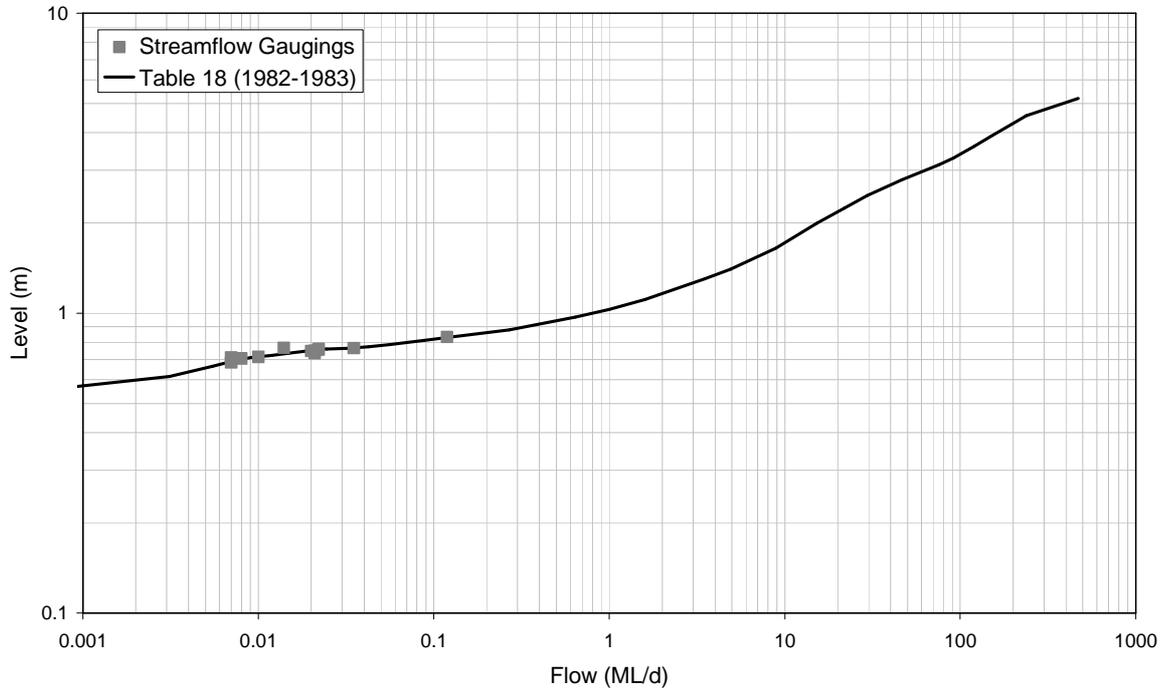
■ **Figure A-79: Rating Table 18 and Streamflow Gaugings for 8170066 (1982-1983)**
