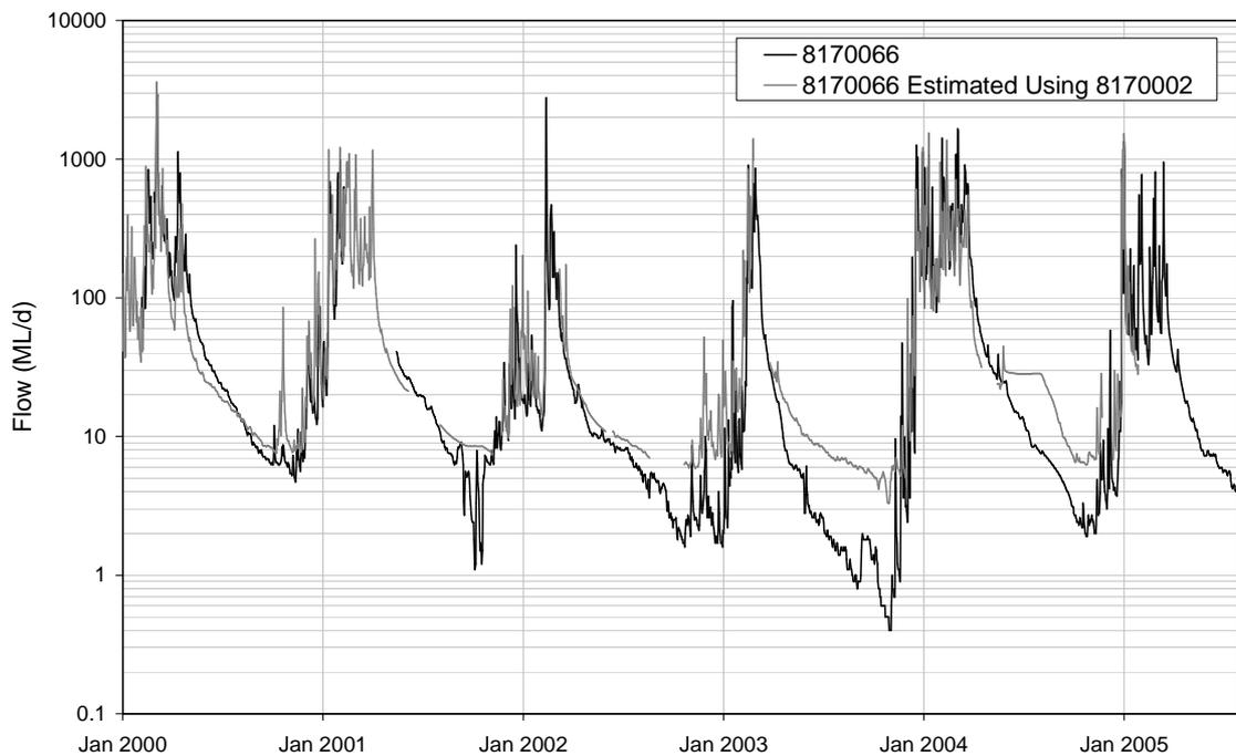
■ **Figure C-10: Comparison of Gauged and Estimated Flow at 8170066 (Regression 1)**
