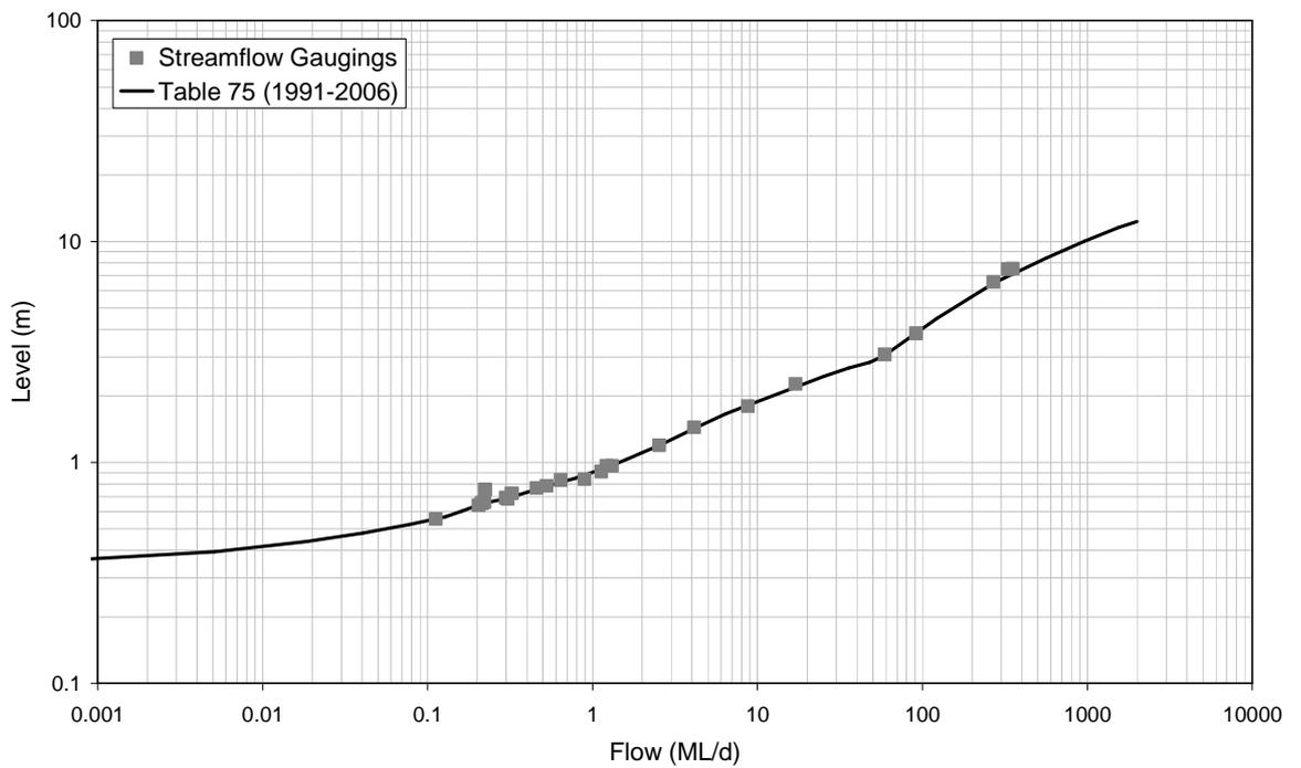
■ **Figure A-40: Rating Table 75 and Streamflow Gaugings for 8150180 (1991-2006)**
