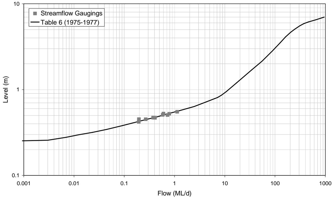
■ **Figure A-90: Rating Table 6 and Streamflow Gaugings for 8170084 (1975-1977)**
