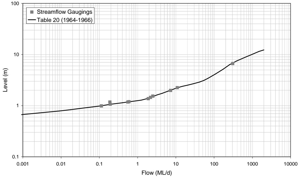
■ **Figure A-27: Rating Table 20 and Streamflow Gaugings for 8150180 (1964-1966)**
