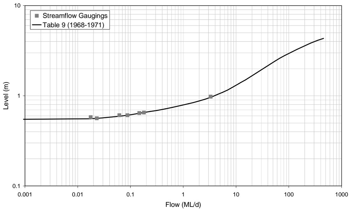
■ **Figure A-12: Rating Table 9 and Streamflow Gaugings for 8150097 (1968-1971)**
