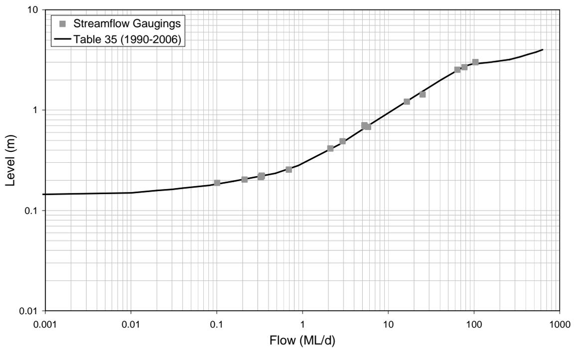
■ **Figure A-7: Rating Table 35 and Streamflow Gaugings for 8150018 (1990-2006)**
