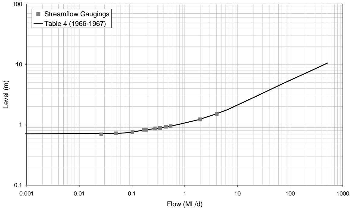
■ **Figure A-51: Rating Table 4 and Streamflow Gaugings for 8170005 (1966-1967)**
