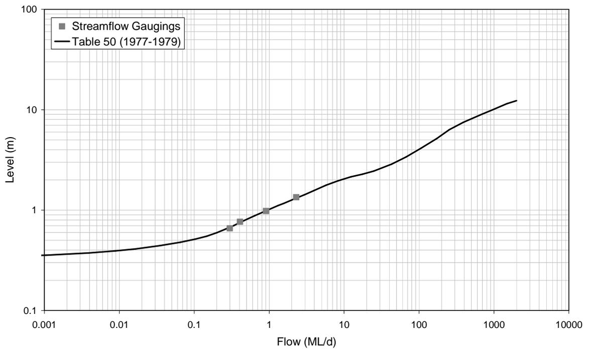
■ **Figure A-34: Rating Table 50 and Streamflow Gaugings for 8150180 (1977-1979)**
