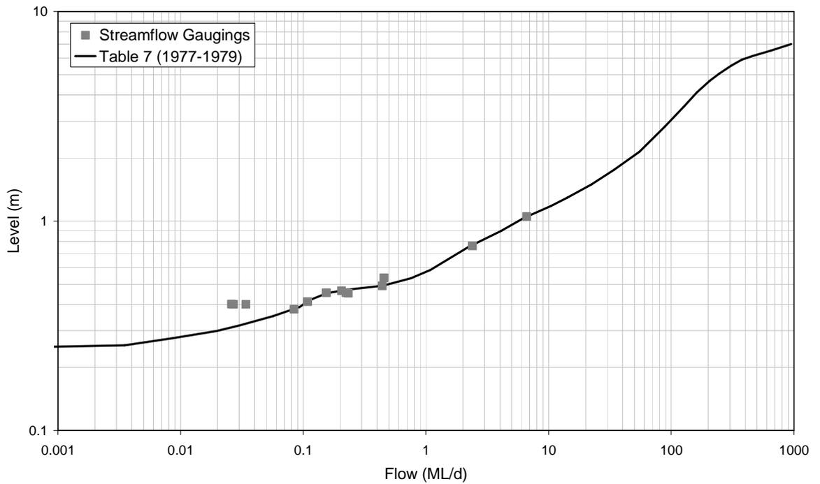
■ **Figure A-91: Rating Table 7 and Streamflow Gaugings for 8170084 (1977-1979)**
