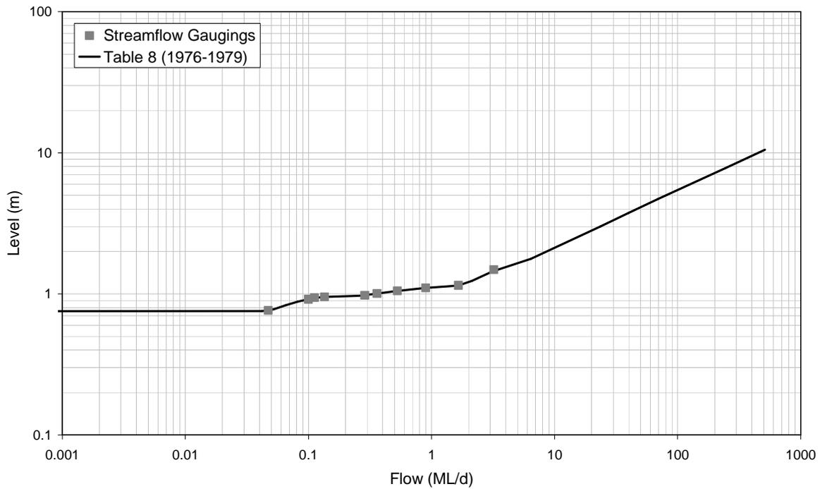
■ **Figure A-58: Rating Table 8 and Streamflow Gaugings for 8170005 (1976-1979)**
