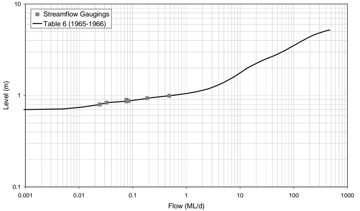
■ **Figure A-69: Rating Table 6 and Streamflow Gaugings for 8170066 (1965-1966)**
