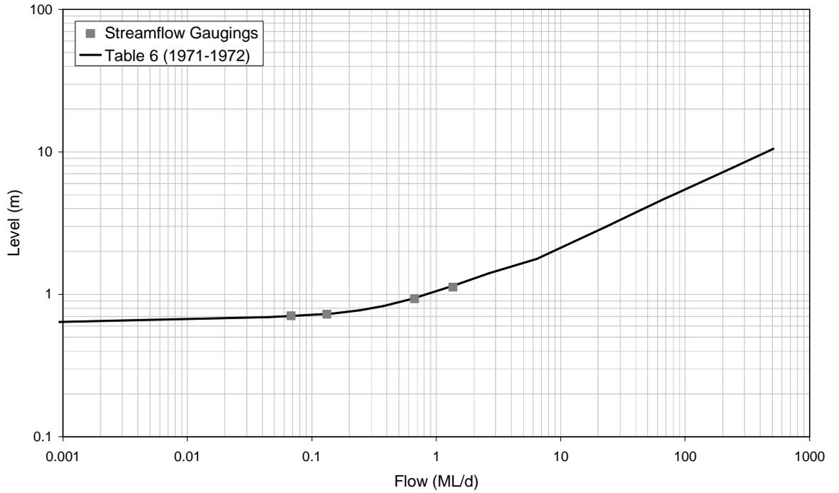
■ **Figure A-55: Rating Table 6 and Streamflow Gaugings for 8170005 (1971-1972)**
