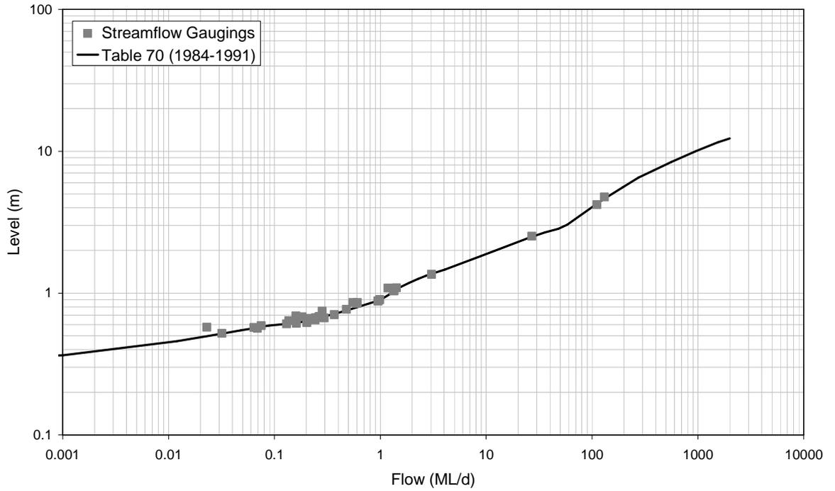
■ **Figure A-39: Rating Table 70 and Streamflow Gaugings for 8150180 (1984-1991)**
