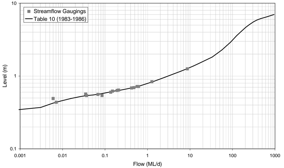
■ **Figure A-94: Rating Table 10 and Streamflow Gaugings for 8170084 (1983-1986)**
