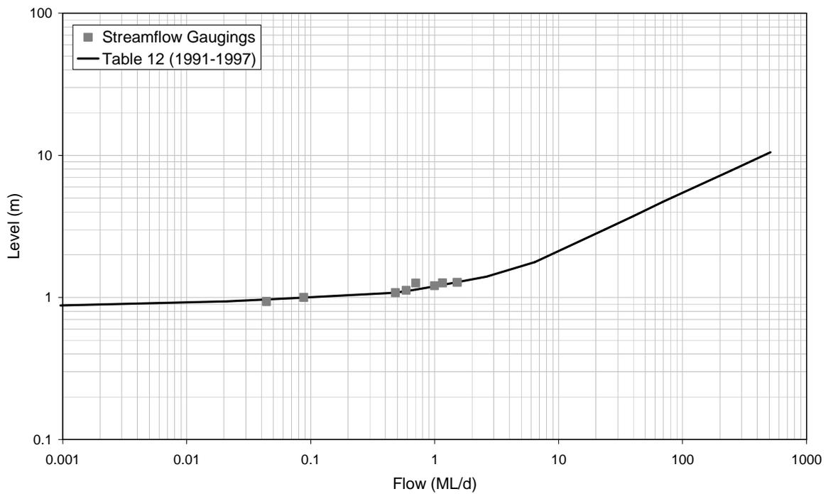
■ **Figure A-62: Rating Table 12 and Streamflow Gaugings for 8170005 (1991-1997)**
