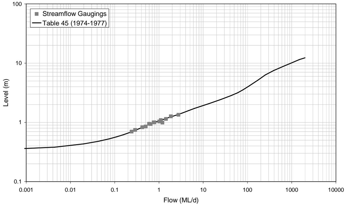
■ **Figure A-33: Rating Table 45 and Streamflow Gaugings for 8150180 (1974-1977)**
