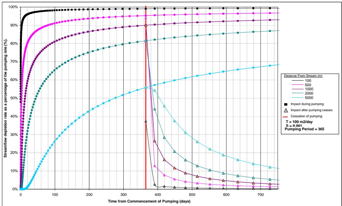
■ Figure 3-2 Examples of Estimated Stream Flow Depletion at Differing Distances from the River for Different Aquifer Hydraulic Parameters
