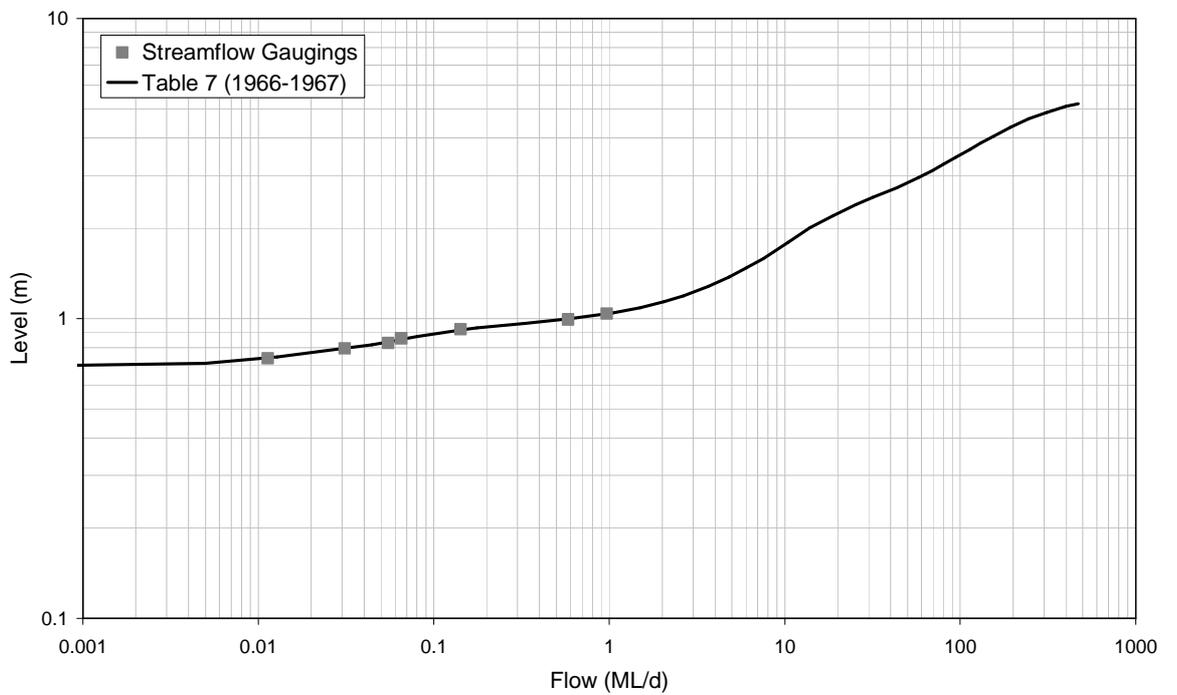
■ **Figure A-70: Rating Table 7 and Streamflow Gaugings for 8170066 (1966-1967)**
