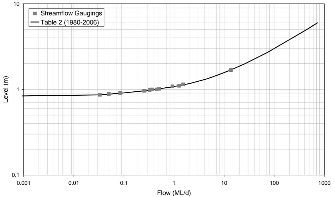
■ **Figure A-66: Rating Table 1 and Streamflow Gaugings for 8170062 (1980-2006)**
