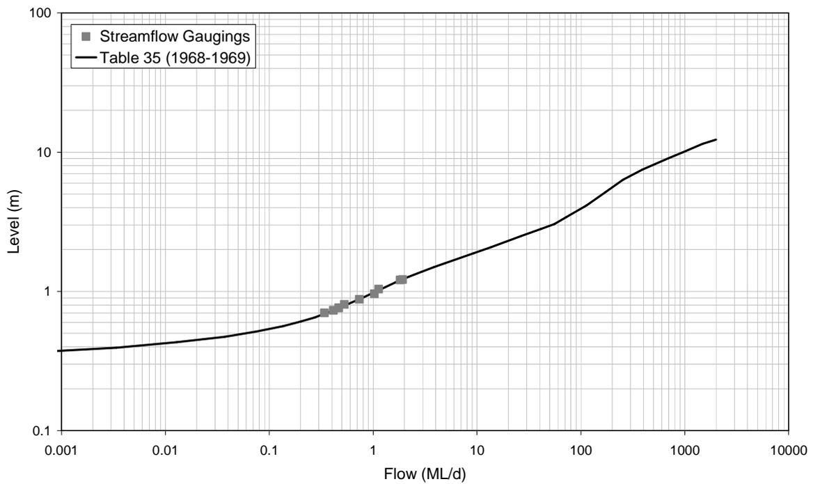
■ **Figure A-30: Rating Table 35 and Streamflow Gaugings for 8150180 (1968-1969)**
