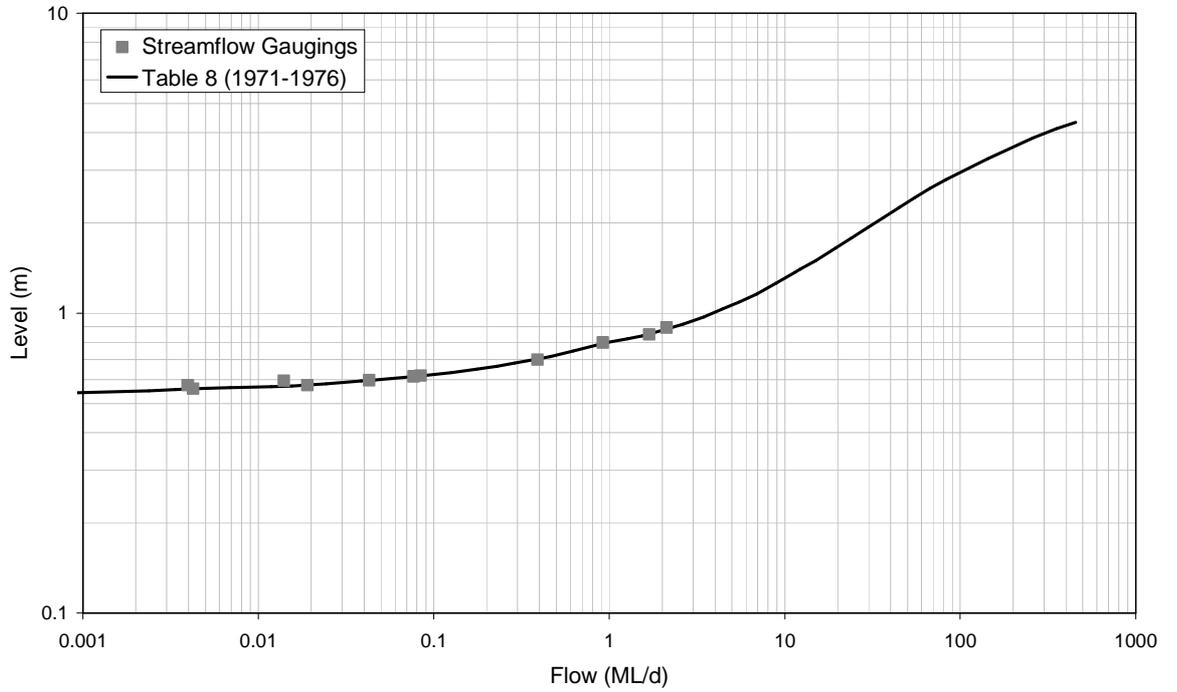
■ **Figure A-13: Rating Table 8 and Streamflow Gaugings for 8150097 (1971-1976)**
