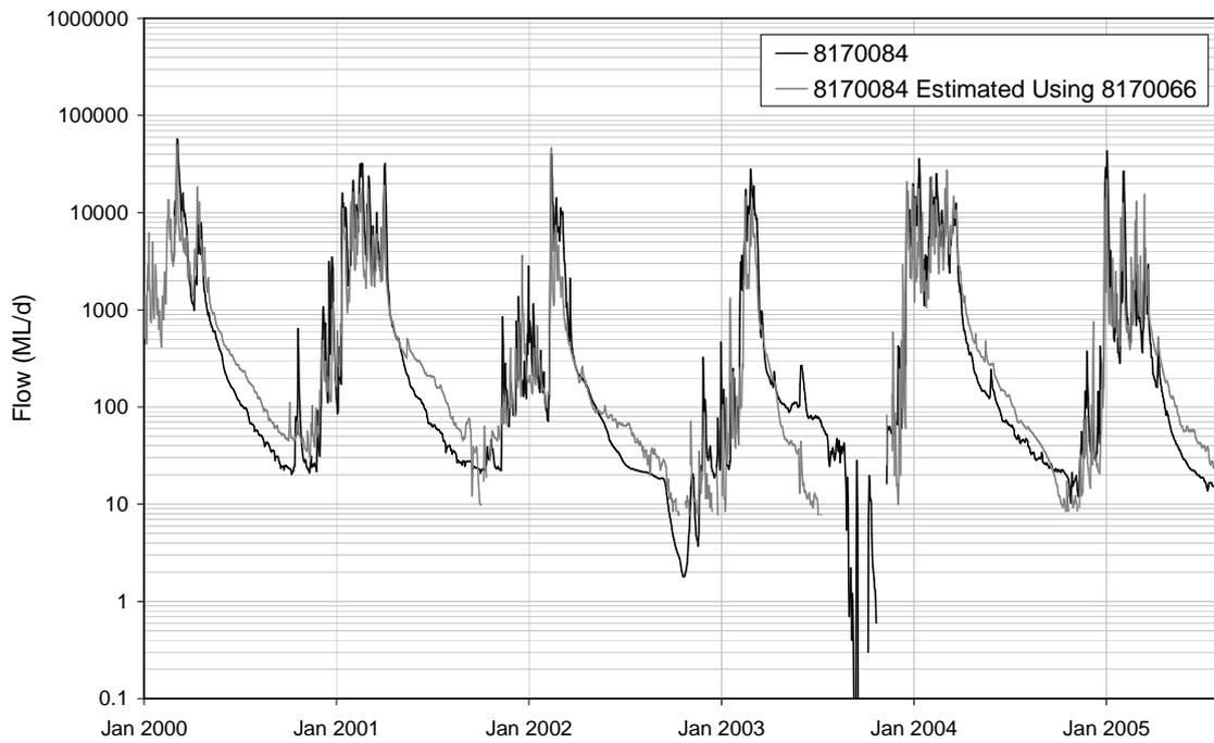
■ **Figure C-12: Comparison of Gauged and Estimated Flow at 8170084**
