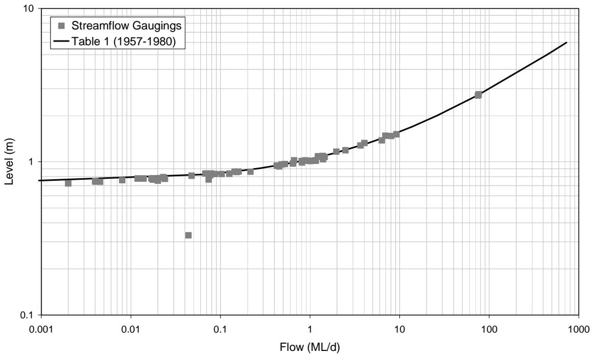
■ **Figure A-65: Rating Table 1 and Streamflow Gaugings for 8170062 (1957-1980)**
