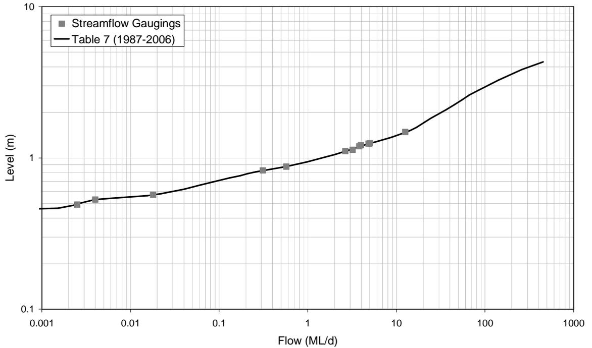
■ **Figure A-19: Rating Table 7 and Streamflow Gaugings for 8150097 (1987-2006)**
