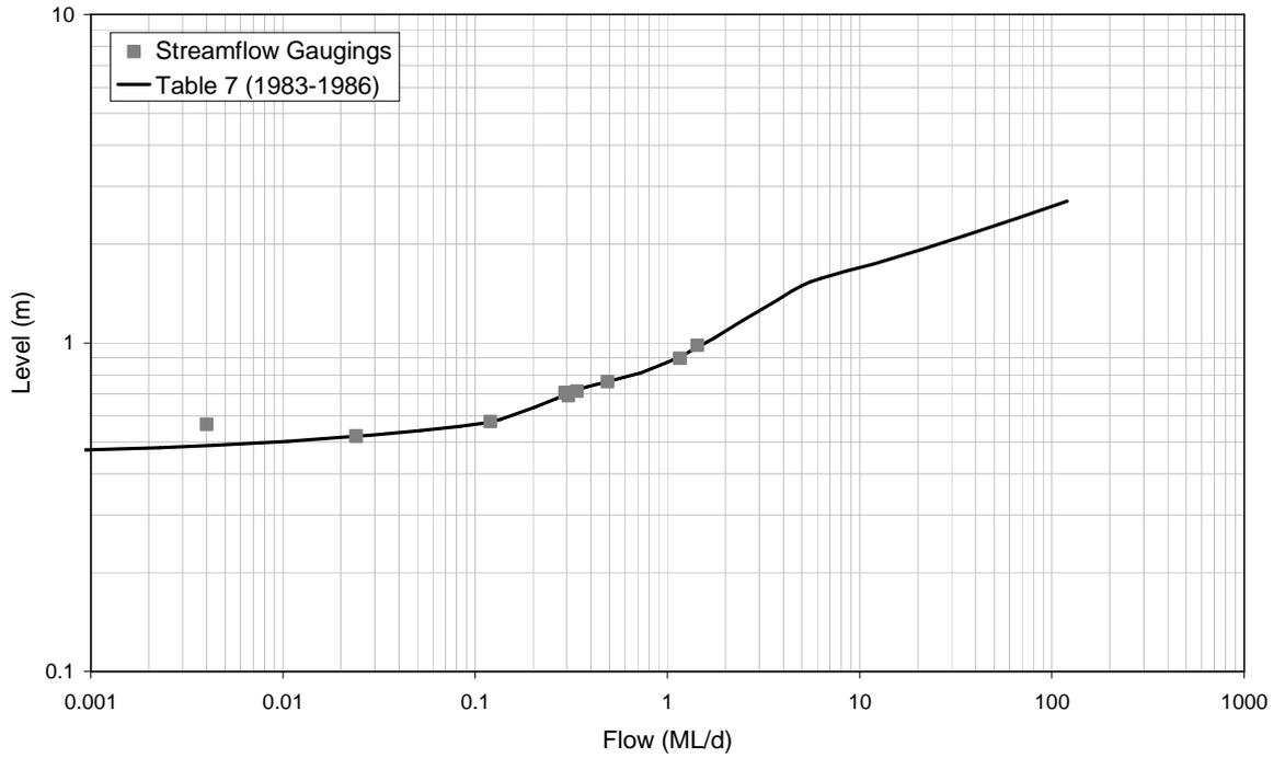
■ **Figure A-103: Rating Table 7 and Streamflow Gaugings for 8170085 (1983-1986)**
