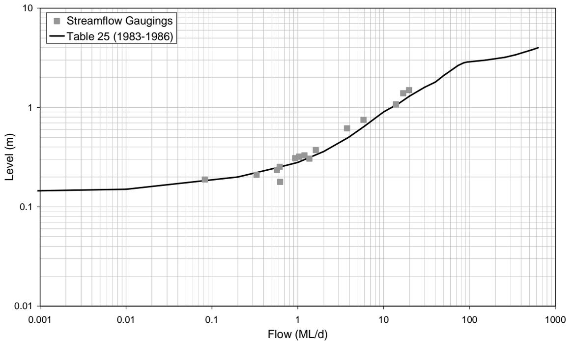
■ **Figure A-5: Rating Table 25 and Streamflow Gaugings for 8150018 (1983-1986)**
