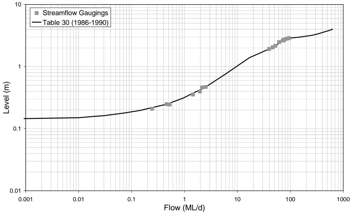
■ **Figure A-6: Rating Table 30 and Streamflow Gaugings for 8150018 (1986-1990)**
