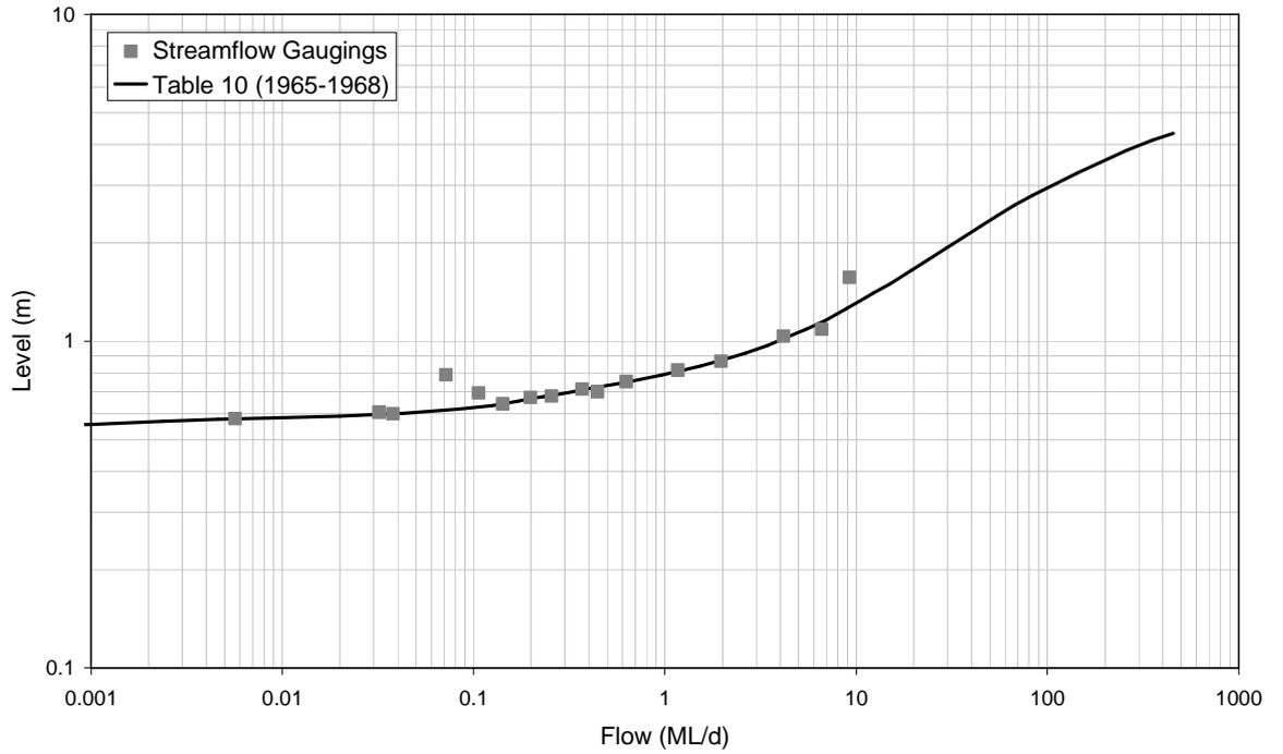
■ **Figure A-11: Rating Table 10 and Streamflow Gaugings for 8150097 (1965-1968)**
