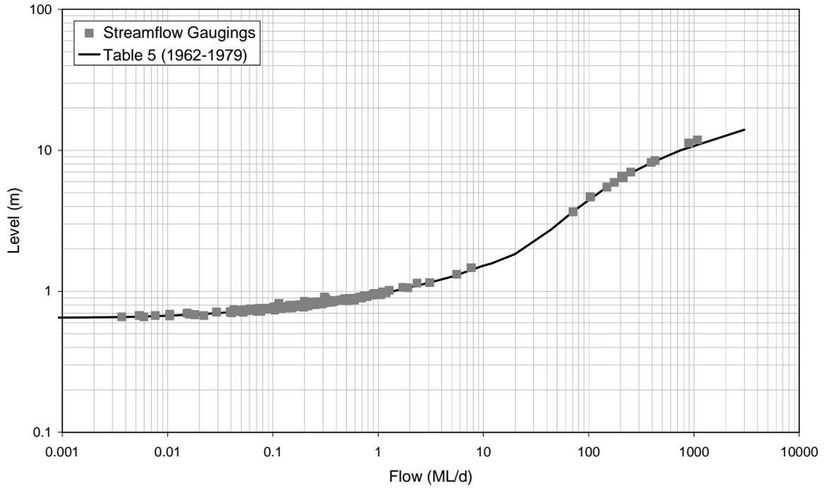
■ **Figure A-42: Rating Table 5 and Streamflow Gaugings for 8170002 (1962-1979)**
