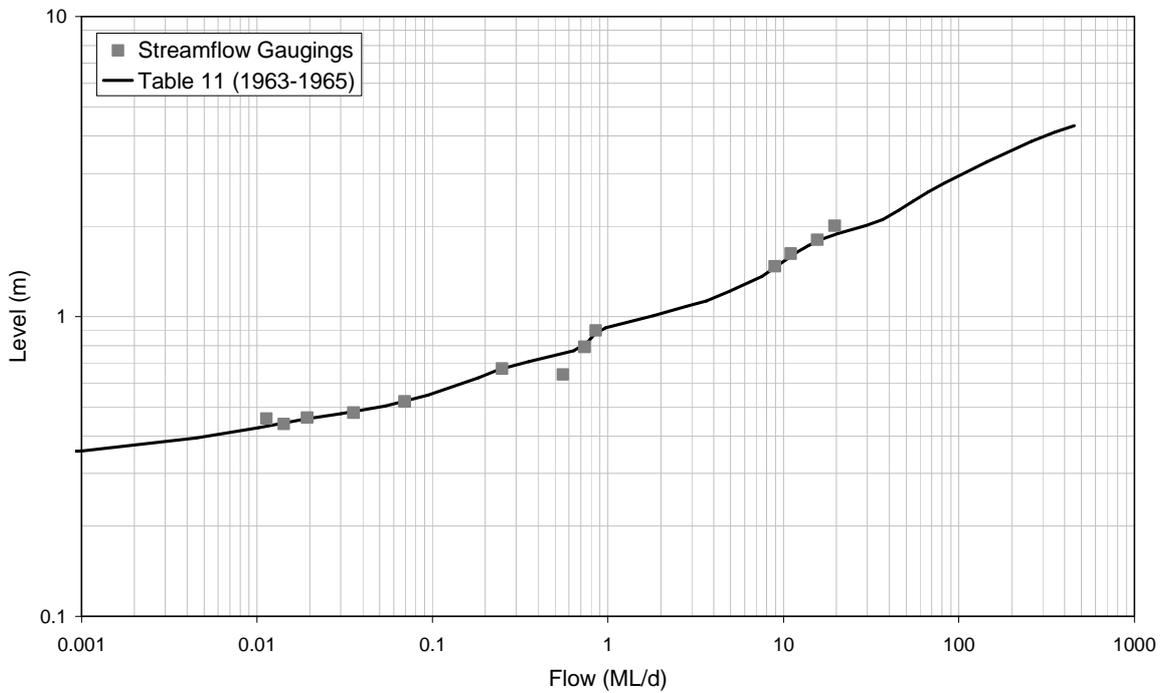
■ **Figure A-10: Rating Table 11 and Streamflow Gaugings for 8150097 (1963-1965)**
