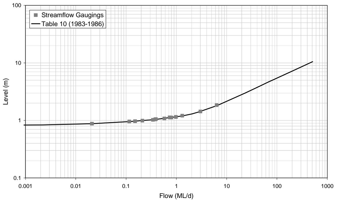
■ **Figure A-60: Rating Table 10 and Streamflow Gaugings for 8170005 (1983-1986)**
