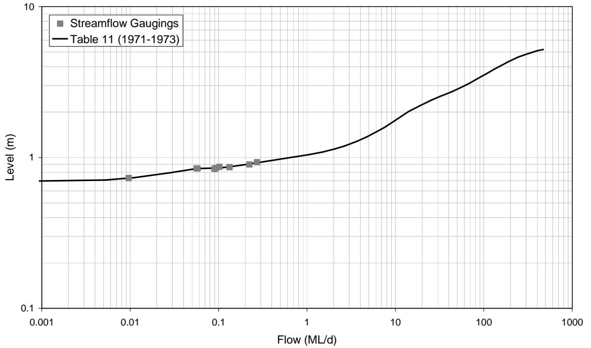
■ **Figure A-73: Rating Table 11 and Streamflow Gaugings for 8170066 (1971-1973)**
