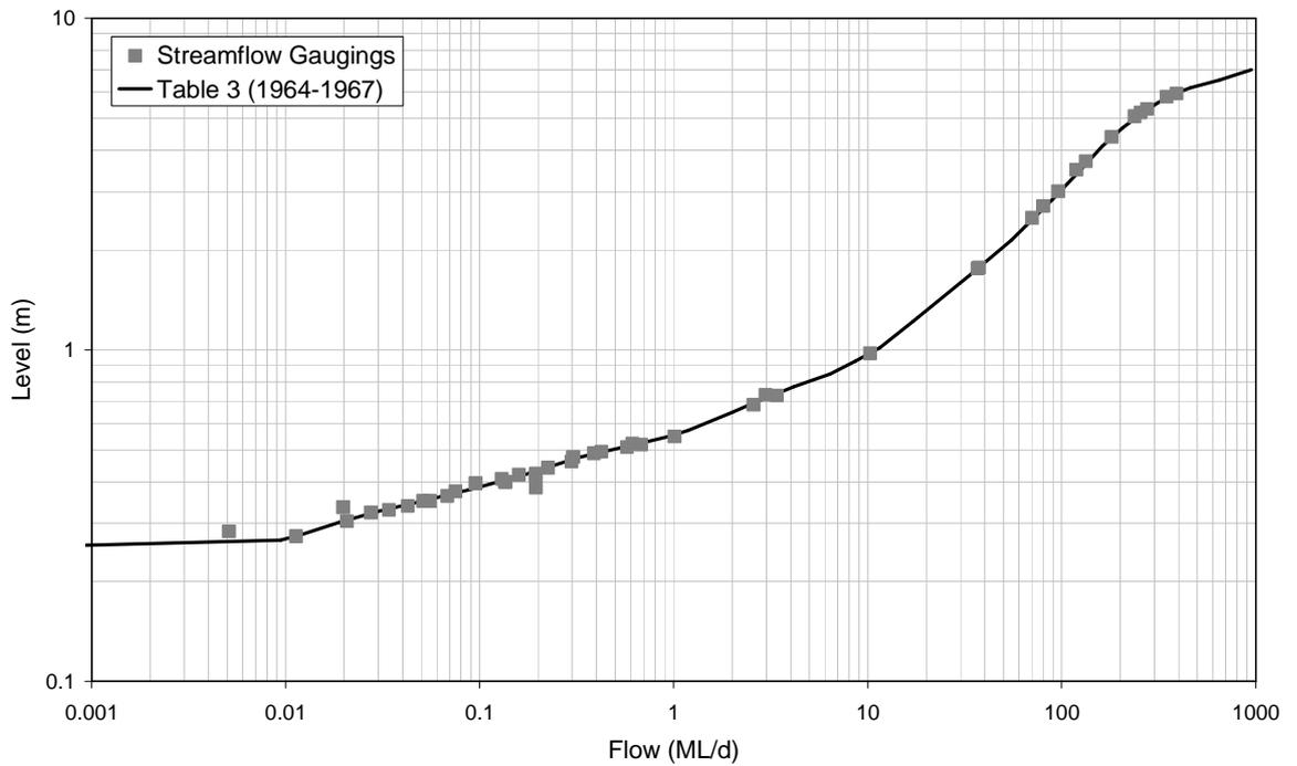
■ **Figure A-87: Rating Table 3 and Streamflow Gaugings for 8170084 (1964-1967)**
