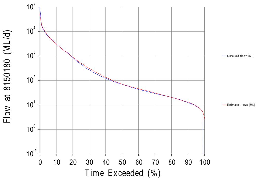
■ **Figure D-4 Daily SIMHYD Flow-Duration Curve - Finniss River at Gitchams (G8150180)**
