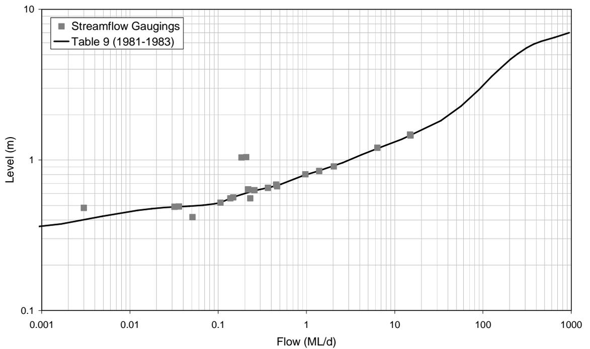
■ **Figure A-93: Rating Table 9 and Streamflow Gaugings for 8170084 (1981-1983)**
