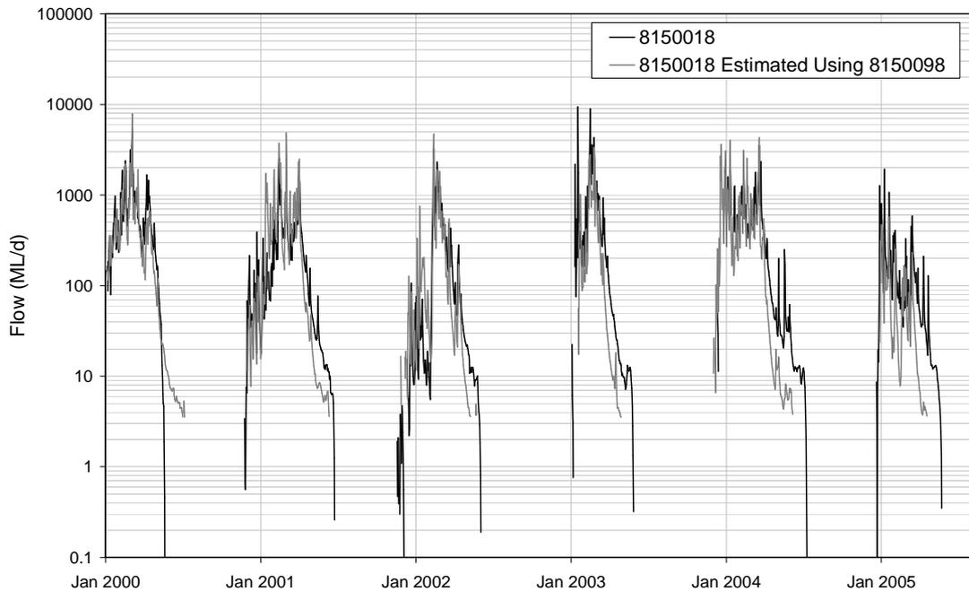
■ **Figure C-2: Comparison of Gauged and Estimated Flow at 8150018**
