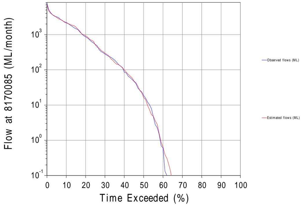
■ **Figure D-14 Monthly SIMHYD Flow-Duration Curve - Acacia Creek at Stuart Highway (G8170085)**
