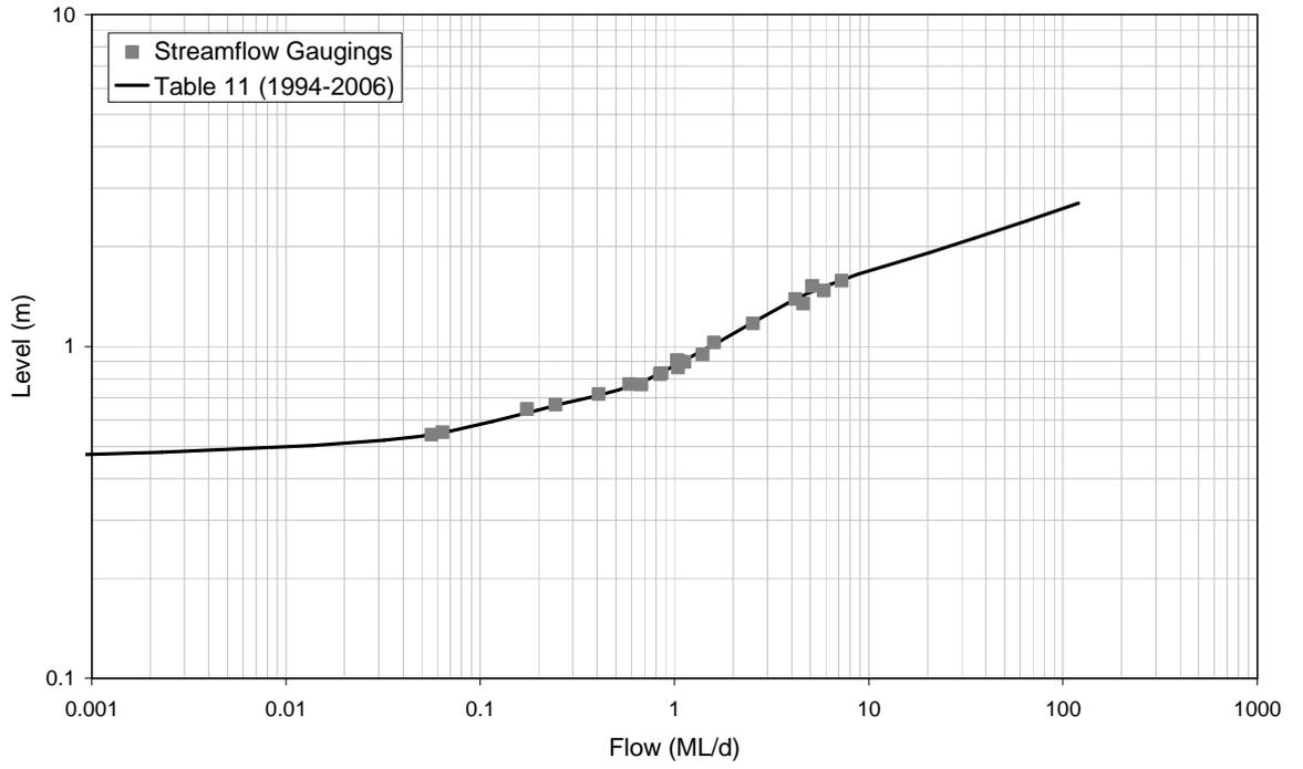
■ **Figure A-107: Rating Table 11 and Streamflow Gaugings for 8170085 (1994-2006)**
