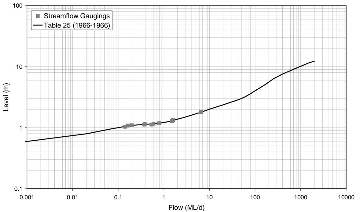
■ **Figure A-28: Rating Table 25 and Streamflow Gaugings for 8150180 (1966)**
