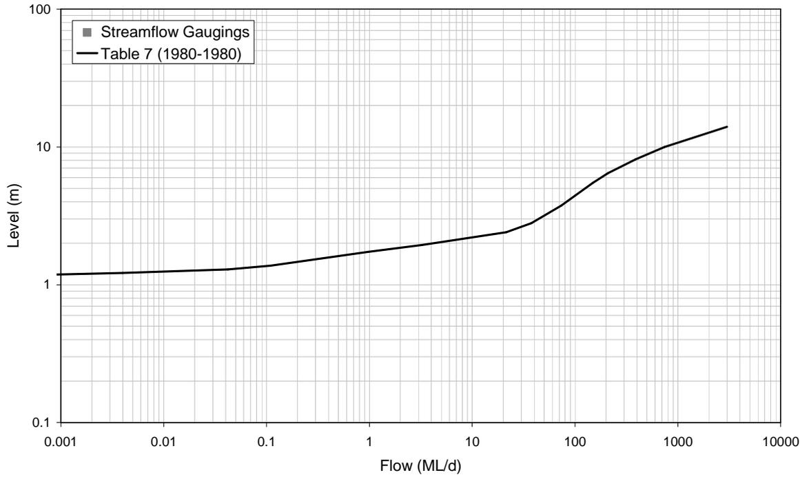
■ **Figure A-46: Rating Table 7 and Streamflow Gaugings for 8170002 (1980)**
