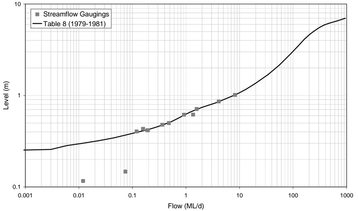
■ **Figure A-92: Rating Table 8 and Streamflow Gaugings for 8170084 (1979-1981)**
