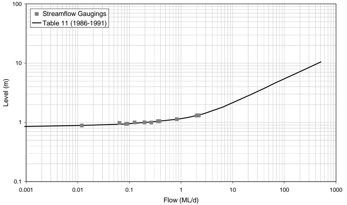
■ **Figure A-61: Rating Table 11 and Streamflow Gaugings for 8170005 (1986-1991)**
