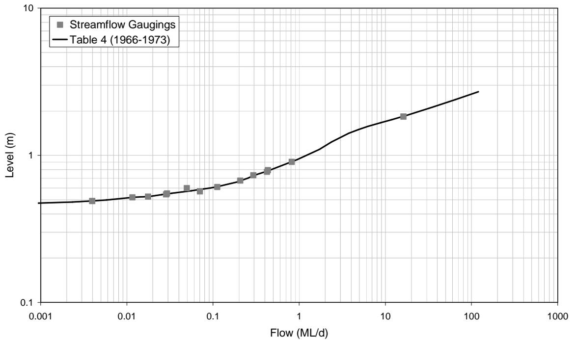
■ **Figure A-100: Rating Table 4 and Streamflow Gaugings for 8170085 (1966-1973)**
