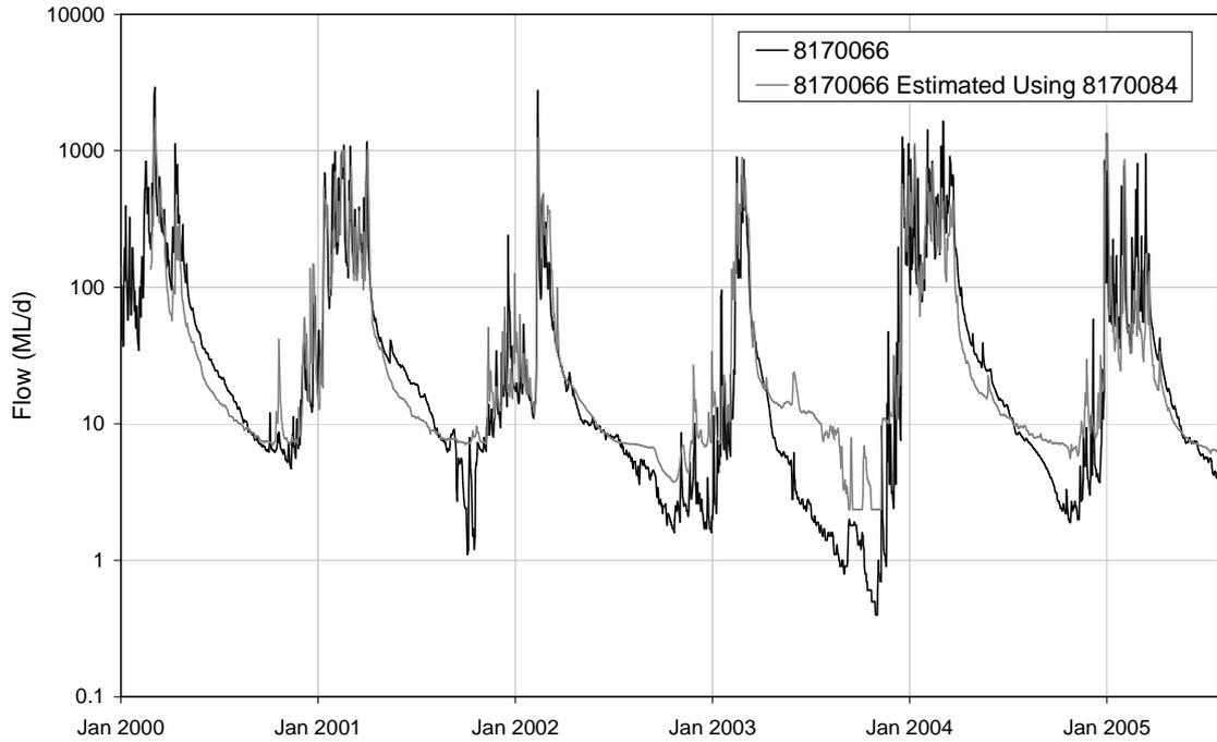
■ **Figure C-11: Comparison of Gauged and Estimated Flow at 8170066 (Regression 2)**
