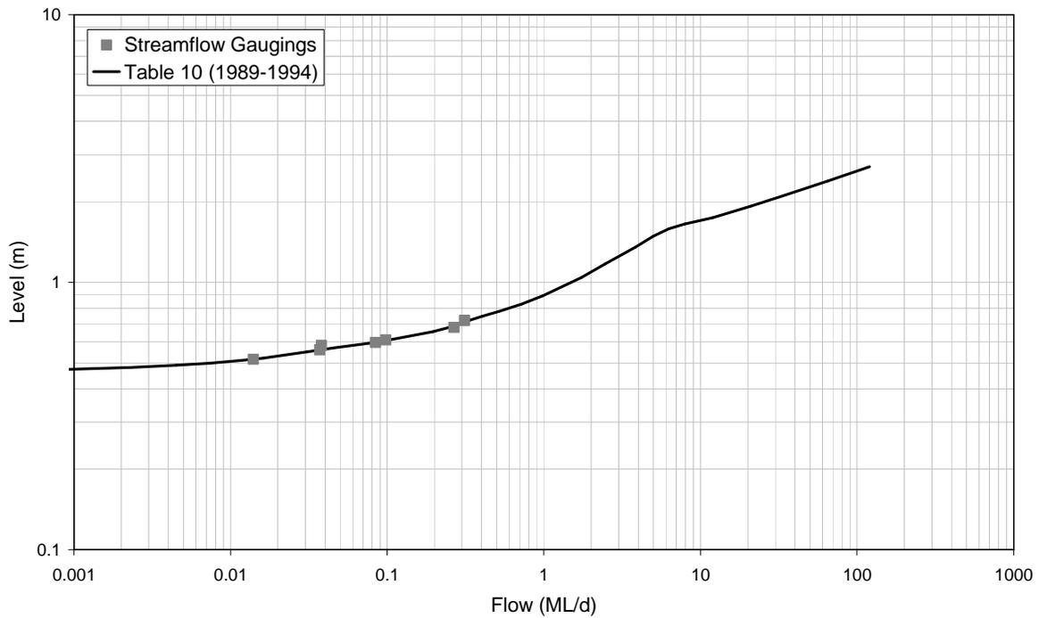
■ **Figure A-106: Rating Table 10 and Streamflow Gaugings for 8170085 (1989-1994)**
