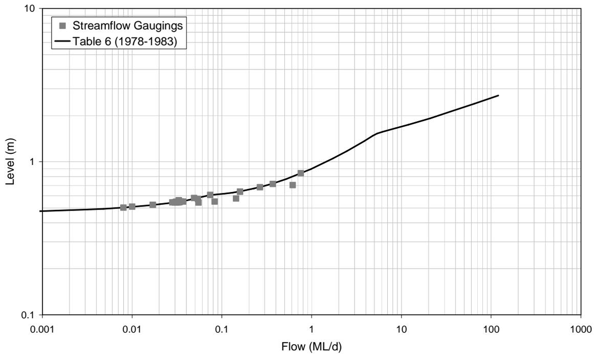
■ **Figure A-102: Rating Table 6 and Streamflow Gaugings for 8170085 (1978-1983)**
