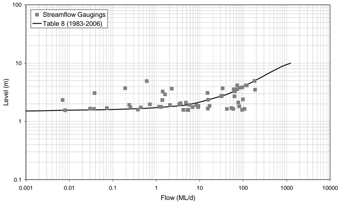
■ **Figure A-25: Rating Table 8 and Streamflow Gaugings for 8150098 (1981-2006)**
