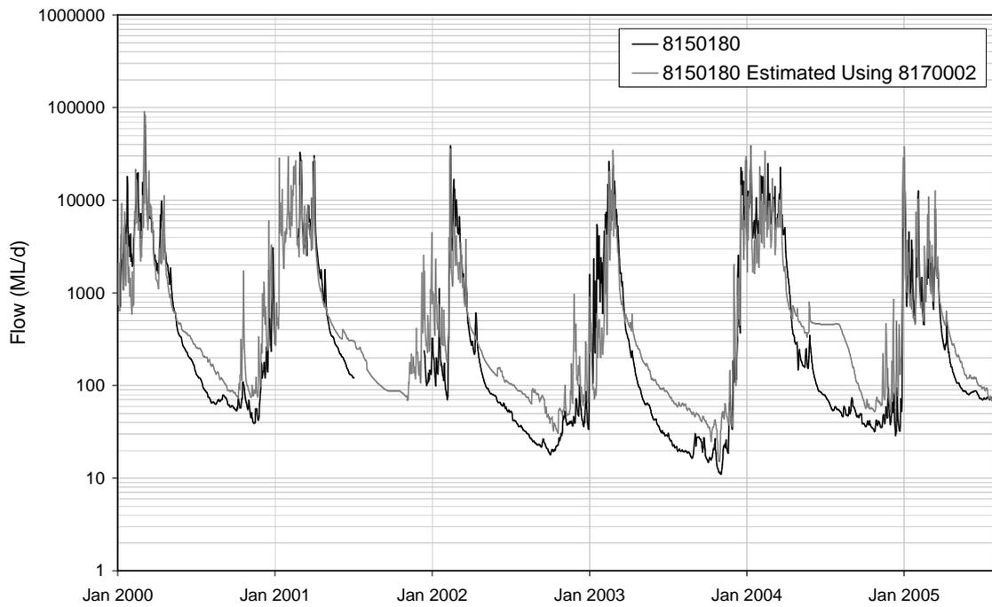
■ **Figure C-6: Comparison of Gauged and Estimated Flow at 8150180**
