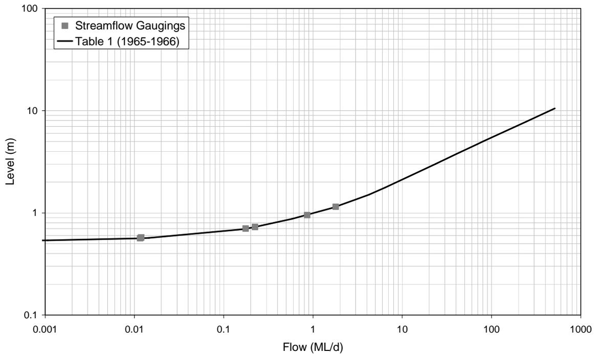
■ **Figure A-50: Rating Table 1 and Streamflow Gaugings for 8170005 (1965-1966)**
