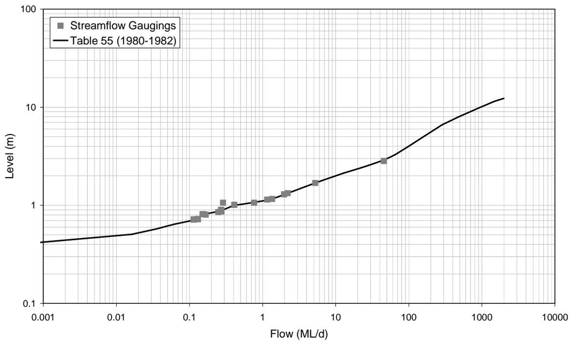
■ **Figure A-36: Rating Table 55 and Streamflow Gaugings for 8150180 (1980-1982)**
