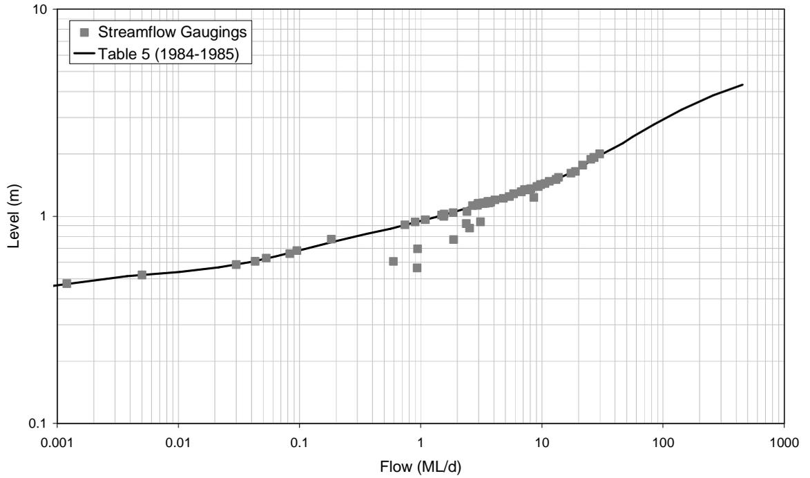
■ **Figure A-17: Rating Table 5 and Streamflow Gaugings for 8150097 (1984-1985)**
