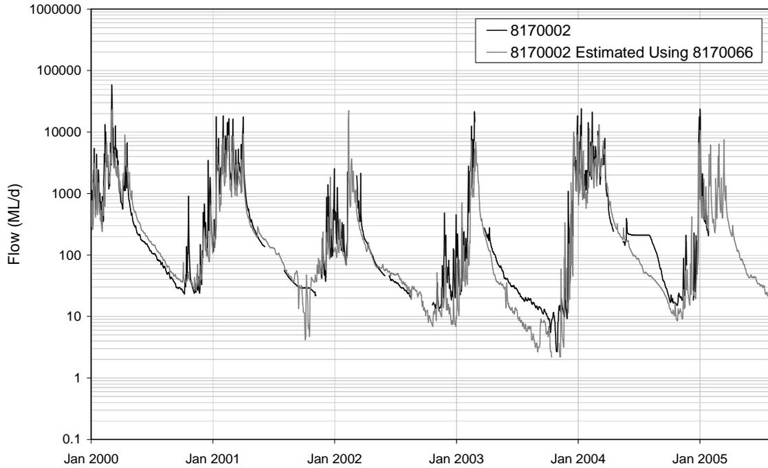
■ **Figure C-7: Comparison of Gauged and Estimated Flow at 8170002**
