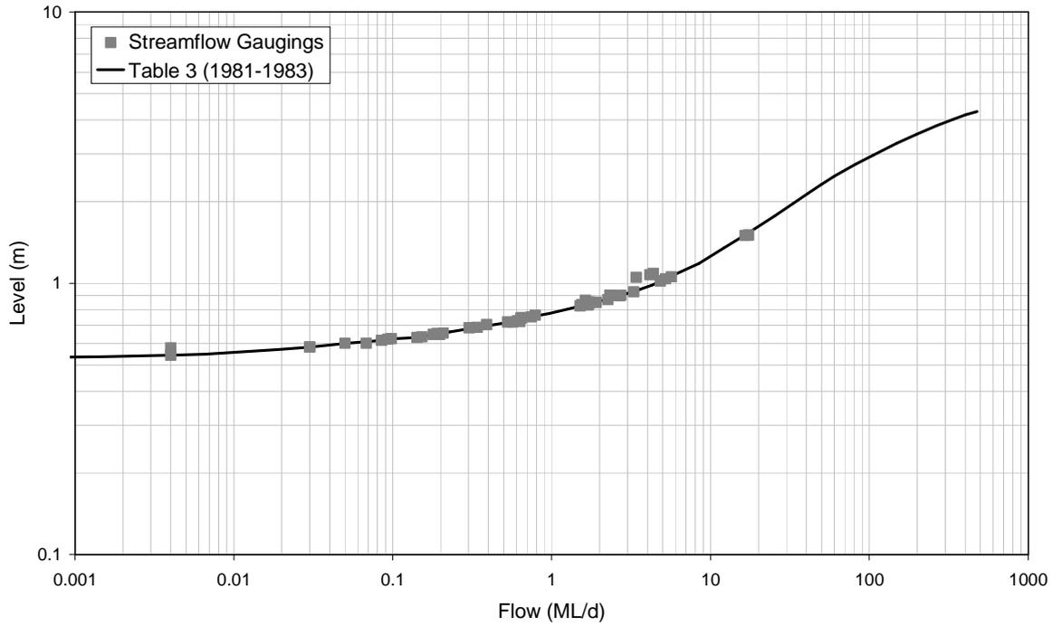
■ **Figure A-15: Rating Table 3 and Streamflow Gaugings for 8150097 (1981-1983)**
