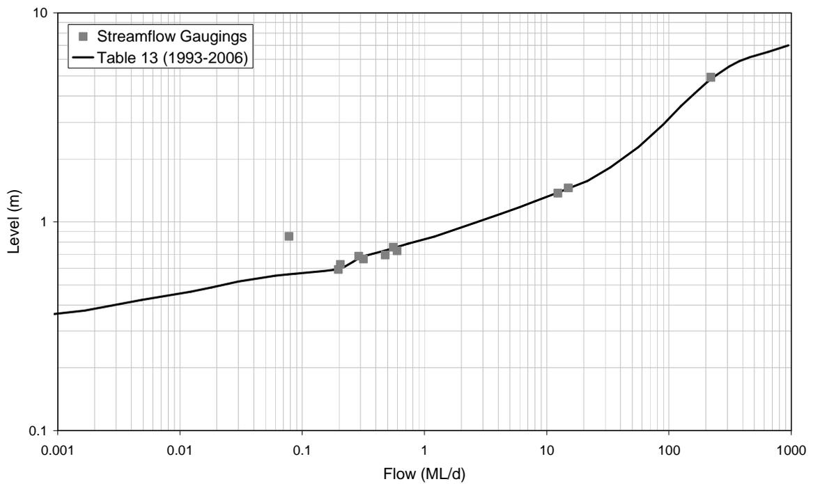
■ **Figure A-97: Rating Table 13 and Streamflow Gaugings for 8170084 (1993-2006)**
