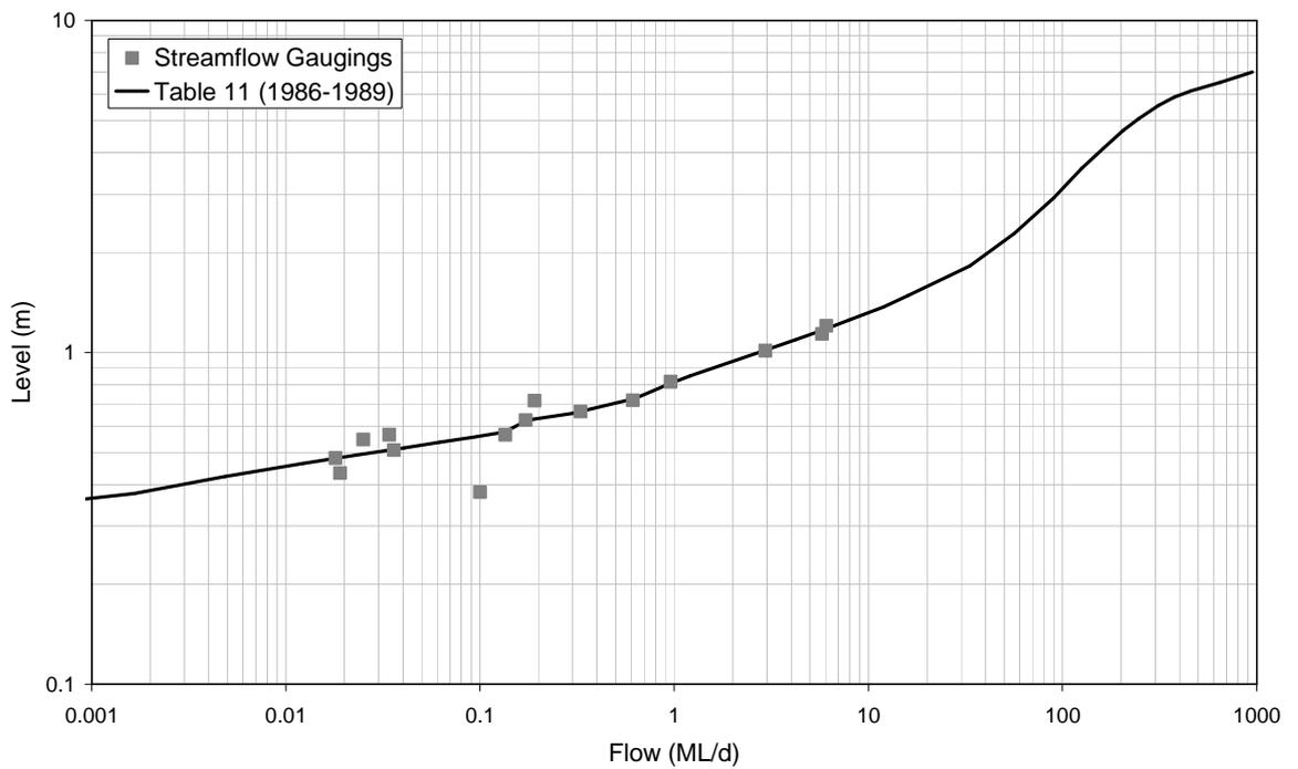
■ **Figure A-95: Rating Table 11 and Streamflow Gaugings for 8170084 (1986-1989)**
