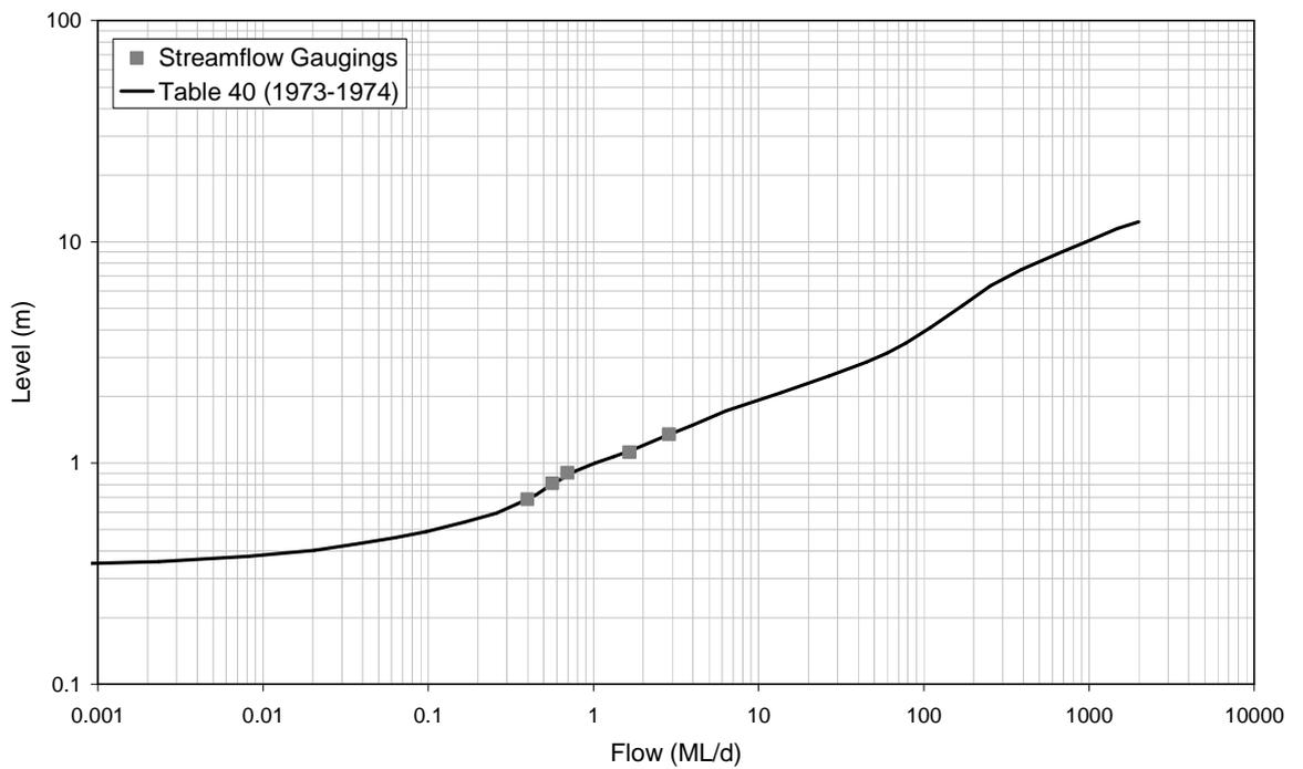
■ **Figure A-32: Rating Table 40 and Streamflow Gaugings for 8150180 (1973-1974)**
