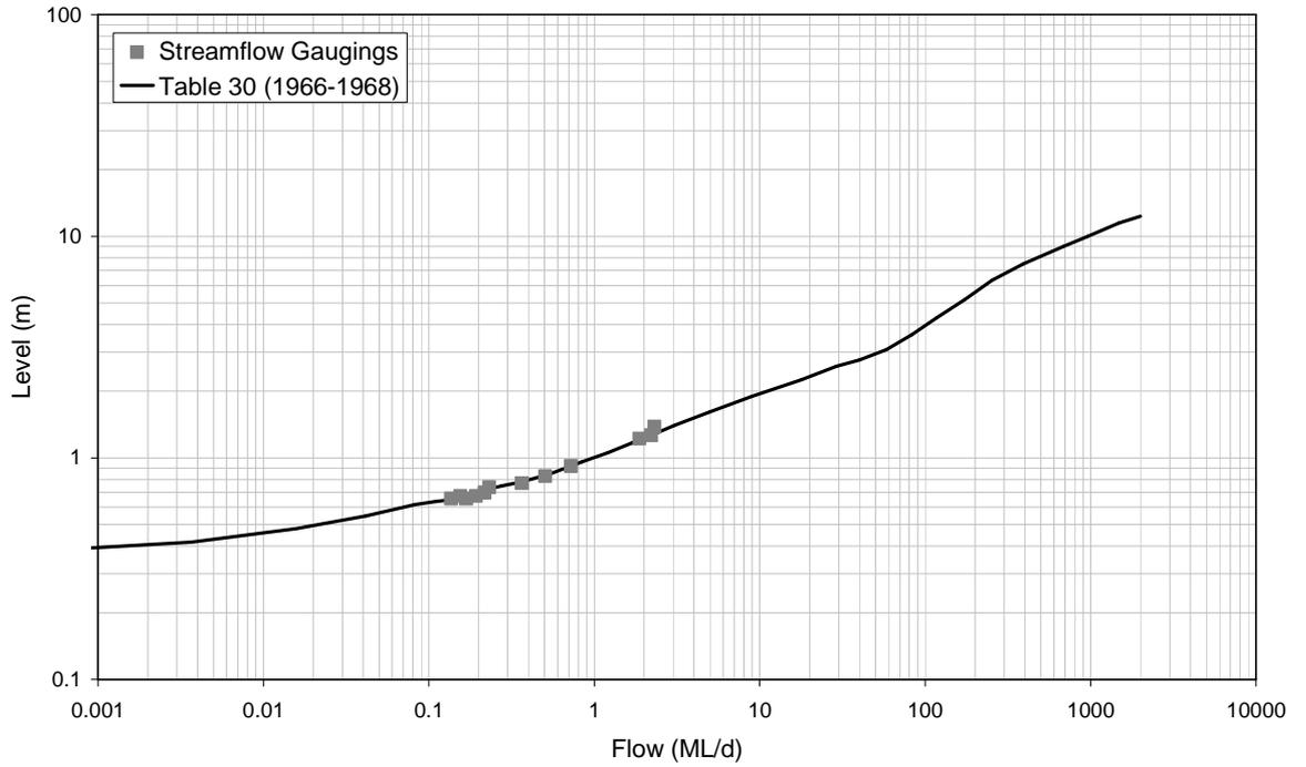
■ **Figure A-29: Rating Table 30 and Streamflow Gaugings for 8150180 (1966-1968)**
