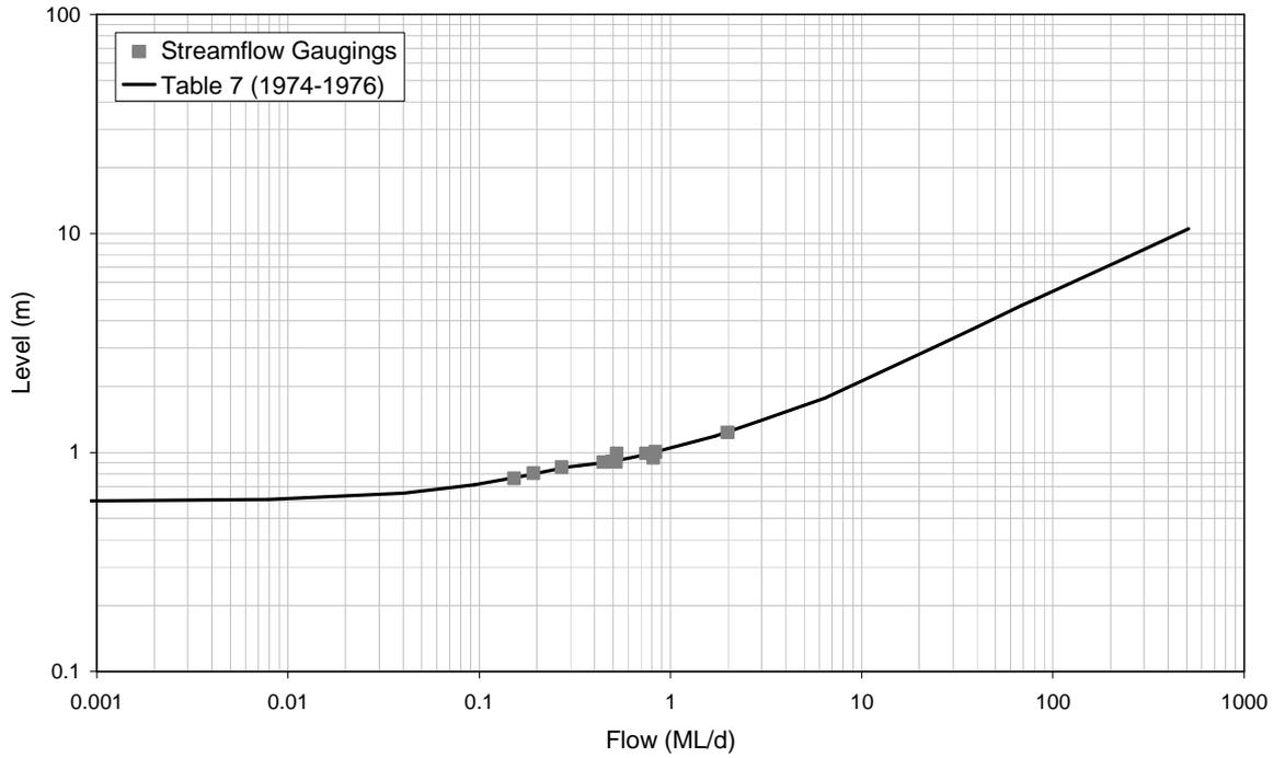
■ **Figure A-57: Rating Table 7 and Streamflow Gaugings for 8170005 (1974-1976)**
