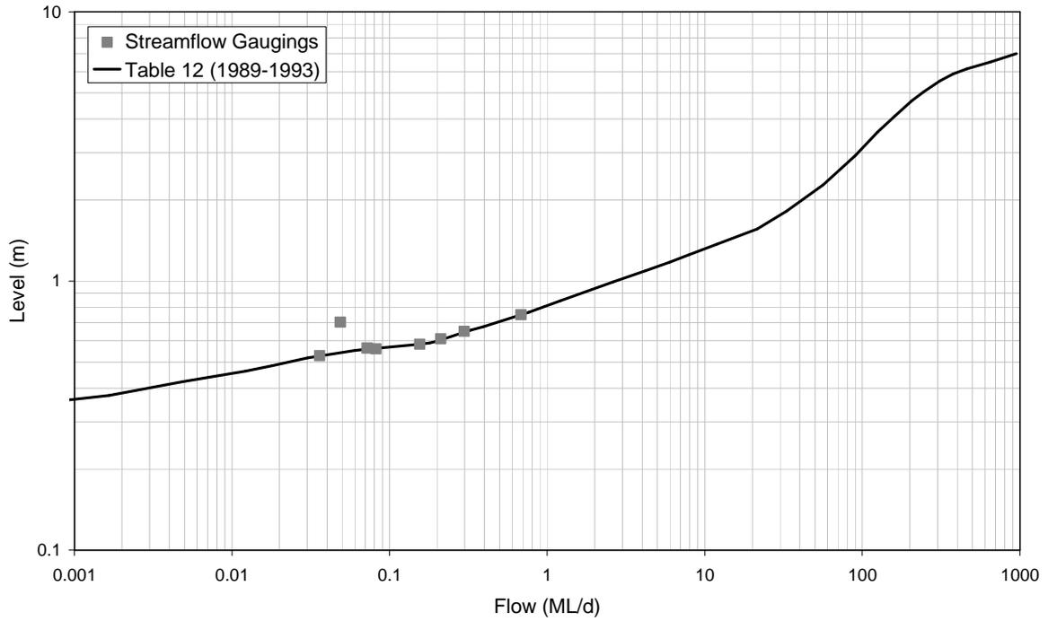
■ **Figure A-96: Rating Table 12 and Streamflow Gaugings for 8170084 (1989-1993)**
