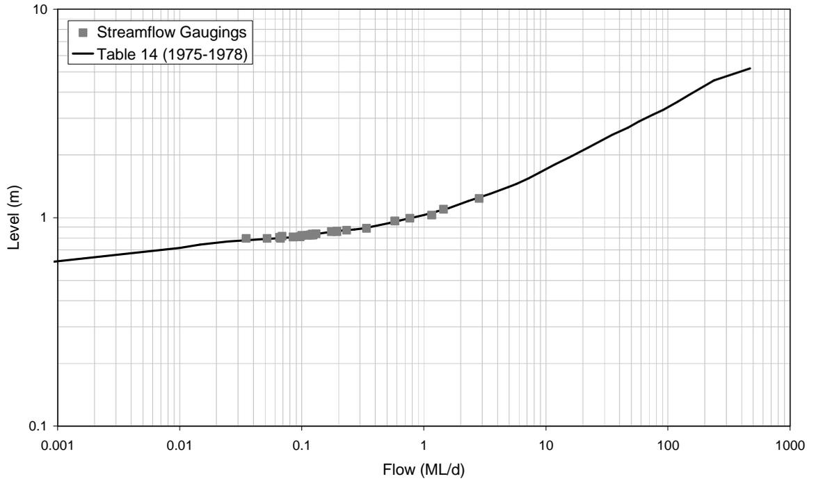
■ **Figure A-75: Rating Table 14 and Streamflow Gaugings for 8170066 (1975-1978)**
