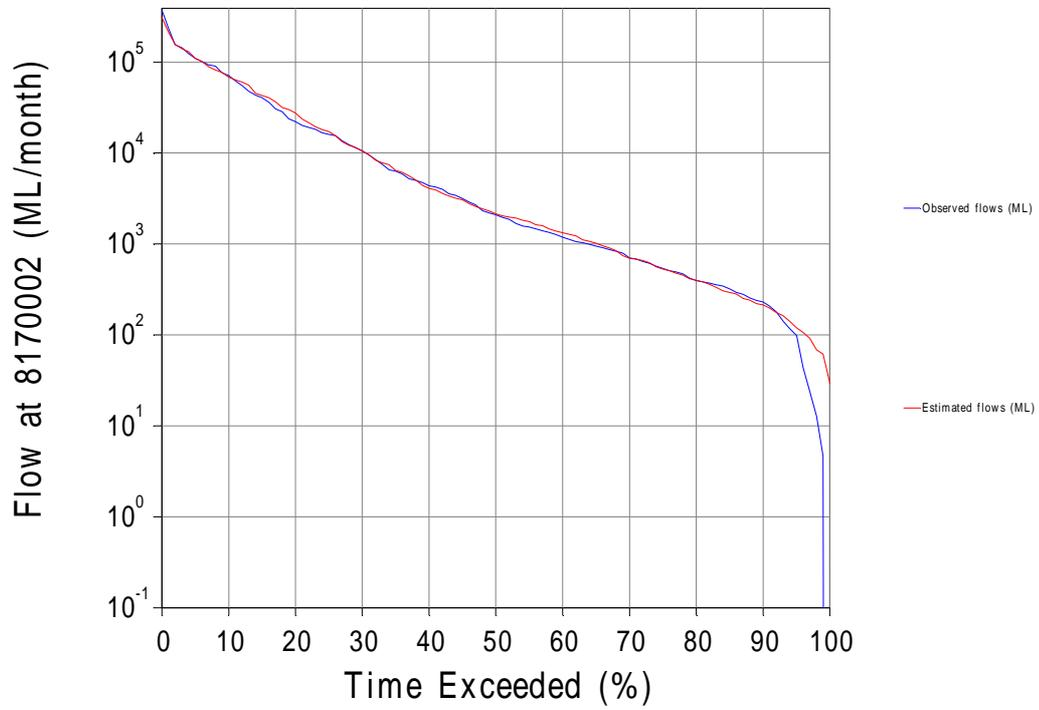
■ **Figure D-12 Monthly SIMHYD Flow-Duration Curve - Adelaide River at Railway Bridge (G8170002)**
