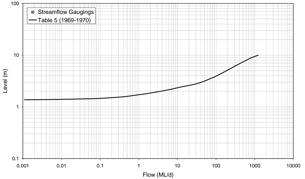
■ **Figure A-22: Rating Table 5 and Streamflow Gaugings for 8150098 (1969-1970)**
