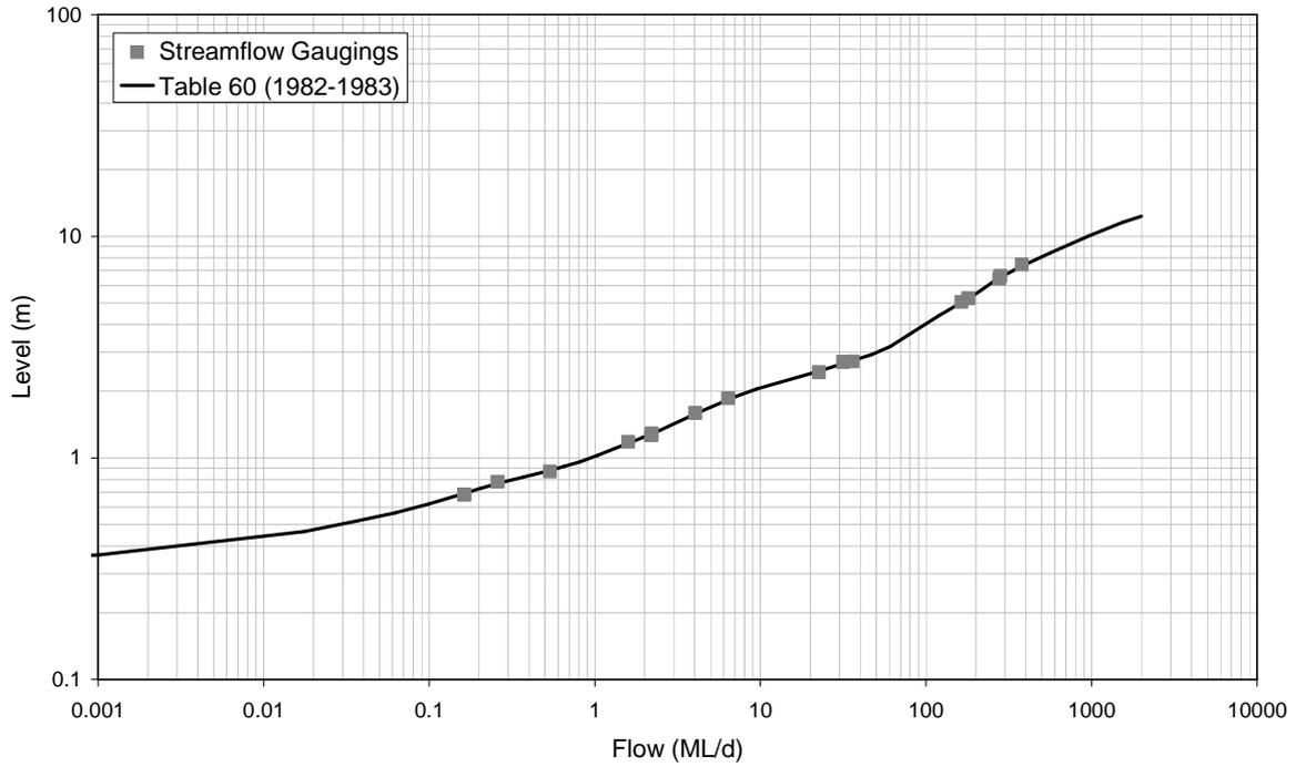
■ **Figure A-37: Rating Table 60 and Streamflow Gaugings for 8150180 (1982-1983)**
