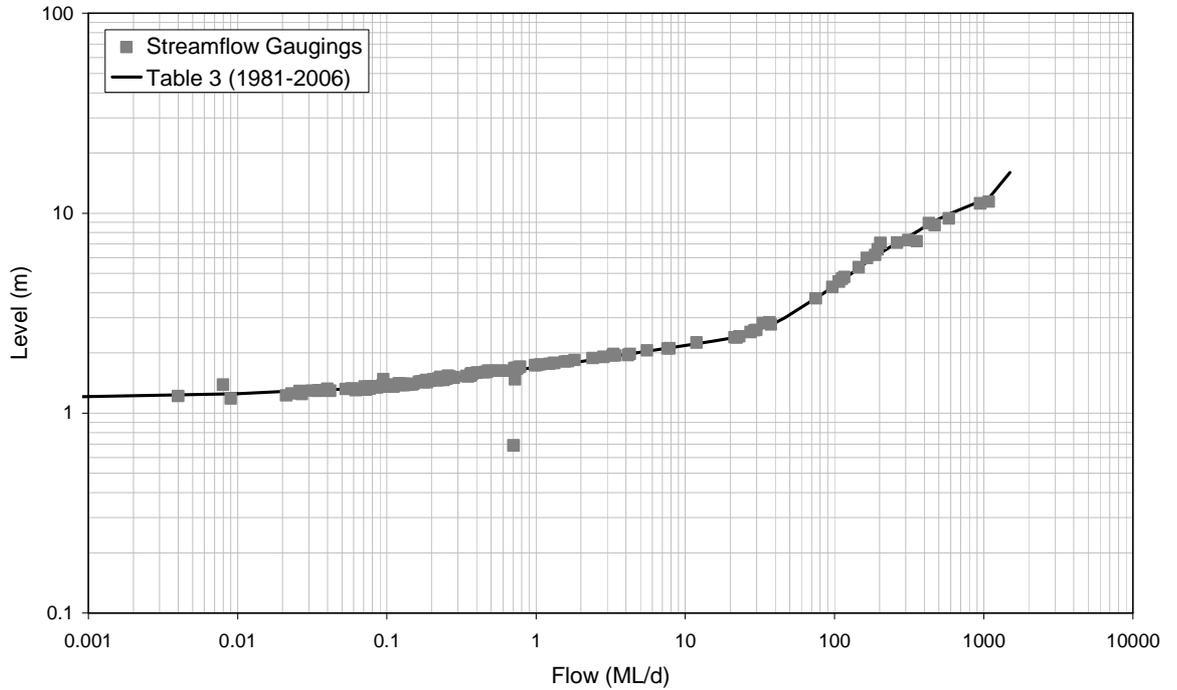
■ **Figure A-48: Rating Table 3 and Streamflow Gaugings for 8170002 (1981-2006)**
