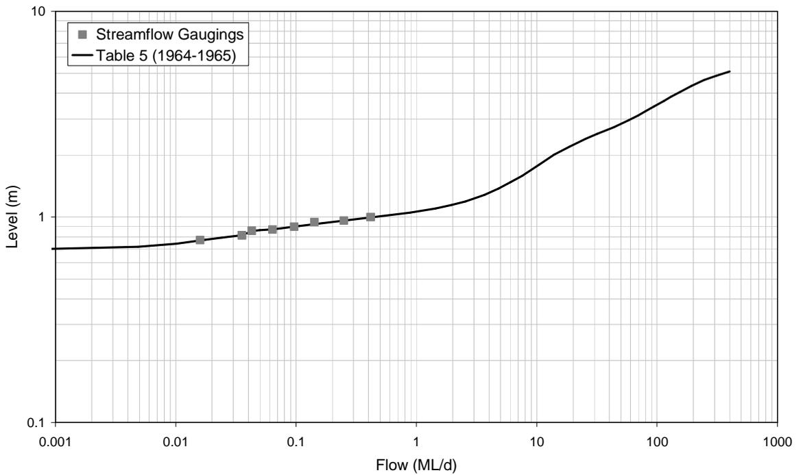
■ **Figure A-68: Rating Table 1 and Streamflow Gaugings for 8170066 (1964-1965)**
