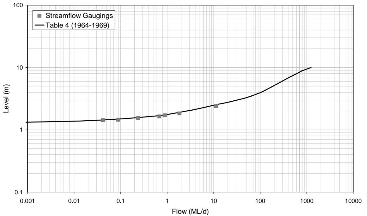
■ **Figure A-21: Rating Table 4 and Streamflow Gaugings for 8150098 (1964-1969)**
