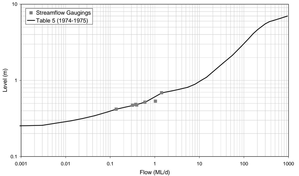
■ **Figure A-89: Rating Table 5 and Streamflow Gaugings for 8170084 (1974-1975)**
