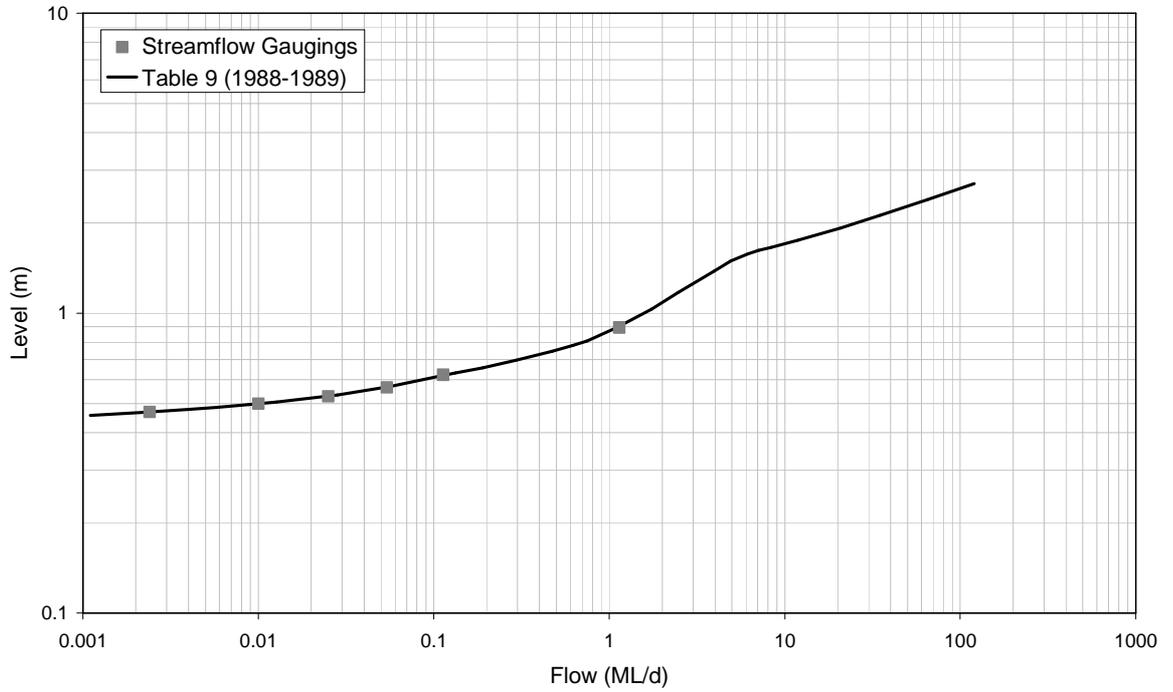
■ **Figure A-105: Rating Table 9 and Streamflow Gaugings for 8170085 (1988-1989)**
