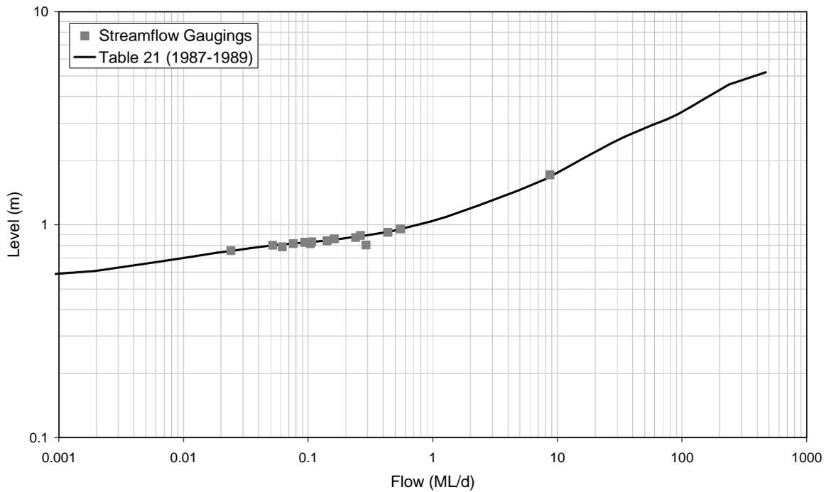
■ **Figure A-82: Rating Table 21 and Streamflow Gaugings for 8170066 (1987-1989)**
