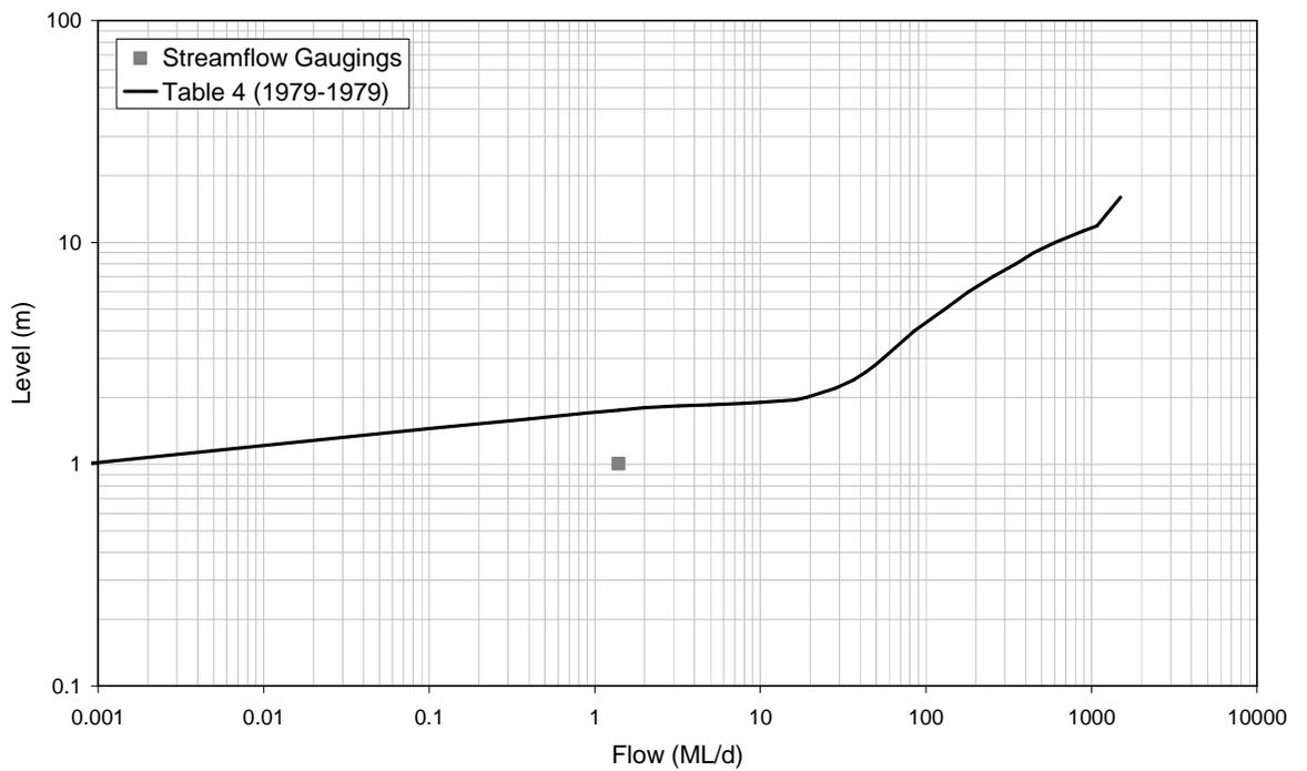
■ **Figure A-43: Rating Table 4 and Streamflow Gaugings for 8170002 (1979)**
