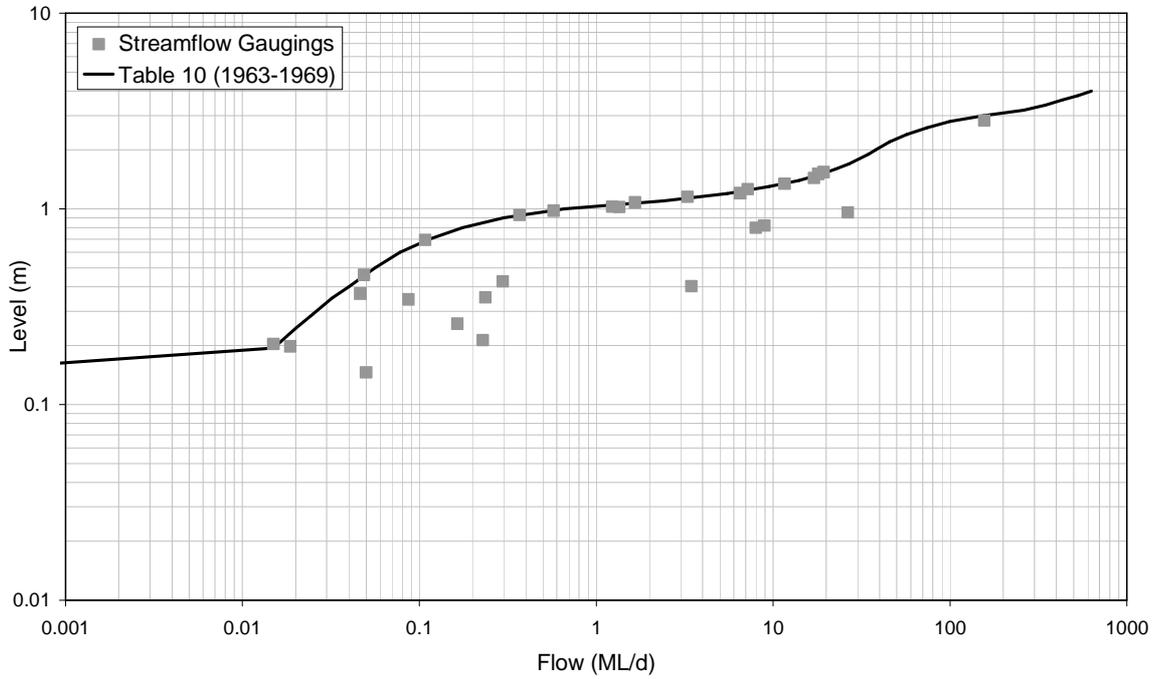
■ **Figure A-2: Rating Table 10 and Streamflow Gaugings for 8150018 (1963-1969)**
