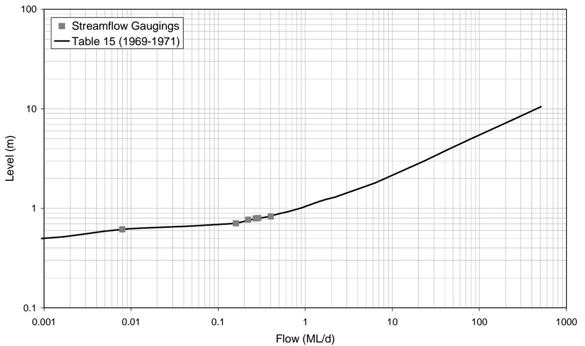
■ **Figure A-54: Rating Table 15 and Streamflow Gaugings for 8170005 (1969-1971)**
