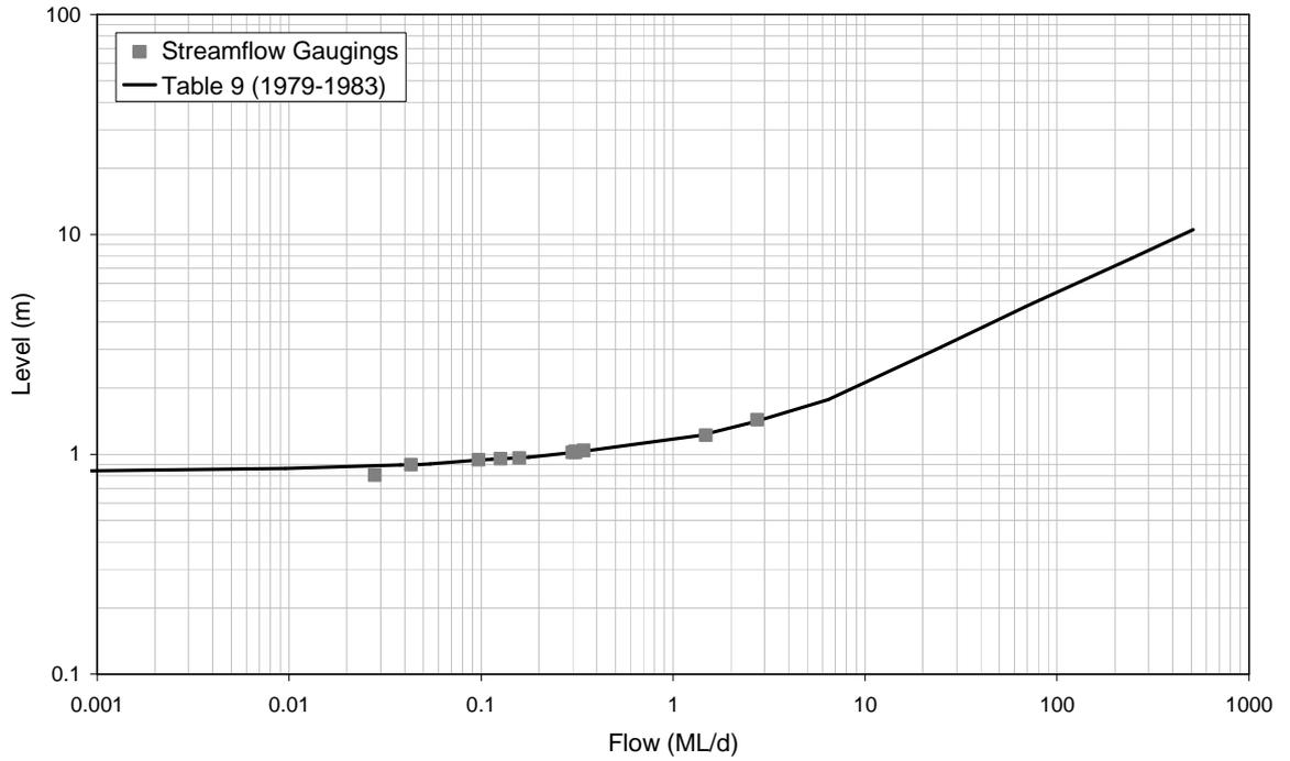
■ **Figure A-59: Rating Table 9 and Streamflow Gaugings for 8170005 (1979-1983)**
