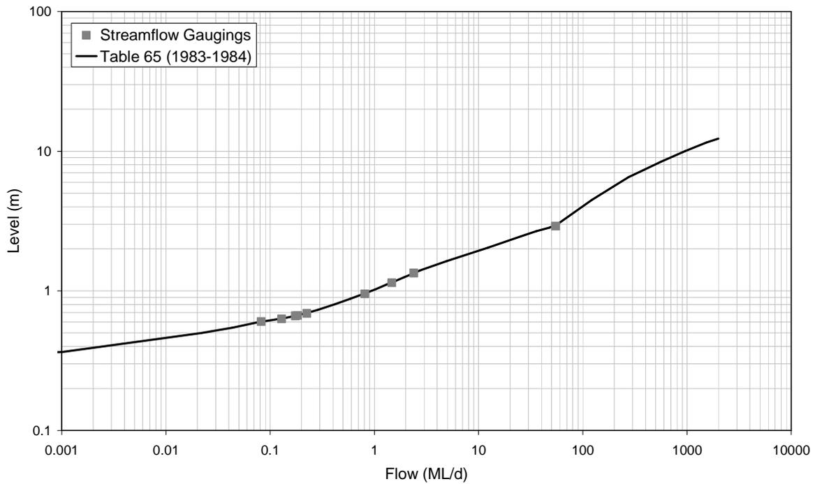
■ **Figure A-38: Rating Table 65 and Streamflow Gaugings for 8150180 (1983-1984)**
