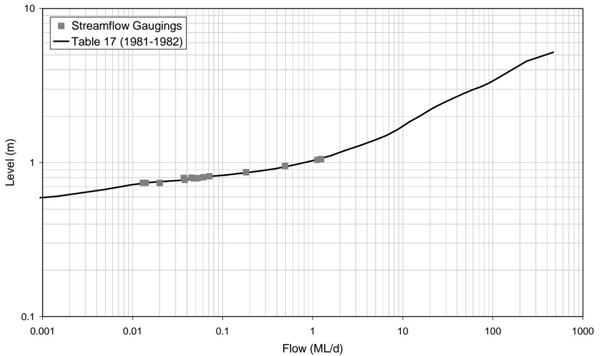
■ **Figure A-78: Rating Table 17 and Streamflow Gaugings for 8170066 (1981-1982)**
