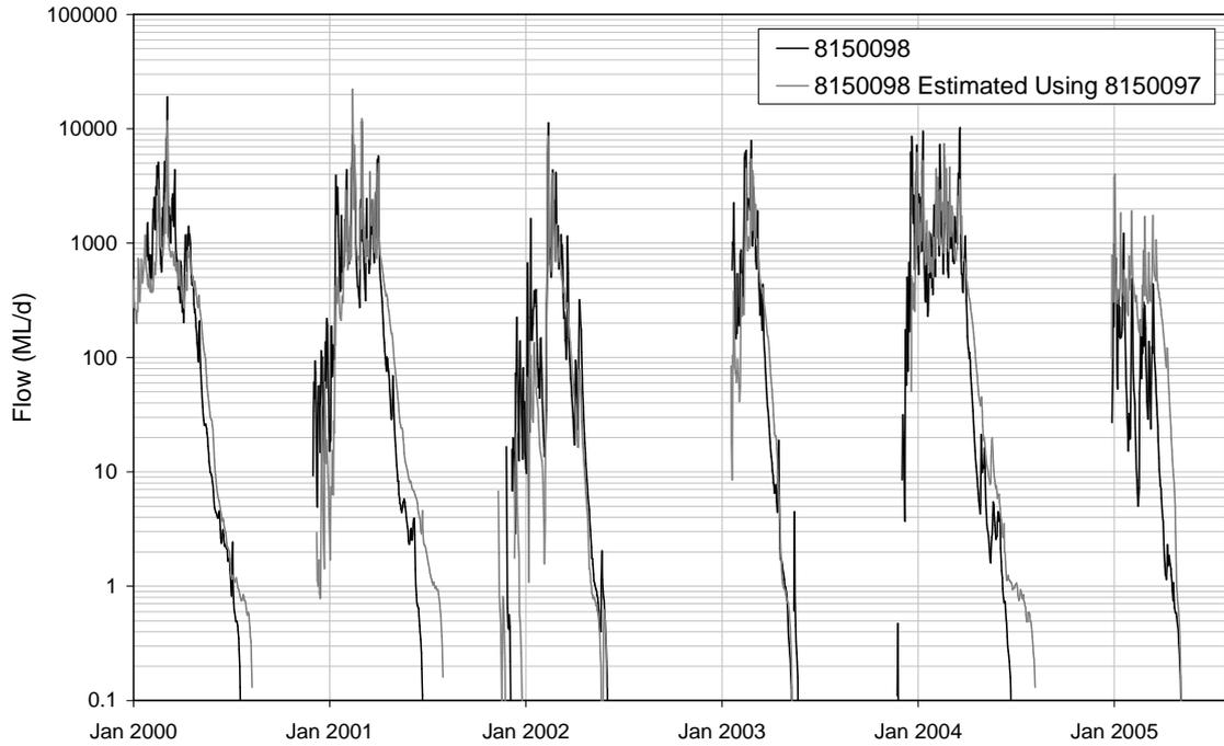
■ **Figure C-5: Comparison of Gauged and Estimated Flow at 8150098**
