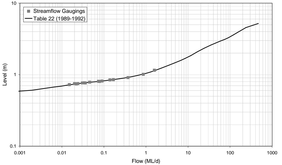
■ **Figure A-83: Rating Table 22 and Streamflow Gaugings for 8170066 (1989-1992)**
