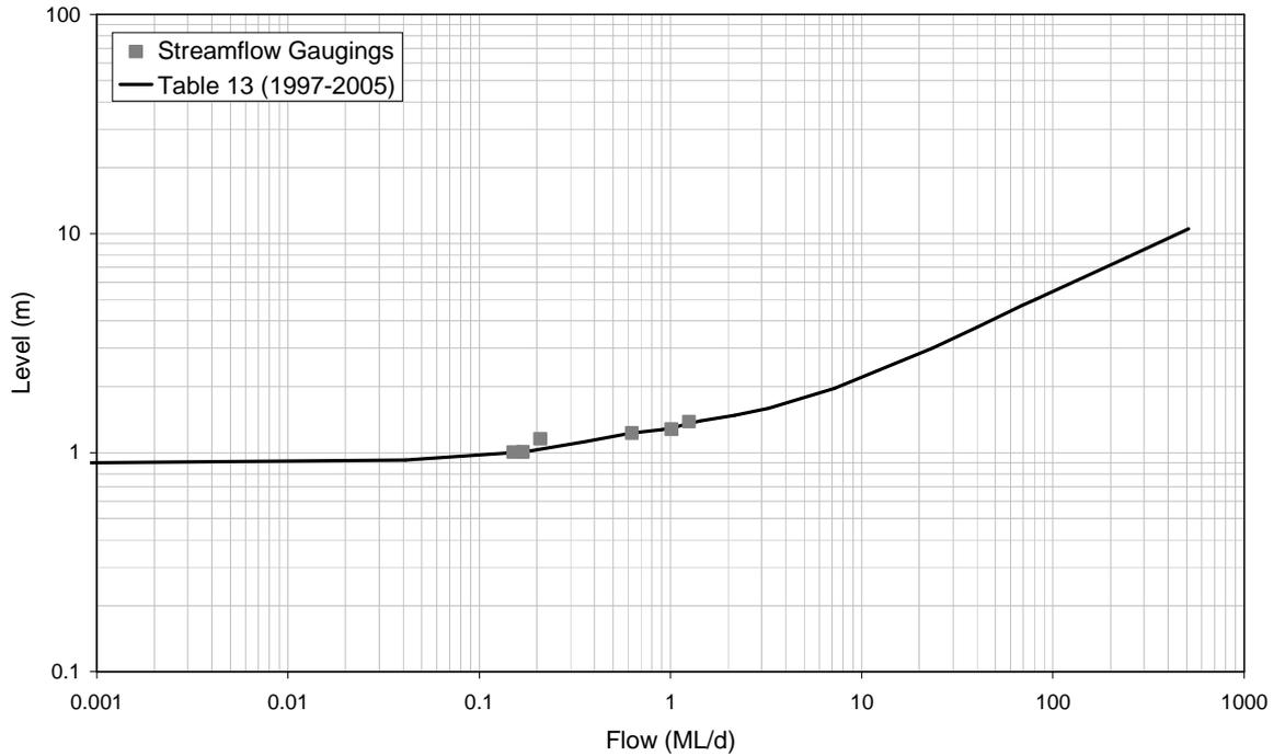
■ **Figure A-63: Rating Table 13 and Streamflow Gaugings for 8170005 (1997-2006)**
