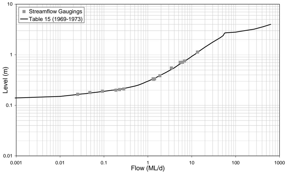
■ **Figure A-3: Rating Table 15 and Streamflow Gaugings for 8150018 (1969-1973)**
