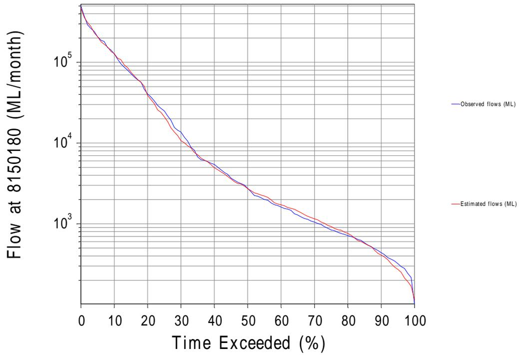
■ **Figure D-11 Monthly SIMHYD Flow-Duration Curve - Finniss River at Gitchams (G8150180)**
