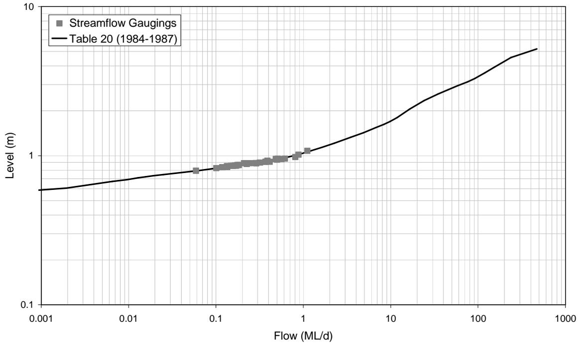
■ **Figure A-81: Rating Table 20 and Streamflow Gaugings for 8170066 (1984-1987)**
