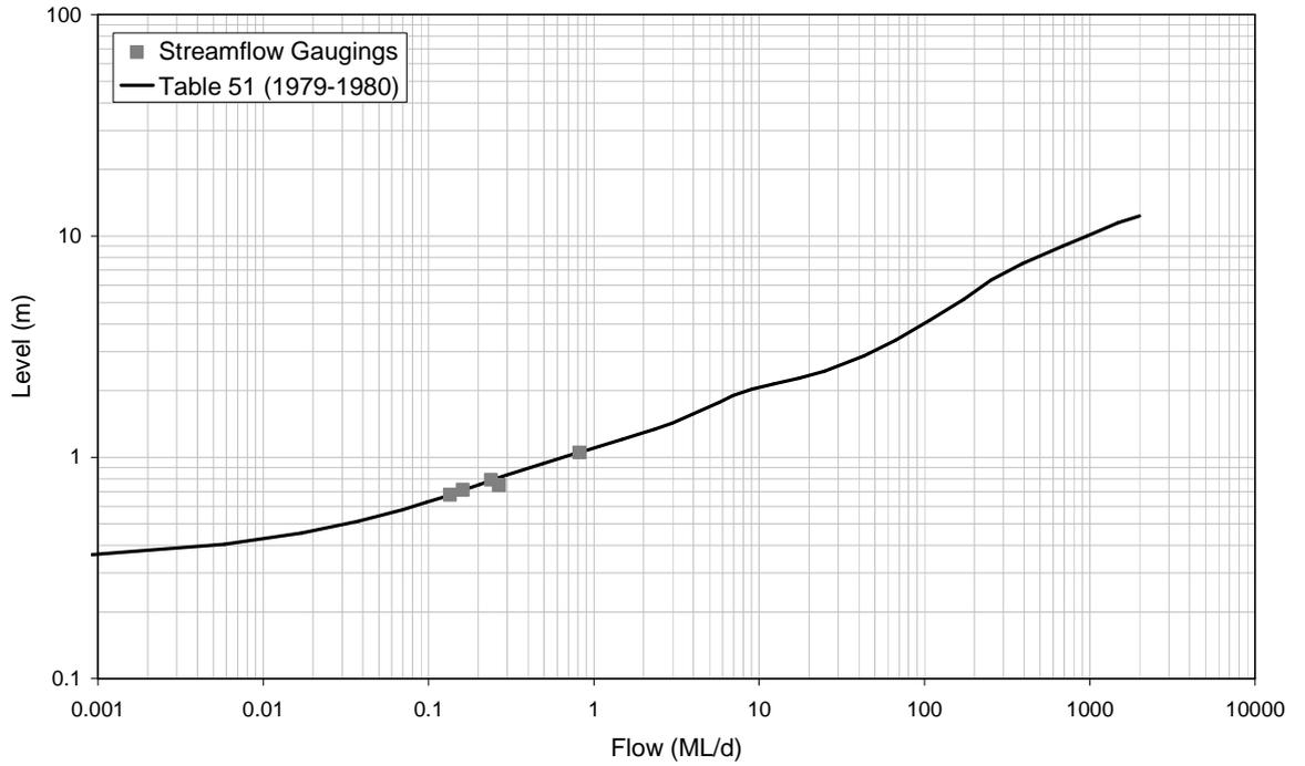
■ **Figure A-35: Rating Table 51 and Streamflow Gaugings for 8150180 (1979-1980)**
