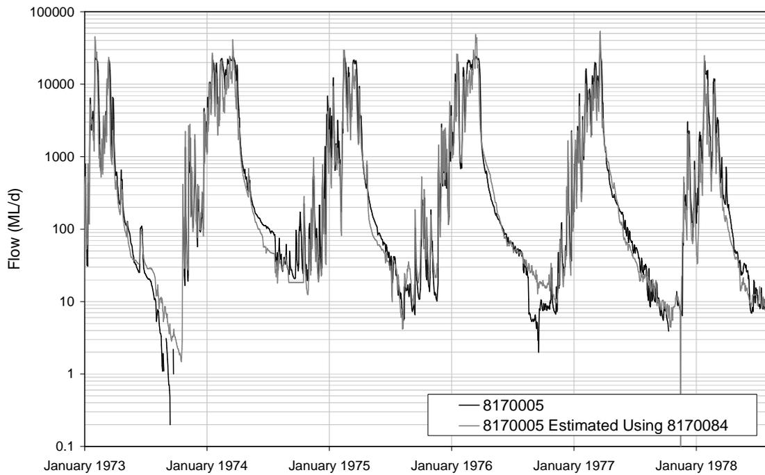
■ **Figure C-8: Comparison of Gauged and Estimated Flow at 8170005**
