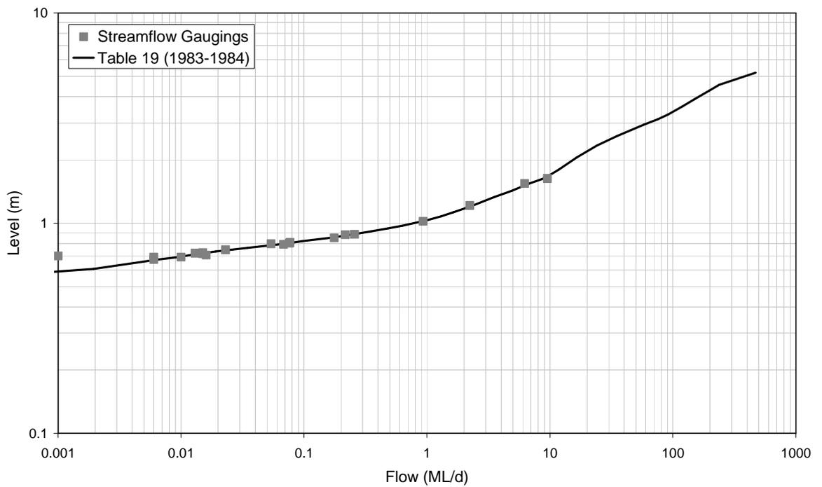
■ **Figure A-80: Rating Table 19 and Streamflow Gaugings for 8170066 (1983-1984)**
