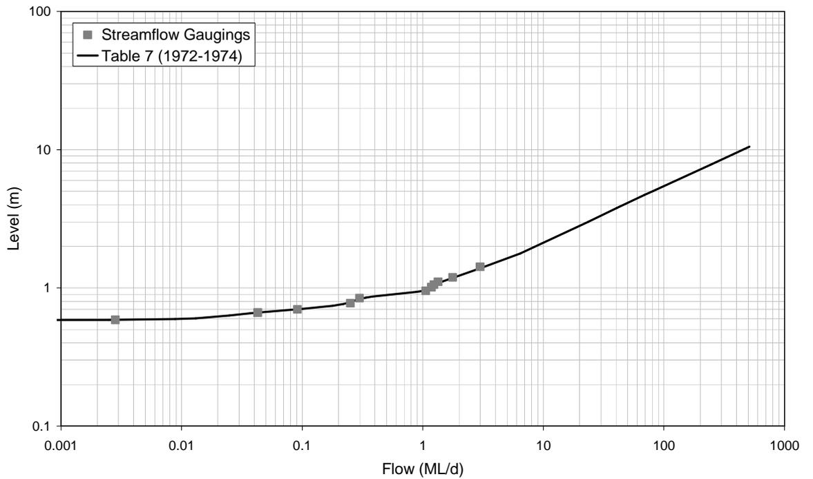
■ **Figure A-56: Rating Table 7 and Streamflow Gaugings for 8170005 (1972-1974)**
