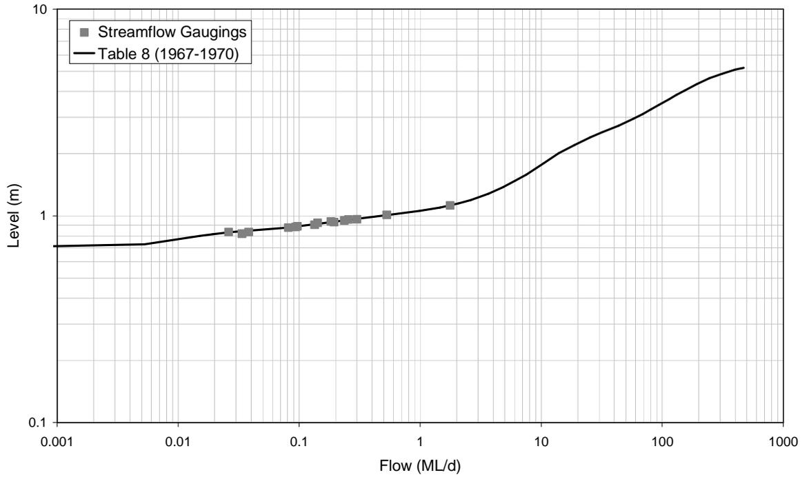
■ **Figure A-71: Rating Table 8 and Streamflow Gaugings for 8170066 (1967-1970)**
