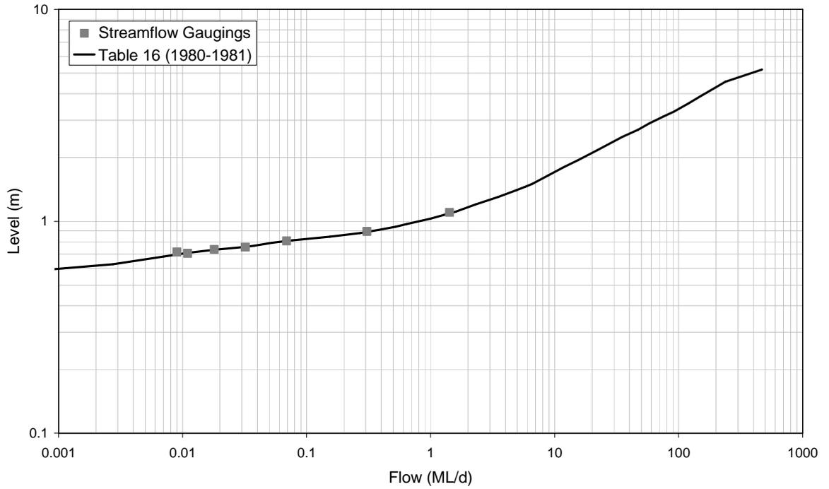
■ **Figure A-77: Rating Table 16 and Streamflow Gaugings for 8170066 (1980-1981)**
