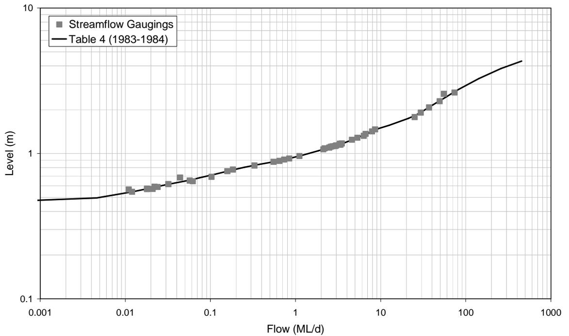
■ **Figure A-16: Rating Table 4 and Streamflow Gaugings for 8150097 (1983-1984)**
