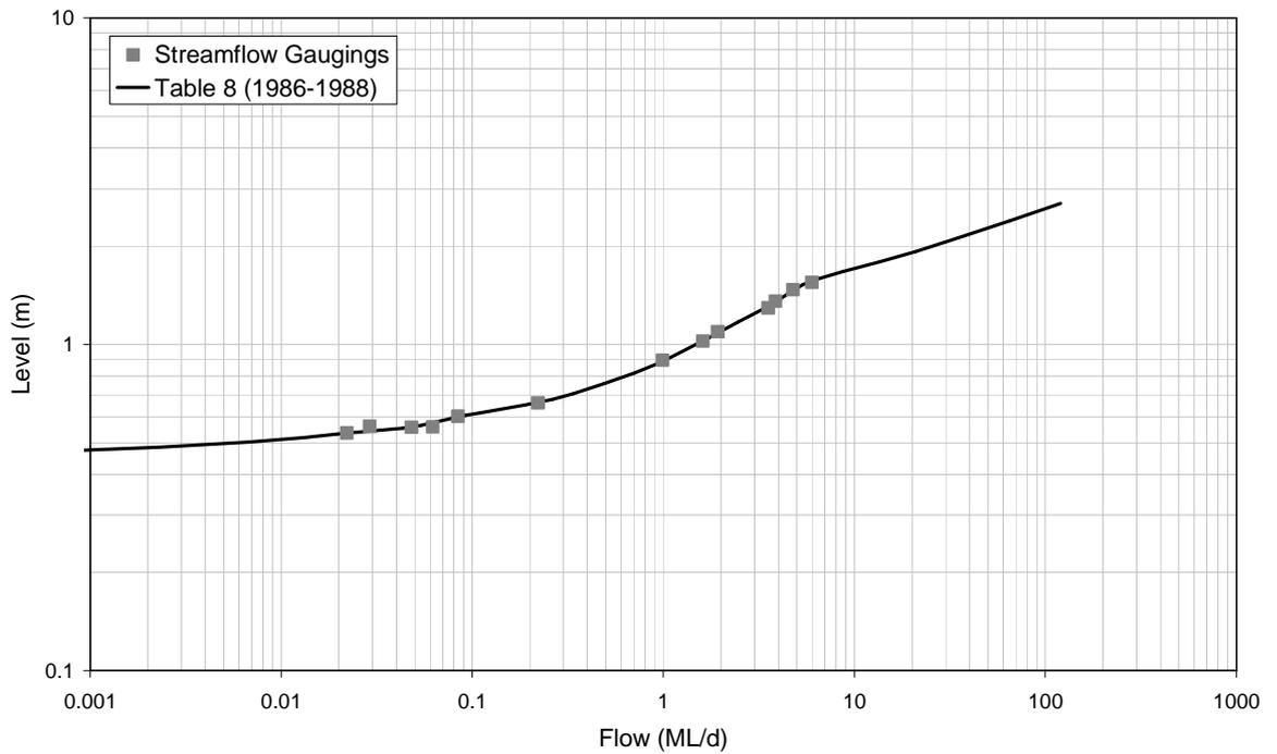
■ **Figure A-104: Rating Table 8 and Streamflow Gaugings for 8170085 (1986-1988)**
