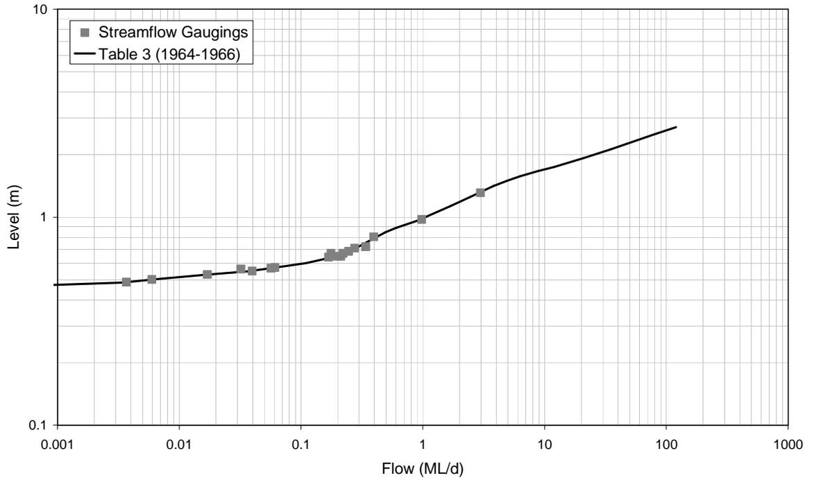
■ **Figure A-99: Rating Table 3 and Streamflow Gaugings for 8170085 (1964-1966)**
