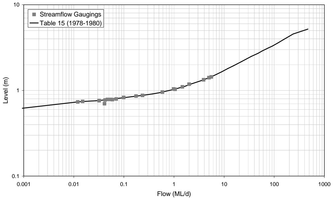
■ **Figure A-76: Rating Table 15 and Streamflow Gaugings for 8170066 (1978-1980)**
