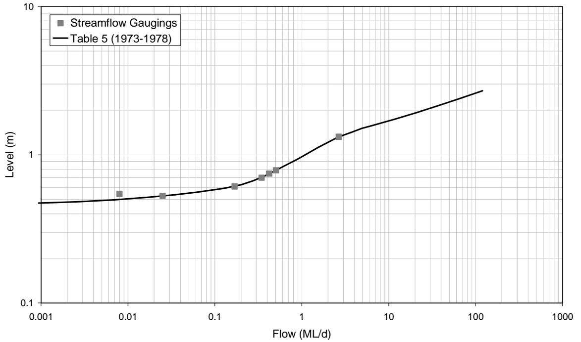
■ **Figure A-101: Rating Table 5 and Streamflow Gaugings for 8170085 (1973-1978)**
