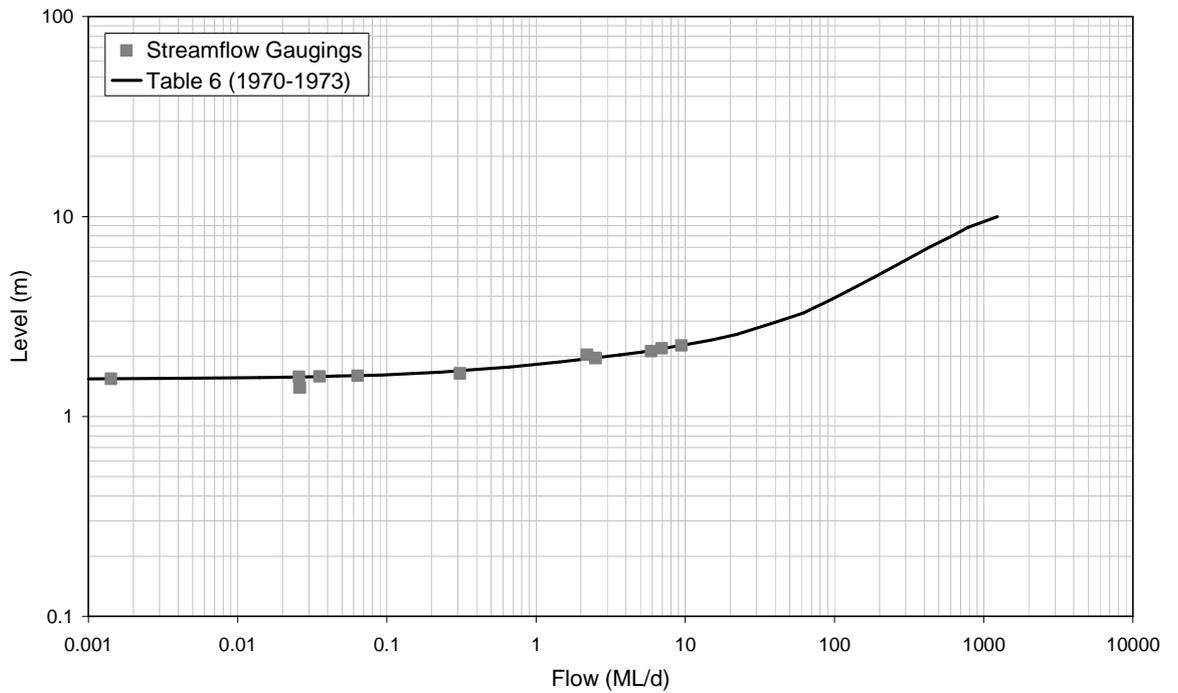
■ **Figure A-23: Rating Table 6 and Streamflow Gaugings for 8150098 (1970-1973)**
