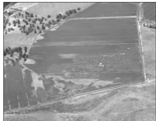
This photo shows uneven irrigation which contributes to poor water use efficiency.
