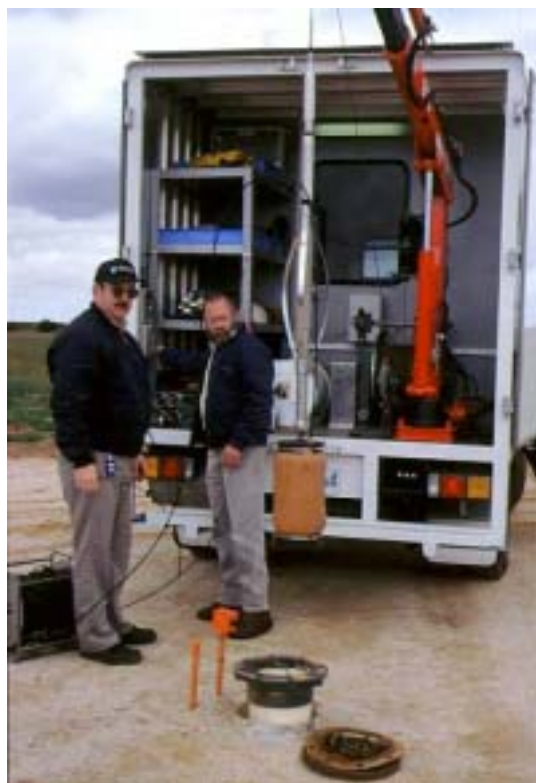
Figure 4.10. Preparing to carry out borehole flowmeter measurements. Photo courtesy of Paul Pavelic, CSIRO.
