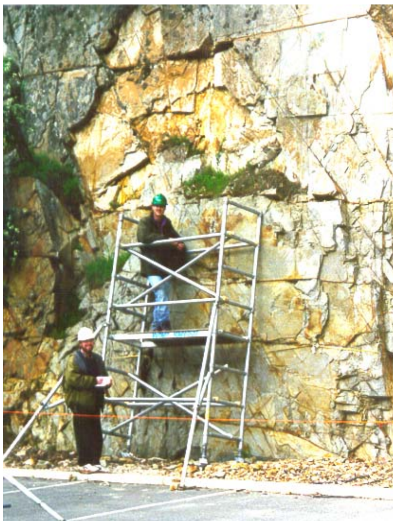
Figure 3.1. Mapping fracture properties in an exposure in the Mintaro Shale, Clare Valley, South Australia. Five sets of fractures are present, four steeply dipping sets and one gently dipping set. This site is located on the limb of a major syncline, with the bedding planes oriented vertically. The bedding comprises one vertically dipping fracture set that strikes 151^{\circ} . (The cliff face is the bedding plane.) A second set of vertical fractures strikes 59^{\circ} . A set of conjugate shear fractures has the same trend as the second set of vertical fractures with dips of approximately 60^{\circ} . The only shallow dipping fracture set has a strike of 345^{\circ} and a dip of 27^{\circ} .
